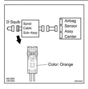
(a) For the orange connector (on the spiral cable sub–assy side) between the horn button assy and the spiral cable sub–assy, measure the voltage between D+ and body ground.
