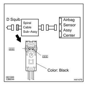
(a) For the black connector (on the spiral cable sub-assy side) between the horn button assy and the spiral cable sub-assy, measure the resistance between D2+ and D2-.
