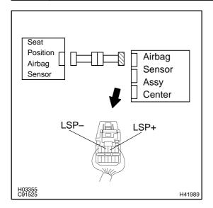
(a) For the connector (on the airbag sensor assy center side) between the airbag sensor assy center and the seat position airbag sensor, measure the resistance between LSP+ and LSP-.
