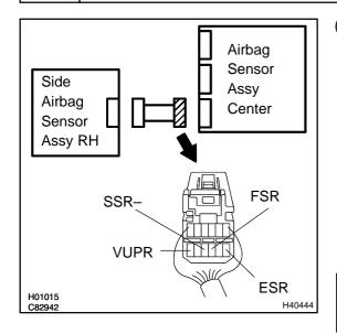
(a) For the connector (on the airbag sensor assy center side) between the airbag sensor assy center and the side airbag sensor assy (RH), measure the resistance between VUPR and ESR, and between FSR and SSR-.
