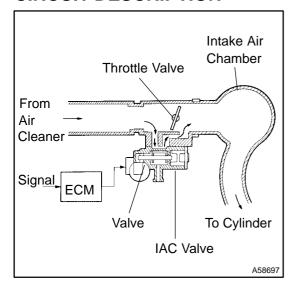
The rotary solenoid type idle air control (IAC) valve is located under the throttle body and intake air bypassing the throttle valve flows into the IAC valve through the passage.
