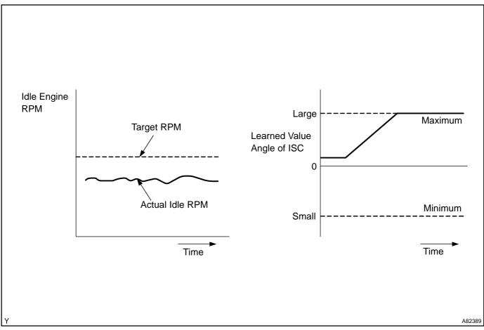
The idle speeds are determined depending on the volume of air that passes through the IAC valve. When the volume is large, the idle speed becomes higher. When the volume is small, the idle speed becomes lower. The IAC valve controls the air volume that bypasses the throttle valve. The engine control module (ECM) sends duty signals to the IAC valve and drives the IAC valve stepper motor to determine the air volume that bypasses the throttle valve.
