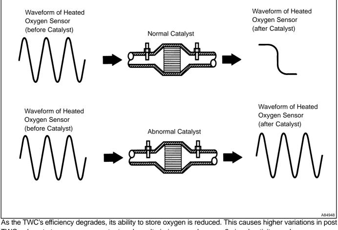
TWC exhaust stream oxygen content and results in increased sensor 2 signal activity as shown. When running the monitor, the ECM compares sensor1 and sensor 2 signals over a specific time to determine the TWC efficiency. The ECM begins by calculating the signal length for both sensors.
