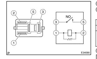
(a) Remove the EFI relay from the engine room R/B.(b) Check for continuity in the EFI relay.
