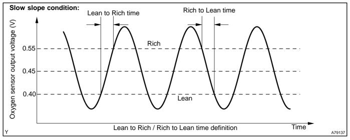
The engine control module (ECM) uses the heated oxygen sensor information to regulate the air–fuel ratio close to a stoichiometric ratio. This maximizes the catalytic converter's ability to purify the exhaust gases. The sensor detects oxygen levels in the exhaust gas and sends this signal to the ECM.
