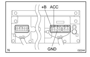
(a) Check that the continuity between terminals at each condition, as shown in the chart.
