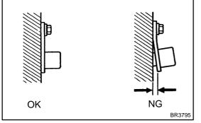
(a) Check the speed sensor installation. **OK**:
