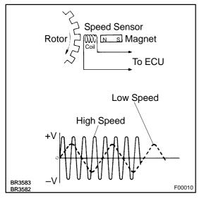
The speed sensor detects wheel speed and transmits the appropriate signals to the ECU. These signals are used for control of the ABS control system. Each of the front and rear rotors has 48 serrations.
