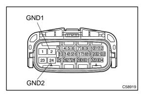
(a) Measure resistance between terminal GND (1,23) of skid control ECU harness side connector and body ground.
