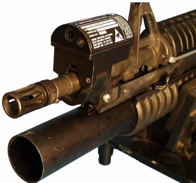
MILES 2000 Transmitter positioned on an M4 Carbine, with M203 attached. (Consult your local TASC for detailed mounting instructions and supporting offset target data)
