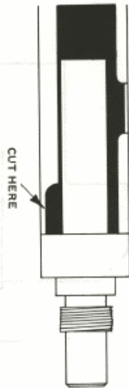
Figure 5 UPPER RECEIVER CLEARANCE CUT
