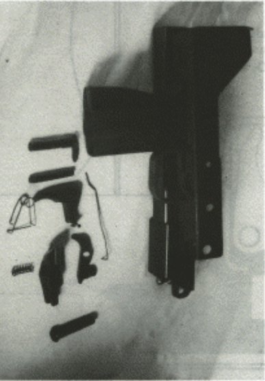
Detail stripped .45 ACP selective fire MAC 10 (less upper receiver. Note selector (far left, bottom row) which is, of course, non-existent in semi-auto model.
