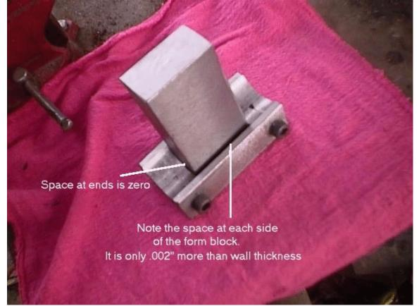
The basic die setup for forming the mag well lips
