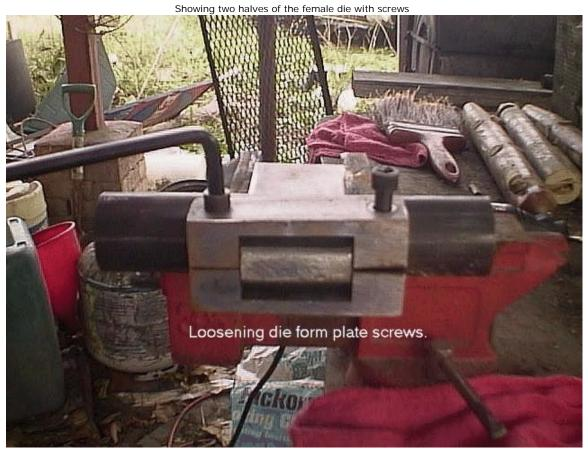
Female die must be formed in two halves in order to release pressure after forming mag well lips
