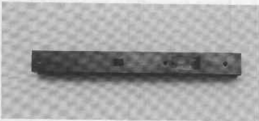
PHOTO 9: Bottom side view of upper receiver tube showing three bolt holes, magazine well, and sear recess.
