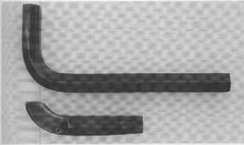
PHOTO 40: The sear before and after modification. Note the position of the spring pin.
