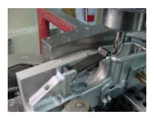
Always check your parts with the feature that is to receive them. I don't have to tell you it is a lot easier now to widen a tight slot than to find out later after you have anodized you work and the trigger guard won't fit!
