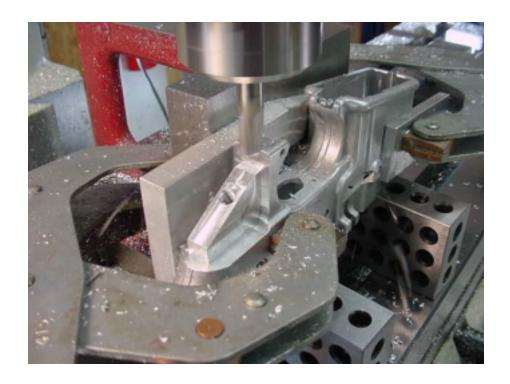
The trigger guard slots are 7/16" wide, but I like to use a 3/8" cutter. While on the centerline, cut down until you are flush with the flat surface of the pistol grip mount and stop there. Now take passes evenly on each side until you have the 7/16" wide slot.
