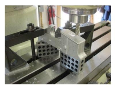
Put the lower on a couple of 1-2-3 blocks and clamp as show above. Using a 1/2" cutter make a flat in the middle of the magazine well, centered and about 3/4" long. Cut this flat in the material that will be removed when we cut the magazine well.
