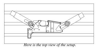
Now the forging is parallel and aligned to the table in the x axis. We will now cut the five surfaces. But, first we have to locate the piece in order for our machining to line up with the various features on the forging.
