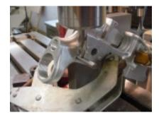
Location: Find the center line as usual and then put a .250 pin in the take down hole. Edge find the pin then move to its center and set zero. Chuck a 1/2" endmill and set the spindle stop and bring the spindle down and lock it against the stop. Raise the table until the cutter touches the pin and zero the elevation dial.
