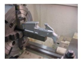
If you don't want to spring for the  $1-3/16 \times 16$  tap for the buffer tube you can use the alternate method of cutting the thread by single pointing it in a lathe.
