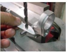
Put a 0.250 dowel pin in the take down hole and move the spindle over it with your drill in place. Bring the quill down to the stop and then bring the table up until the drill touches the pin. A paper shim is always handy and makes a good feeler. Set your elevation dial to zero and then come up 0.639".
