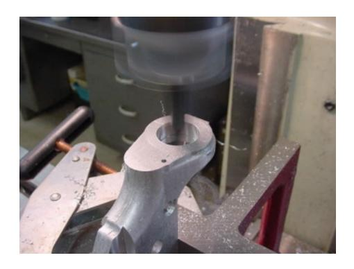
Now for the buffer tube hole. Locate your spindle at 0.000-0.625 and bore a 1.125" hole through the tang.
