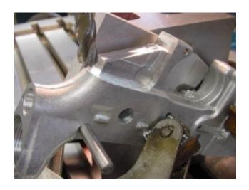
From the pin center-line to the surface to be milled is 1.228". Since we touched off on the top of the pin we will subtract the raidus, .125" from the 1.400" giving us 1.103". Lower the table by this amount and mill the angle face of the pistol grip mount.
