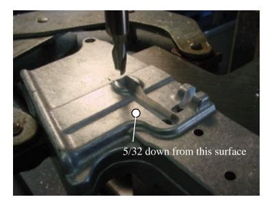
The magazine release lays in a slot you will mill using the same 1/4 inch cutter. The depth of this cut is 5/32 from the surface. The coordinates are 1.938-0.563 to 3.197-0.563.
