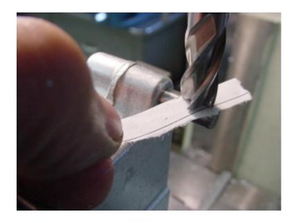
For the slot where the upper and lower meet, chuck a 3/8" end mill. Put a pin in the take-down hole and touch off on the top of the pin. From here you will go down 0.385" to the finished surface.
