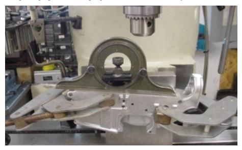
**Workholding:** Set your protractor for 6 degrees and clamp the forging against the angle plate using the clamping pad. Tap the forging until the buble is level and add a second clamp. Re-check the angle after tightening the second clamp.
