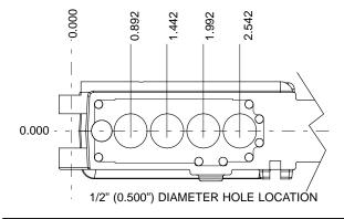
The forging will look like this after the 1/2" holes are drilled.
