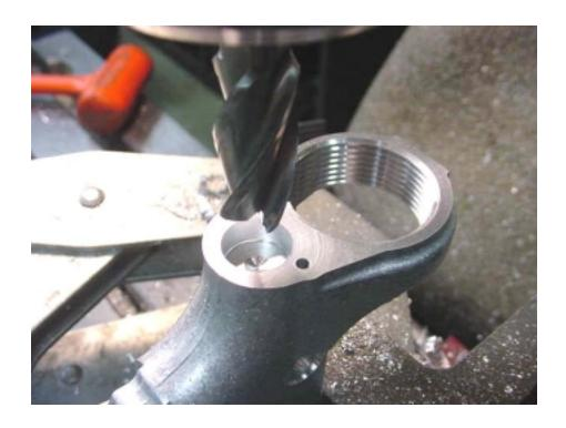
At 0.000-0.375 spot and bore the buttstock anti-rotation hole. The size of this hole is 0.499 plus .004 minus nothing. If you drill a pilot hole first, your 1/2" drill should not cut oversize. It is important not to drill this hole too deep since the buffer retainer hole will go just on the other side. I like to drill a 1/4" hole 1/4" deep and then go in with a 0.500" diameter end mill about .225".
