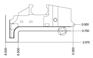
Above is the tool path for a 1" dia cutter. On the right is the table of the 18 steps around the 3/4" radius. The first and last coordinates are the ends of the straight tool paths.
