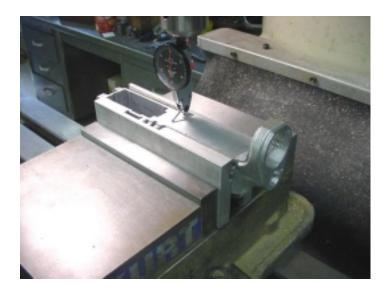
**Workholding:** Clamp up the forging and indicate it as in chapter nine. Position one clamp just behind and below the safety hole and the other clamp with a plate to protect the work just on otp of the magazine release hole. Shown above is an alternate method using a machine vise. Clamp lightly and indicate the deck true then tighten the vise.
