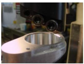
You can put a tool in your boring head or flycutter to put a nice 45 degree chamfer on the corner.
