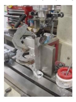
**Workholding:** Clamp the forging to the angle plate using the passenger side plate. Put the butt face against the table. Indicate the deck true to the quill.
