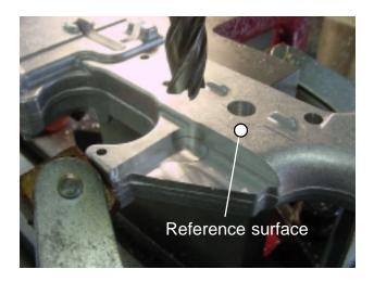
Chuck a 1/2" dia. cutter and touch off on the reference surface. My forging is 0.864 thick at this point so it will be 0.432 to the centerline. The face of the grip pad is 3/16 up from the centerline so we need to subtract .1875 from .432 which gives .244 inches down from the reference surface to the bottom of the cut. You will need to make your own calculations based on the thickness of your particular forging.
