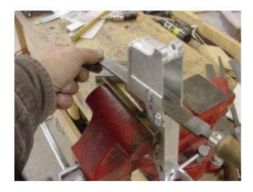
The reason we have left the trigger/hammer cavity solid until now is because we need to grab there with the vise, quite securely, while we file out corners of the magazine well.
