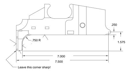
Above are the five surfaces to finish in the first set-up or hold. I use a 1" endmill because it makes for easy math. For the 3/4" radius I x-y it with the 1" endmill in 18 steps (5 degrees each) and it comes out very smooth.
