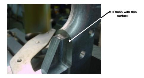
The first surface to mill is 1.050" down from the butt face. Mill until you are flush with the side faces of the pistol grip mount.
