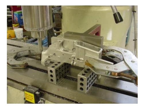
**Location:** Edge find the butt face and then add a second clamp once you have your spindle located. Move 7.500" and set your X axis zero over the pivot pin hole. Y axis zero should be the same as the last setup.
