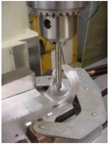
Since you will be drilling into the buffer tube threads, the investment in a long #3 center drill is well worth it. Move to the location and spot the hole to the full diameter (.250) of the center drill.
