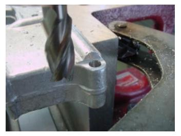
Now use a 3/8" cutter and move to  $0.043 \, x$  (to the right of the pivot pin hole and mill off the face at a setting of  $0.522 \, \text{from}$  the centerline. Check that the pivot pin fits nicely before moving on.
