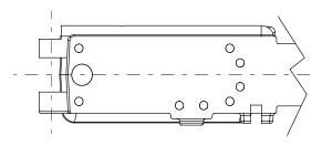
The forging will look like this after the 5/16" hole is drilled.
