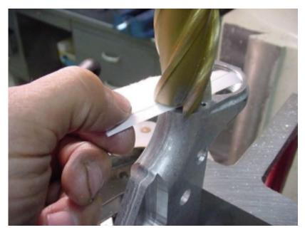
Chuck up a cutter and touch off on the butt face. I use printer paper that is 0.004" thick and set my dial that amount before the zero.
