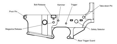
That concludes the drilling portion for this setup. Check your work against the drawing above and be sure you have all eight holes.
