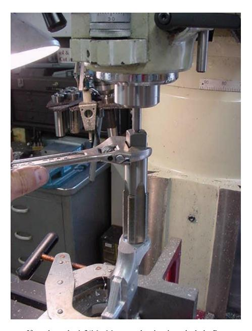
If you have the 1-3/16 - 16 tap go ahead and tap the hole. Put a center in the spindle to keep the tap aligned and with a light pressure on the down handle turn the tap with a wrench. If you don't have a tap, you can single-point the thread in a lathe, see the appendix.
