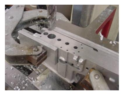
Spot and drill the four roughing holes through with a 5/16" or 3/8" drill. Next, drill through 1/2" diameter at the same locations.
