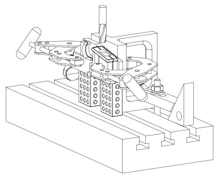
Here is an alternate method for cutting the clamp flat. Support the lower on a 1-2-3 blocks and using the passenger side clamp pad, clamp it to an angle plate. You can also hold the lower in a vise using the driver side and passenger side pads.
