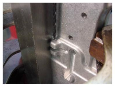
Locate the spindle at 0.625-.188 and chuck that long 3/32 drill. Here is where you will use that little block I told you to make in chapter one. Hold the block tightly against the angle plate and the forging. The drill should line up exactly with the hole in the block. Holding the block tightly, drill the hole through the lug on the forging. Drilling this hole any other way will drive you nuts!
