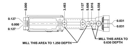
The cavity will be milled out using a 7/16" (0.4375") end mill. This will leave the proper radii in the corners. Refer to the diagram above for the travel limits. It is best to rough it out first leaving about 0.005" per side and on the bottom for finishing. Plunging works well for roughing. Blow the chips out often to avoid binding the cutter.
