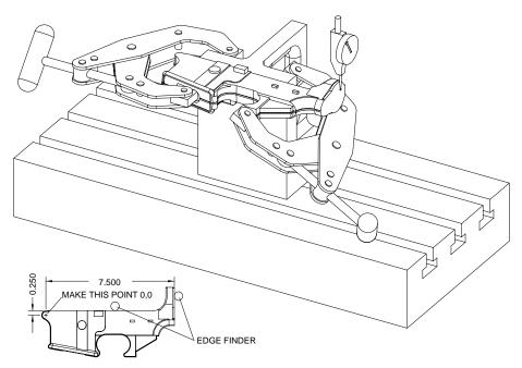
Location: Pick up the surface just indicated (butt face) with an edge finder and then the face of the forging that is against the angle plate (deck). Move to the location of the pivot pin (7.500X -.250Y) and zero your DRO. Refer to the drawing "DRIVER SIDE" in the appendix for dimensions for this setup.
