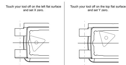
While stroking the quill up and down, move the tool towards the corner with the table locked at Y zero. Once you see the tool is taking a chip you only want to advance the table when the tool is up and out, and then advance no more than 0.005" per stroke. Keep going until you reach X 0.017.
