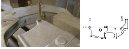
Drill and ream .251 dia. the pivot pin hole through at 0.000-0.000. Now do the same for the take-down pin hole at 6.375-0.000.
