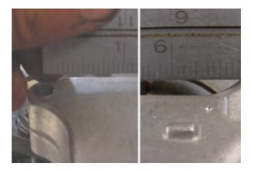
When doing this kind of work it is a wise move to just touch the work with the center drill and then lay your scale on it just to make sure you are in the right place.
