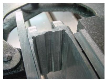
When you have removed all you can with the 3/8 mill there will only be some small cusps in the corners that remain to be eliminated. You can do this with a file or if you make a tool you can 'stroke' it out using your milling machine spindle as a verticle shaper.
