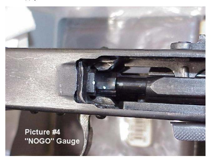
**Option 1:** Obtain a "Field" headspace gauge to accomplish the same check as stated above to ensure that the reference marks will not align. This gauge indicates the maximum "SAFE" chamber dimension.
