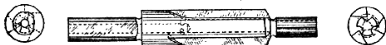
Three groove drill of high speed steel, with straight grooves, to bore out old barrels for relining.
