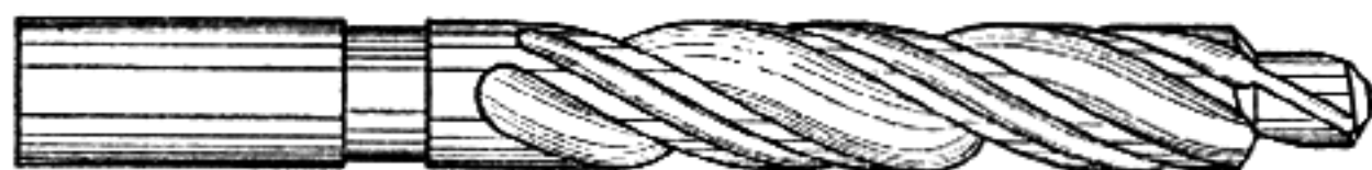
Standard commercial three groove twist drill, with pilot ground on it, to drill out old barrels for relining.
