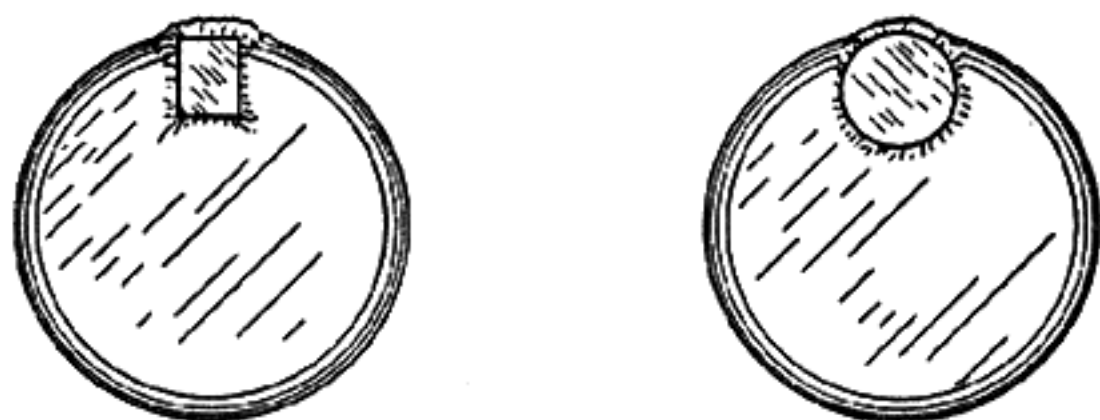
Left is impression made by the rectangular shape, flat-pointed rim-fire firing-pin on a .22 rim-fire case. Right illustrates impression made upon same case by the round, flat-pointed, rim-fire firing-pin.
