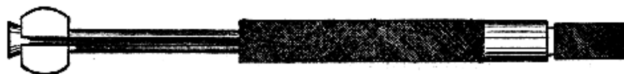
The Starrett small-hole gauge, adjustable for size.
