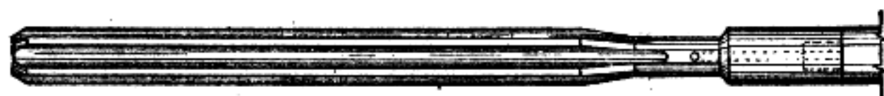
Six-groove barrel reamer, of the type commonly used in sets of three, in graduated sizes.
