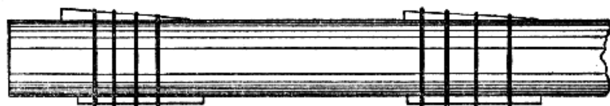
Showing how small wedges are wired around a double-barrel shotgun, used to hold the rib in place while it is being soldered.
