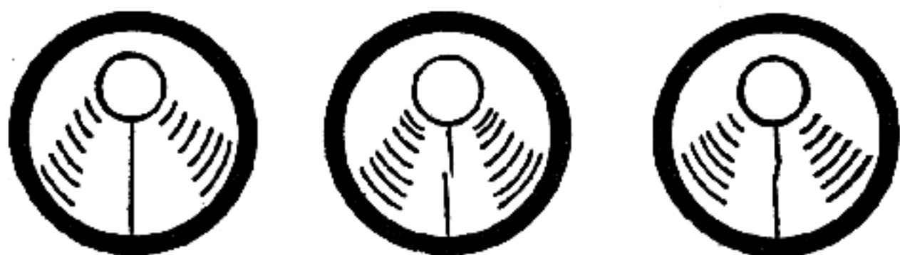
Principle of detecting crooked barrels. Left view shows shadow cast by a straight barrel—other two show shadows cast by crooked barrels.
