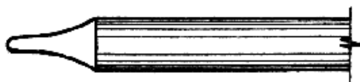
Correct profile of center-fire firing-pin nose.
