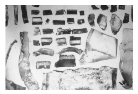
**Figure 10.14** Typical evidence recovered from a pipe bomb that was exploded with a low-explosive filler. (Courtesy of the author's collection.)
