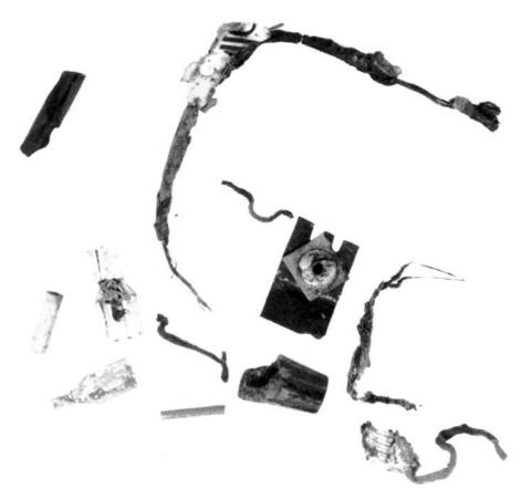
**Figure 10.11** Bomb fragments. Typical fragments from an improvised explosive device that produced a low-order blast, in this case injuring one of the authors.
