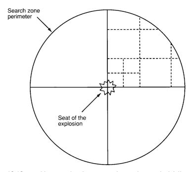
**Figure 10.10** Post-blast search. The area needing to be searched following an explosion should be defined first by a perimeter, then divided into small segments which can be labeled in order to record each location where fragments are found.
