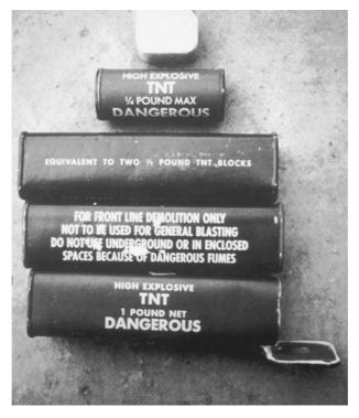
**Figure 8.4** Trinitrotoluene. TNT manufactured for the military comes in a variety of sizes and shapes.
