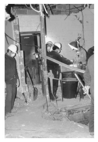
**Figure 10.12** Typical sifting operations at the scene of post-blast scene. Debris is being worked through a fine sifting screen into receptacle below. (Courtesy of F. Guerra.)
