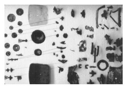
**Figure 10.16** Fragments from a wind-up alarm clock used as a time delay in an improvised explosive device. (Courtesy of the author's collection.)
