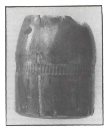
The rifling mark pattern is often easy to see with the naked eye if the bullet isn't too deformed. MagniScation will show up the small details that can link a bullet to a particular weapon.
