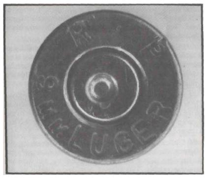
The base of this fired 9mm case has minute marks that can link it to the weapon which fired it The firing pin strike is distinctive, and a slight notch on the case rim may have come from the weapons breechface.
