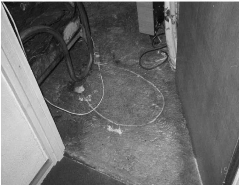
Figure 3.14 Electrical blanket bed fire. Blanket mains lead moved to reveal smoke shadow showing that lead was unplugged during later stages of fire (Photo: Twibell)
