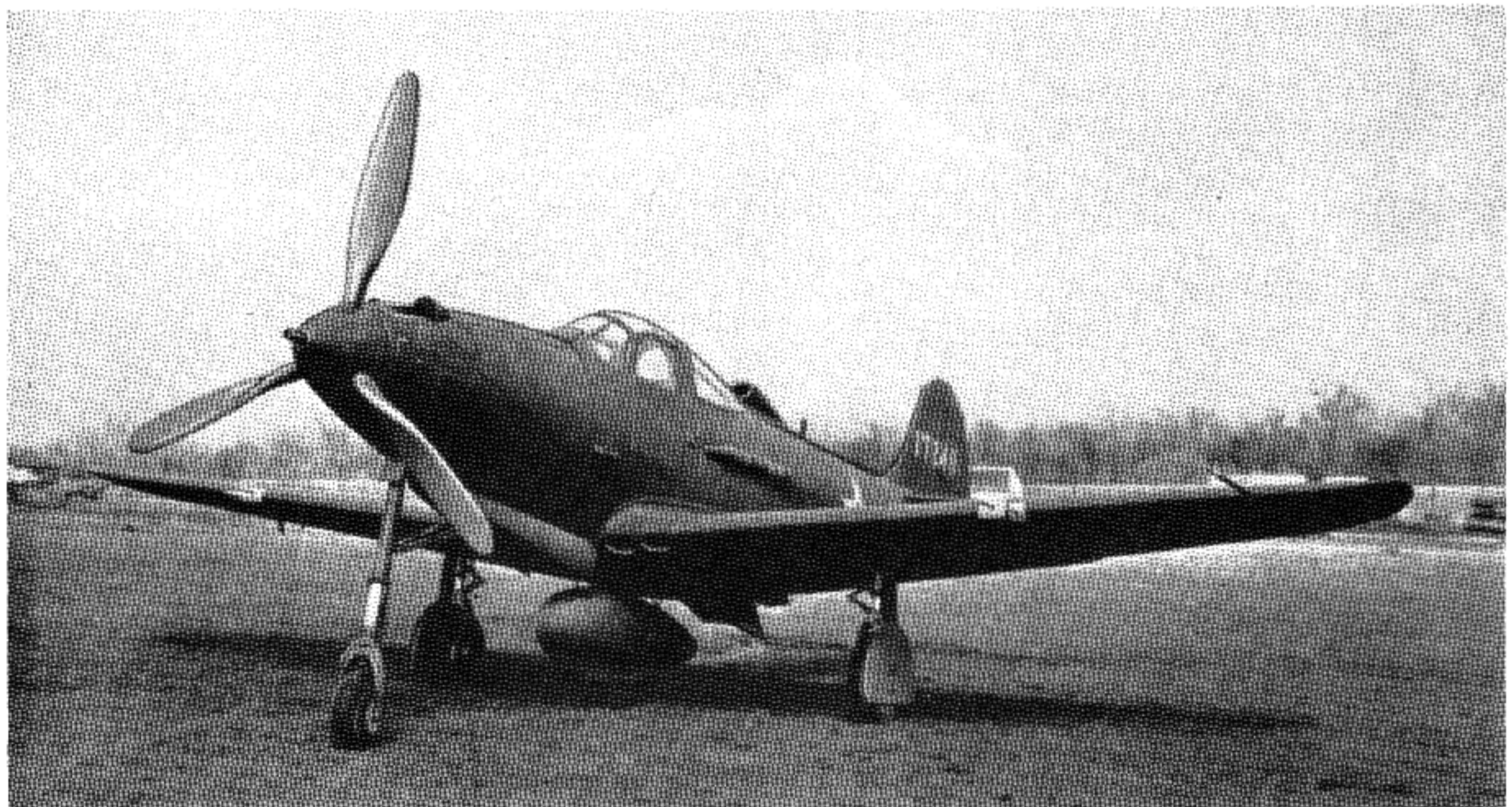
Figure 12-1. 37-mm Browning Gun M4 mounted in a P39F aircraft to fire through the propeller hub.
