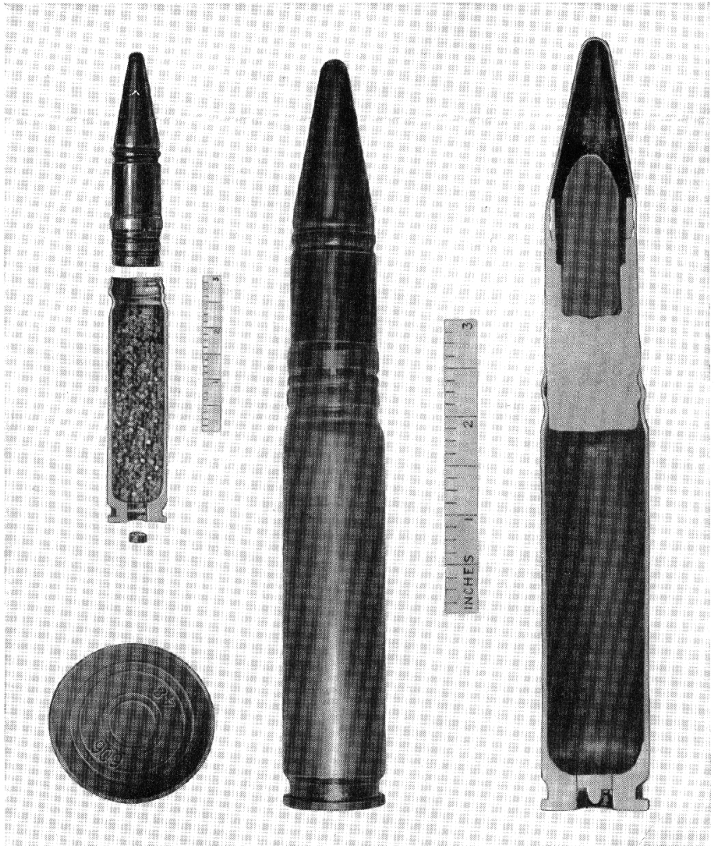
Figure 9-15. Study of a complete round for 23-mm NS cannon.
