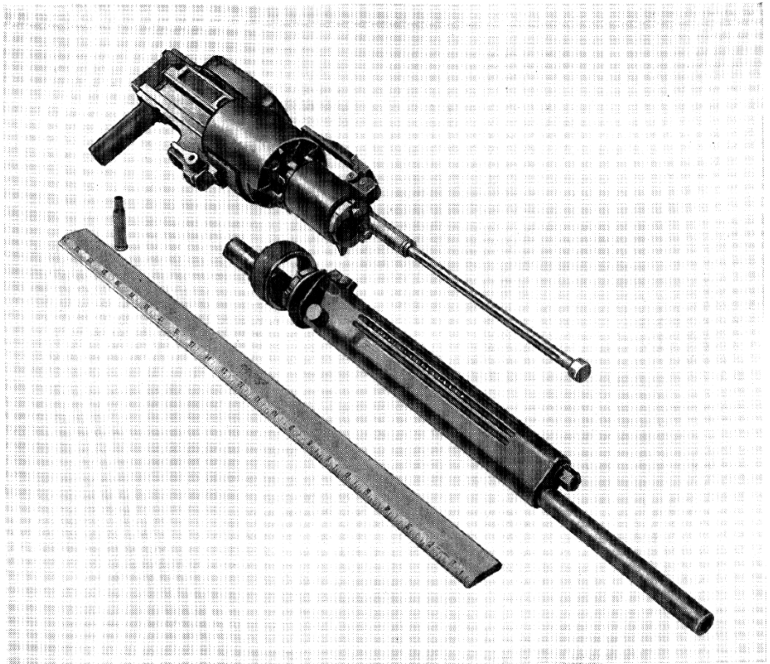
Figure 4-6. 7.62-mm Shkas Fixed Gun, with barrel assembly removed.
