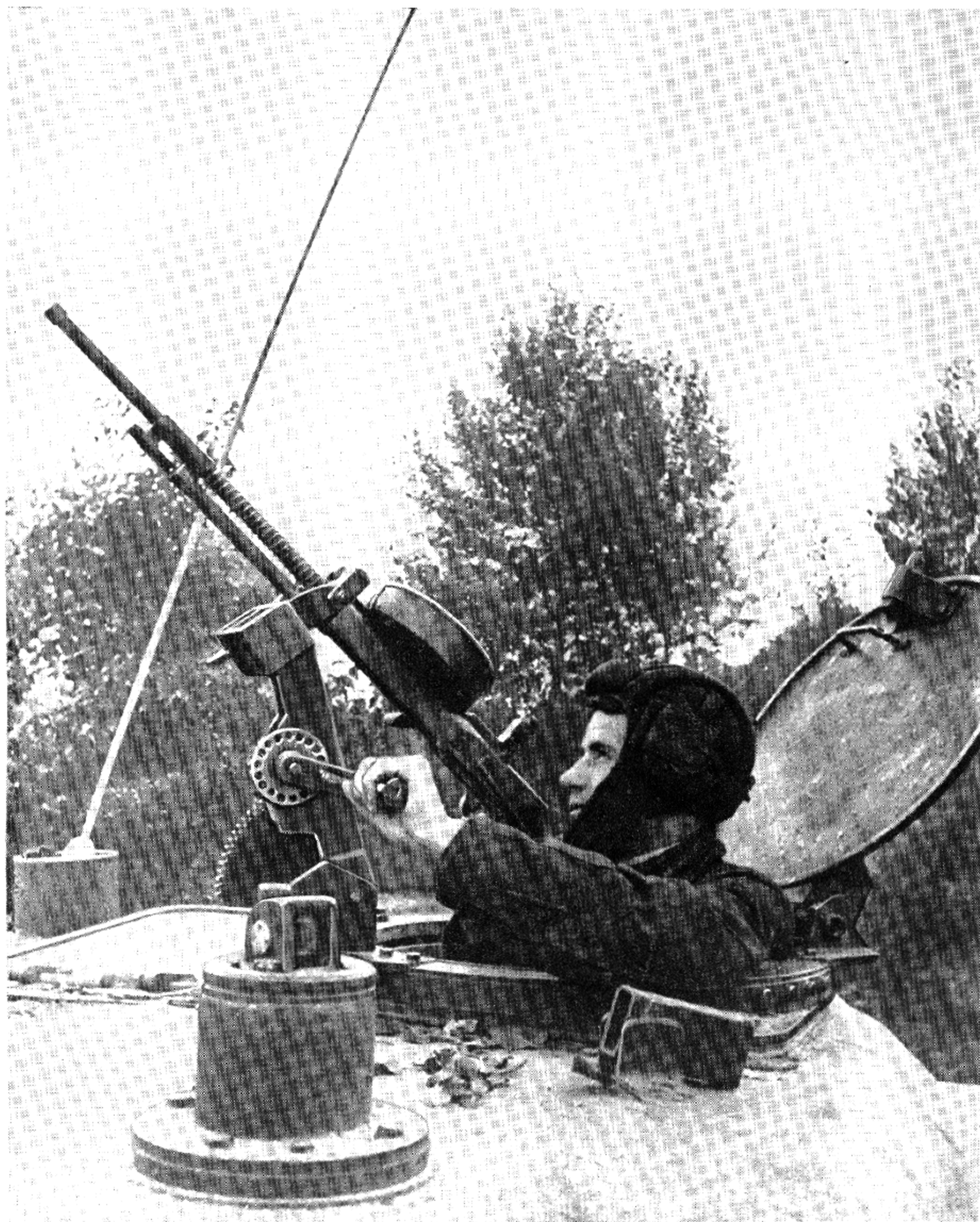
Figure 3-2. Degtyarev Tank Machine Gun in anti-aircraft firing position.
