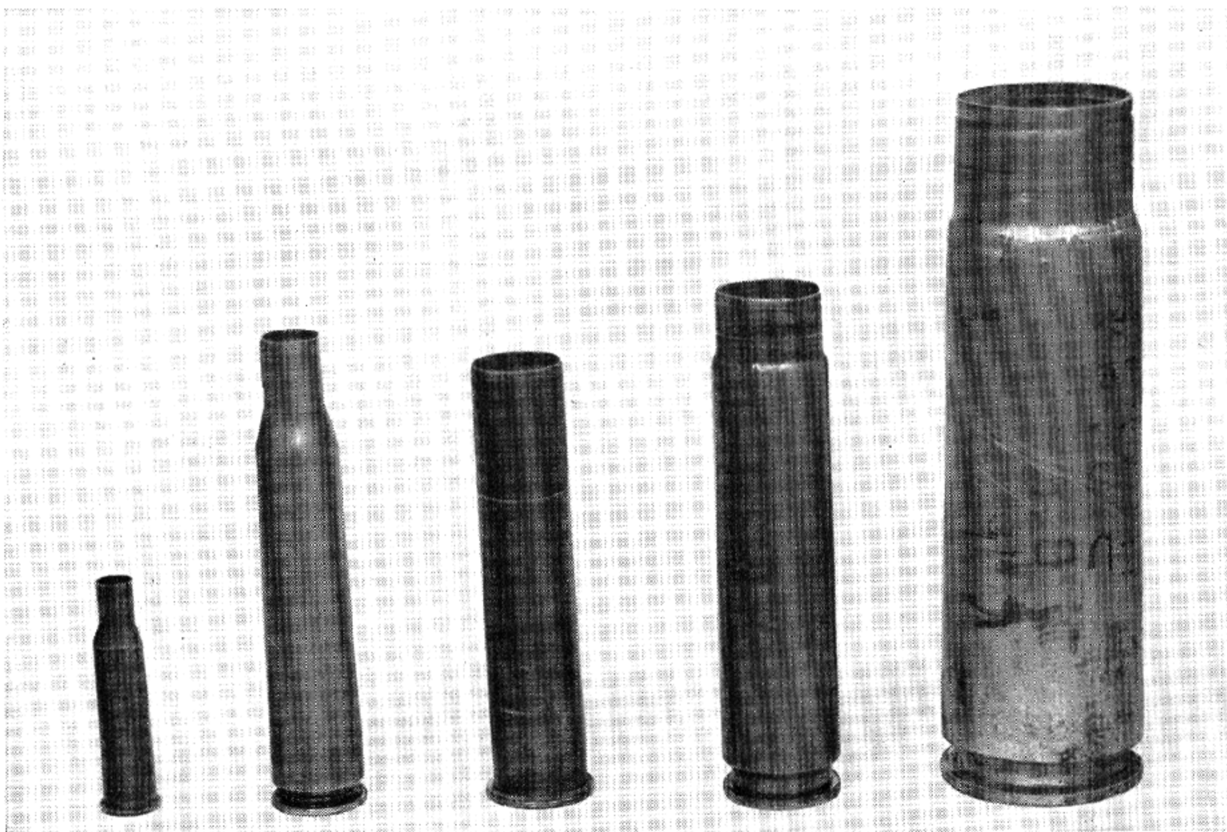
Figure 9-22. Comparison of profiles of Russian cartridge cases. Caliber of each case is given in figure 9-21, above.
