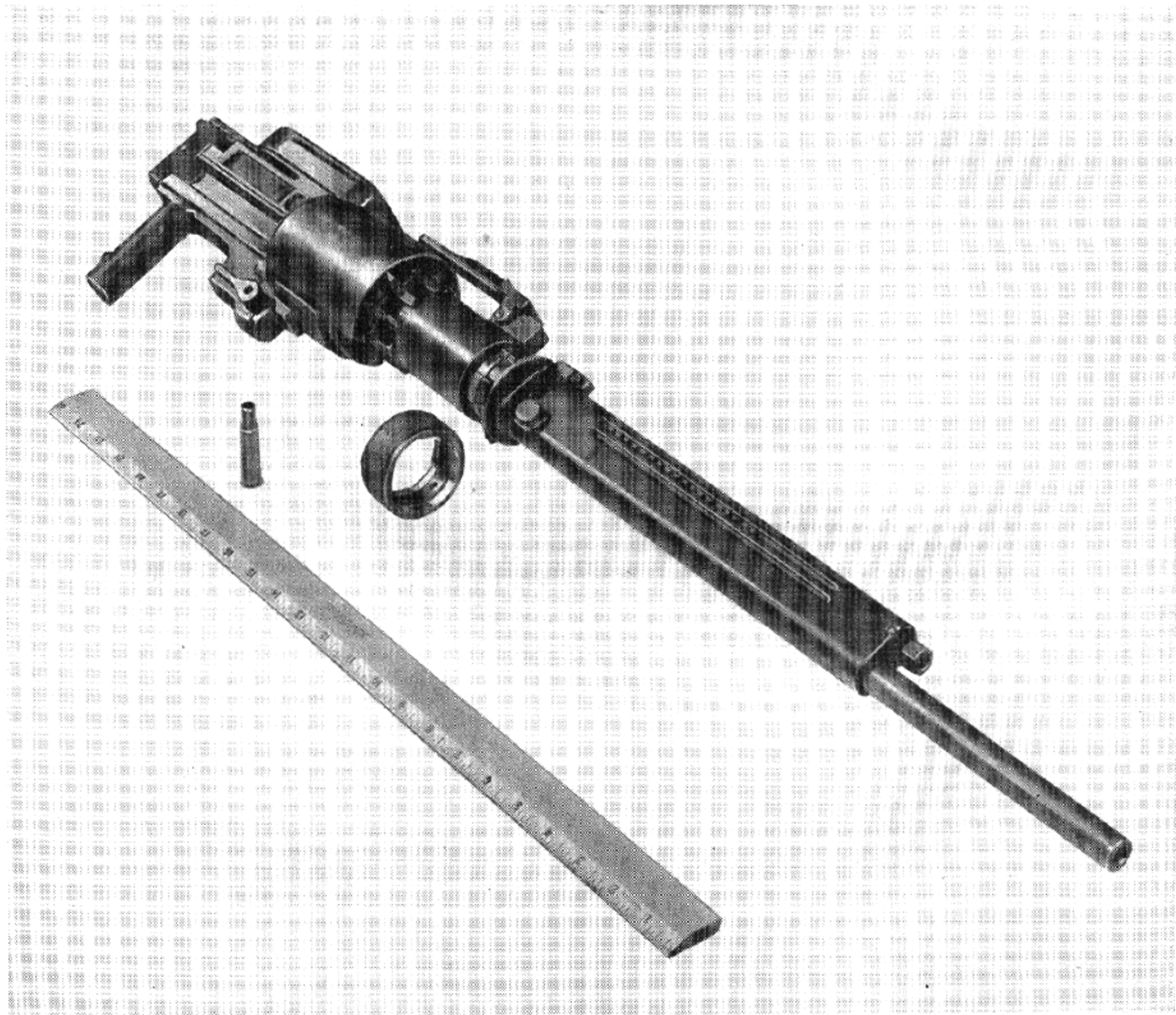
Figure 4-5. 7.62-mm Shkash Fixed Gun, captured from the Red Forces in Korea. Rear hand grip is a field improvisation. Barrel retaining collar has been removed to show securing lugs.
