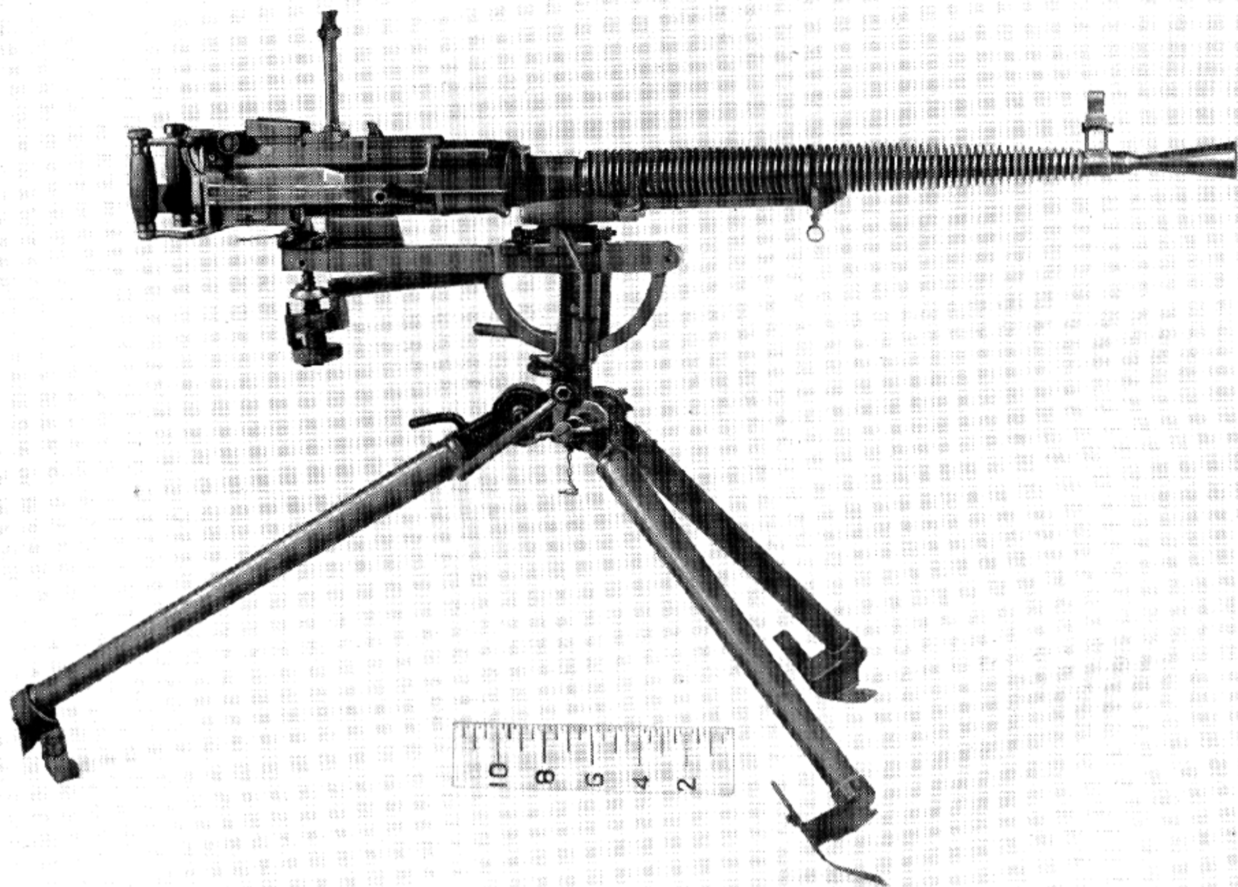
Figure 3-17. The 7.62-mm Degtyarev Belt-fed Machine Gun known as the DS. Very few specimens of this version are in existence.
