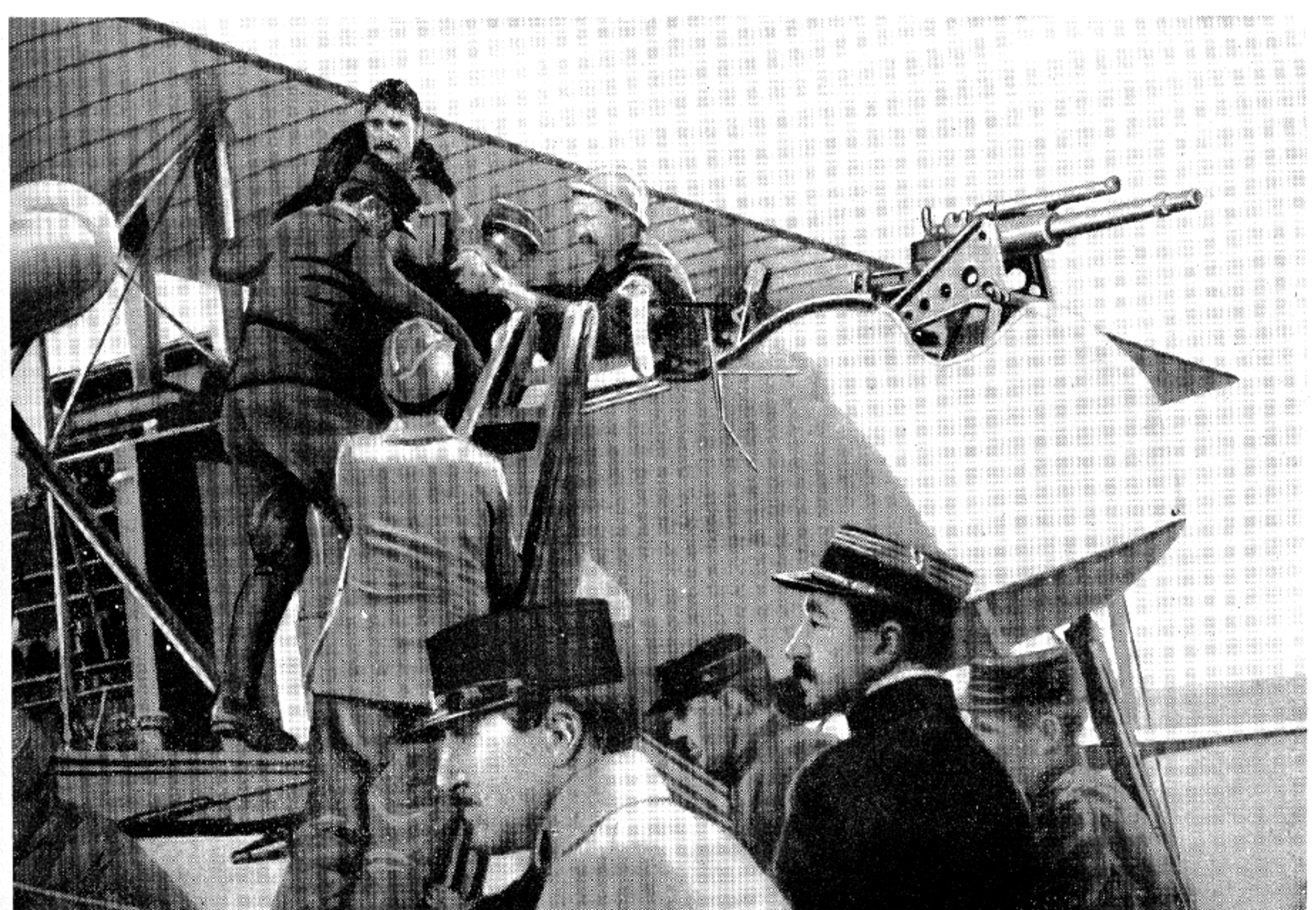
Puteaux 37-mm Aircraft Cannon (Semiautomatic) Mounted on a French Bombing Plane, 1916.
