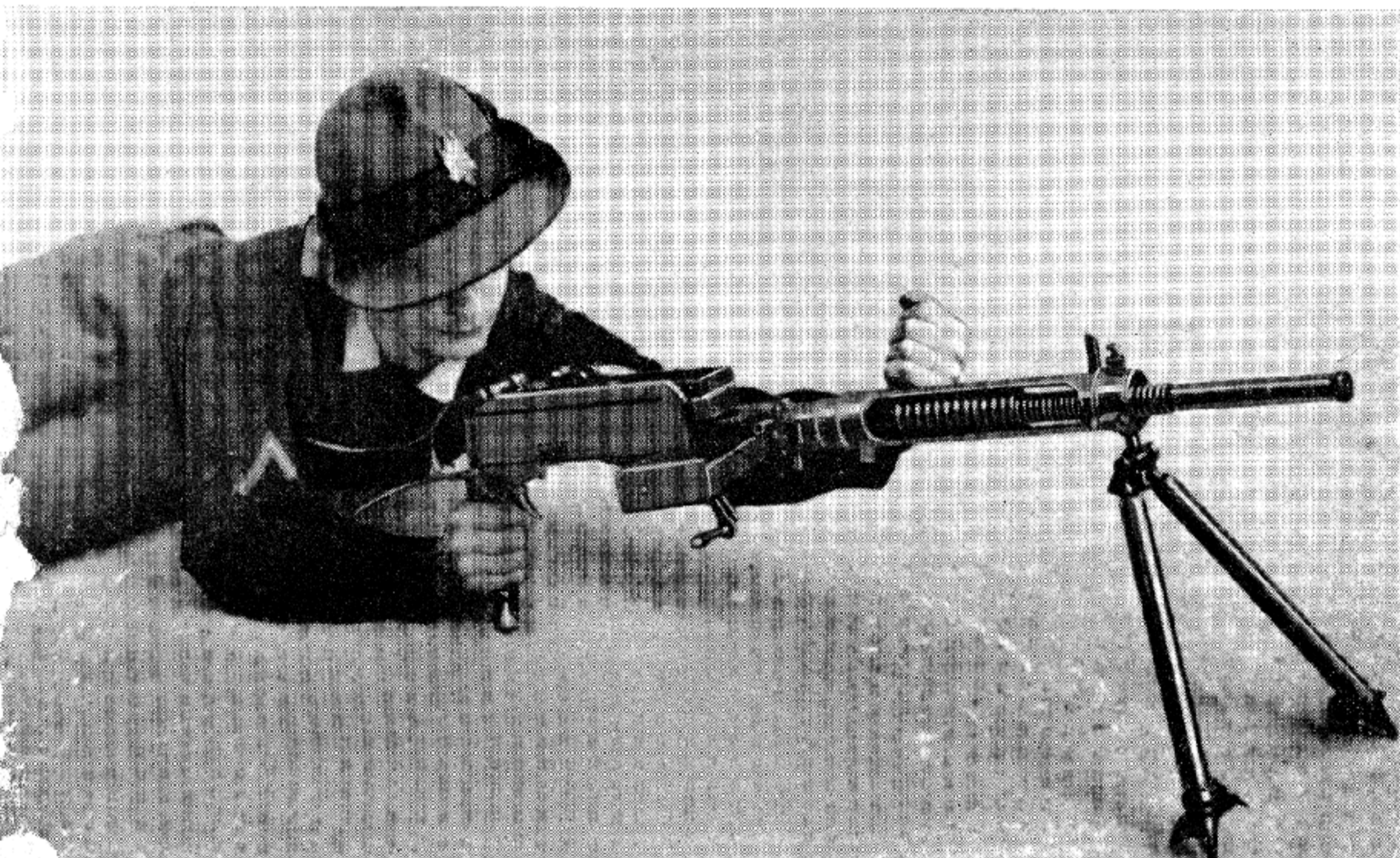
Sistar Light Machine Gun, 6.5 mm. The Operator Is Charging the Weapon.
