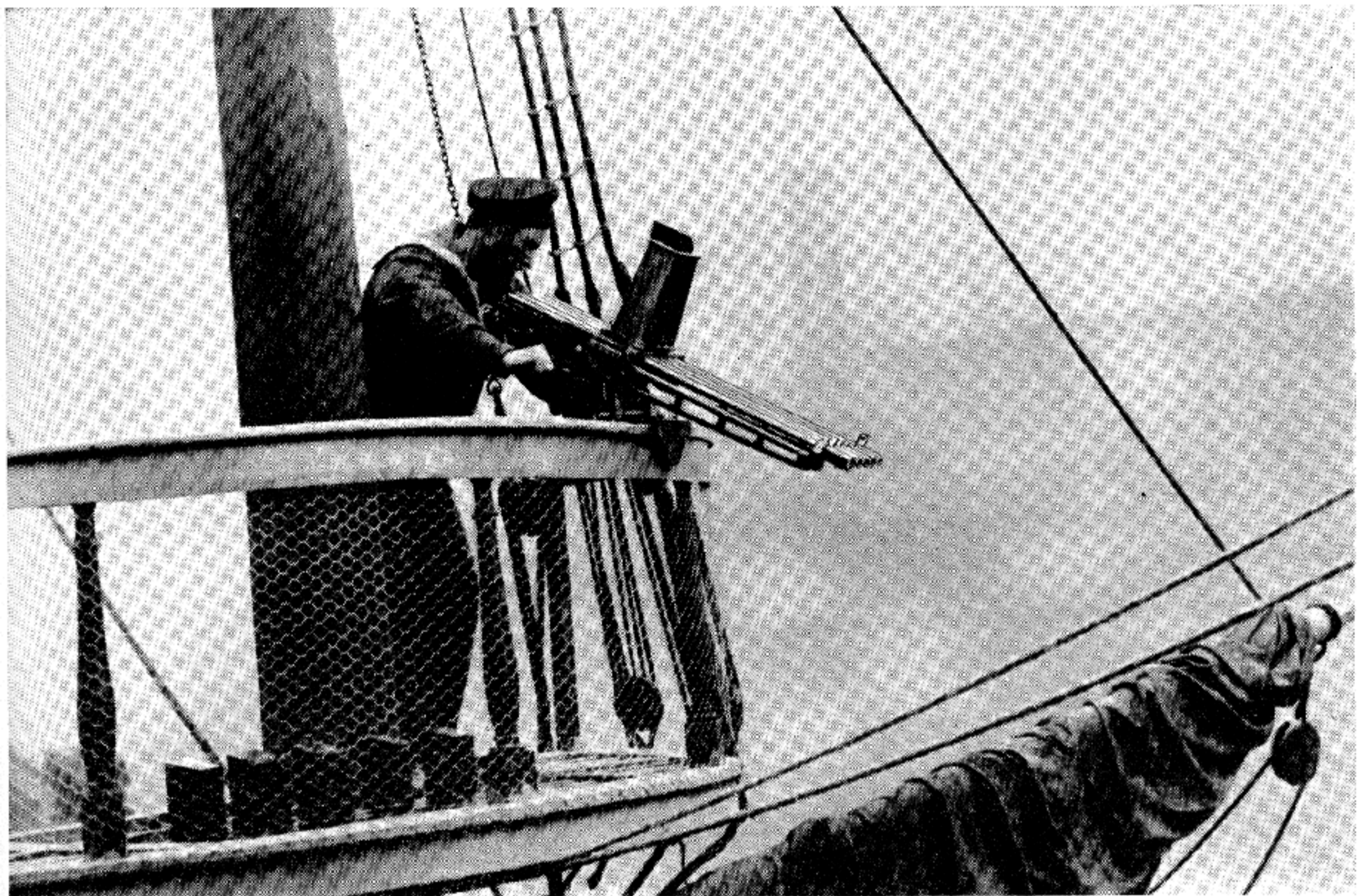
Nordenfelt Machine Gun, Cal. .45, Five-Barrel Model. Mounted in Top of a Fighting Ship to Sweep the Decks of the Enemy.
