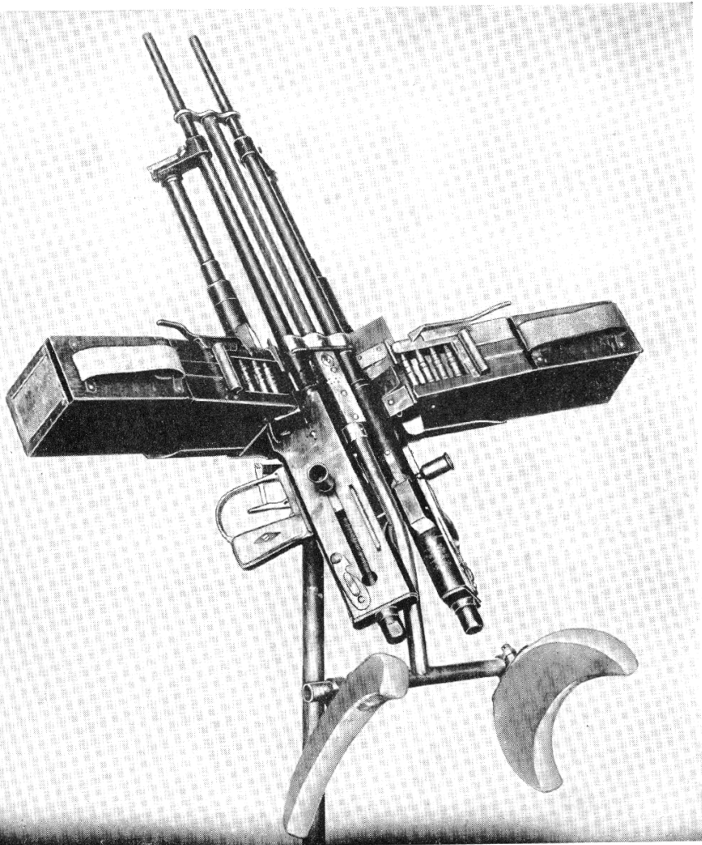
Darne Aircraft Machine Gun, 7.5 mm. Dual Flexible Mount.
