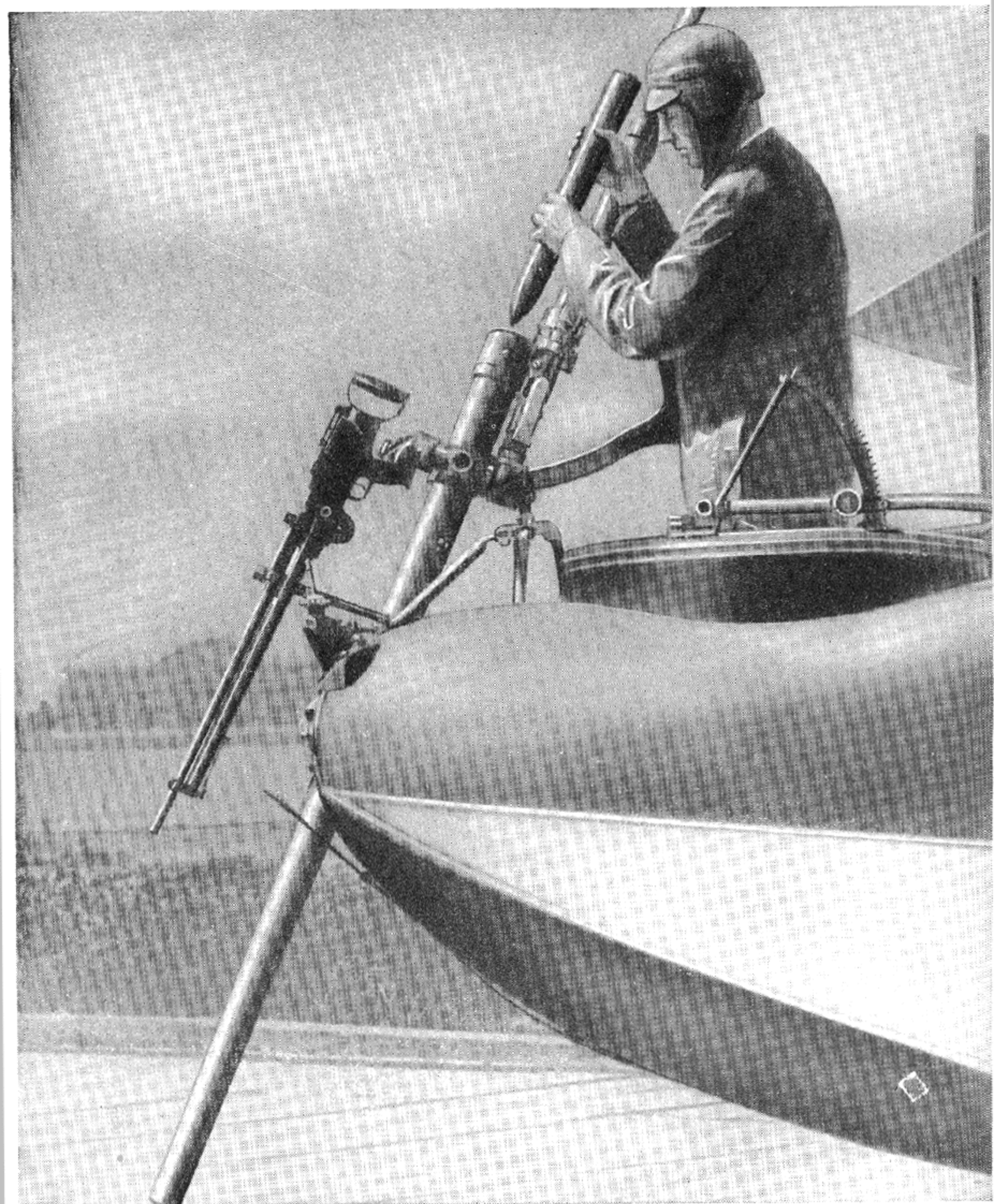
A Davis Gun Mounted on a Naval Seaplane. The Gunner Has Pivoted the Breech to the Open Position for Loading.
