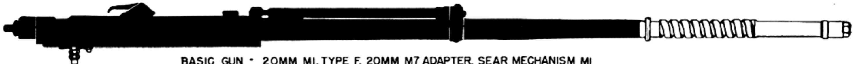
BASIC GUN - 20 MM AN - M2, TYPE E, 20MM AN - MI ADAPTER, ELECTRIC TRIGGER AN - MI, HYDRAULIC CHARGER M1
