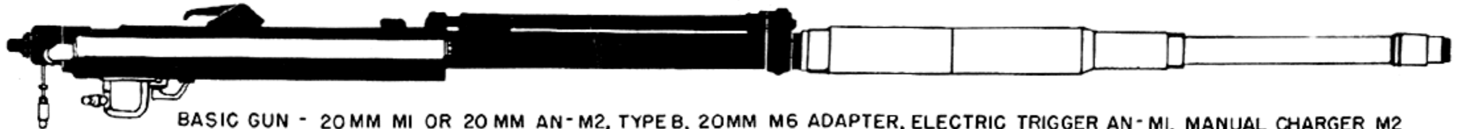
BASIC GUN - 20 MM MI OR 20 MM AN - M2, TYPE A, 20MM AN - MI ADAPTER, ELECTRIC TRIGGER AN - MI, MANUAL CHARGER M2
