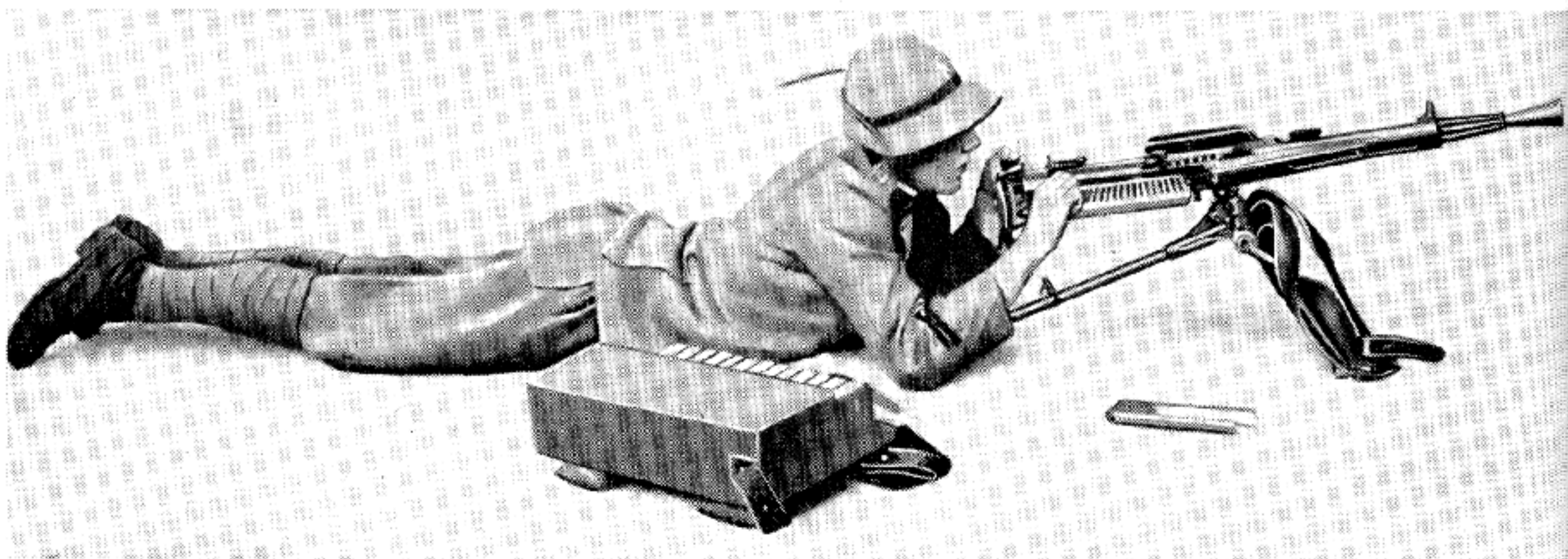
Breda Machine Gun, Model 1924, 6.5 mm. The Operator is Loading the Weapon.
