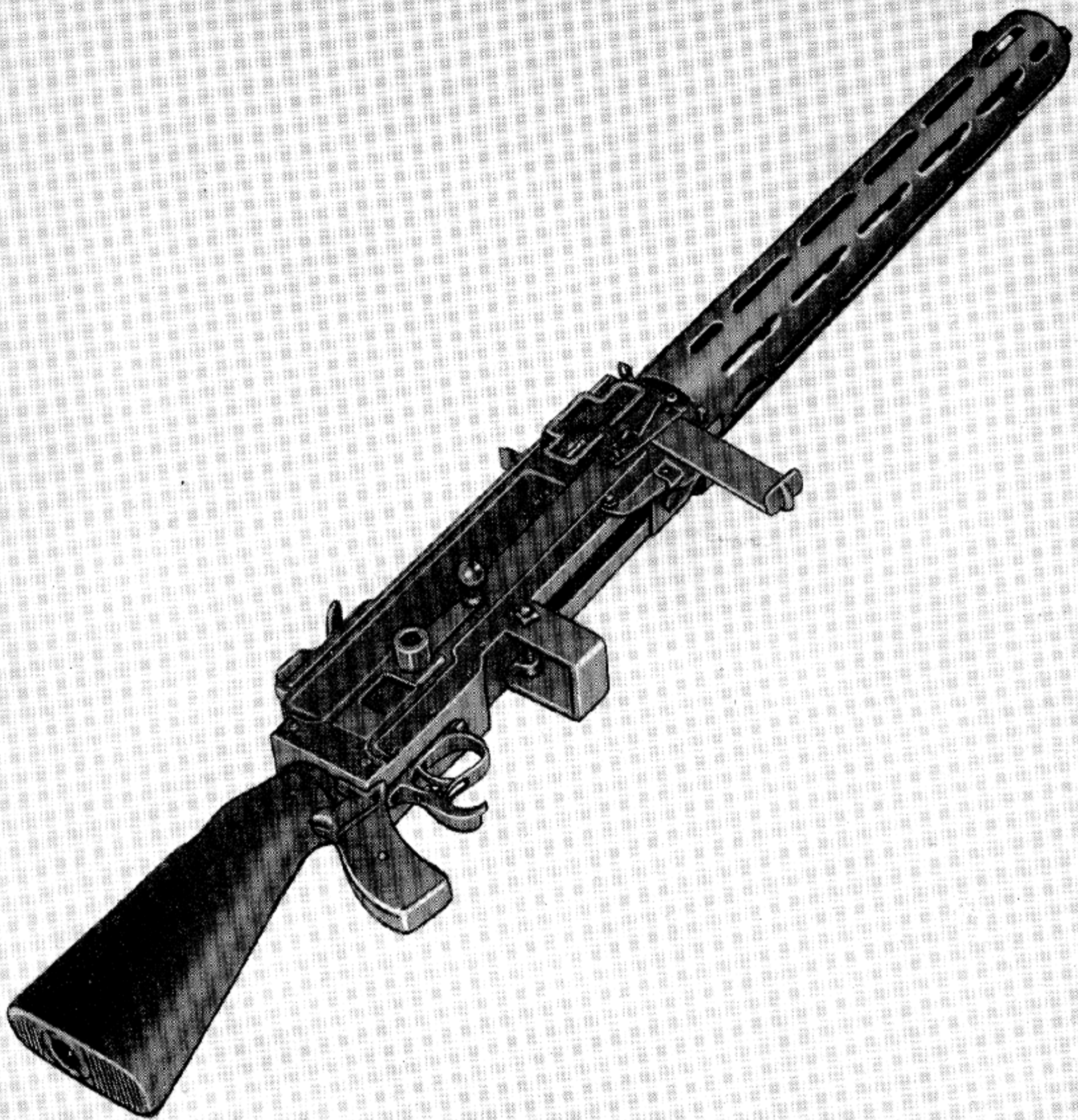
Parabellum Aircraft Machine Gun, Model 1913, 7.92 mm. This Early Type Used the Water-Cooled Jacket Slotted for Air Cooling.
