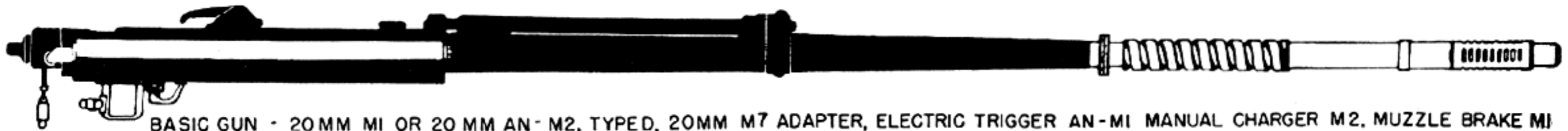
BASIC GUN - 20 MM MI OR 20 MM AN - M2, TYPE C, 20MM M7 ADAPTER, ELECTRIC TRIGGER AN - MI, MANUAL CHARGER M2
