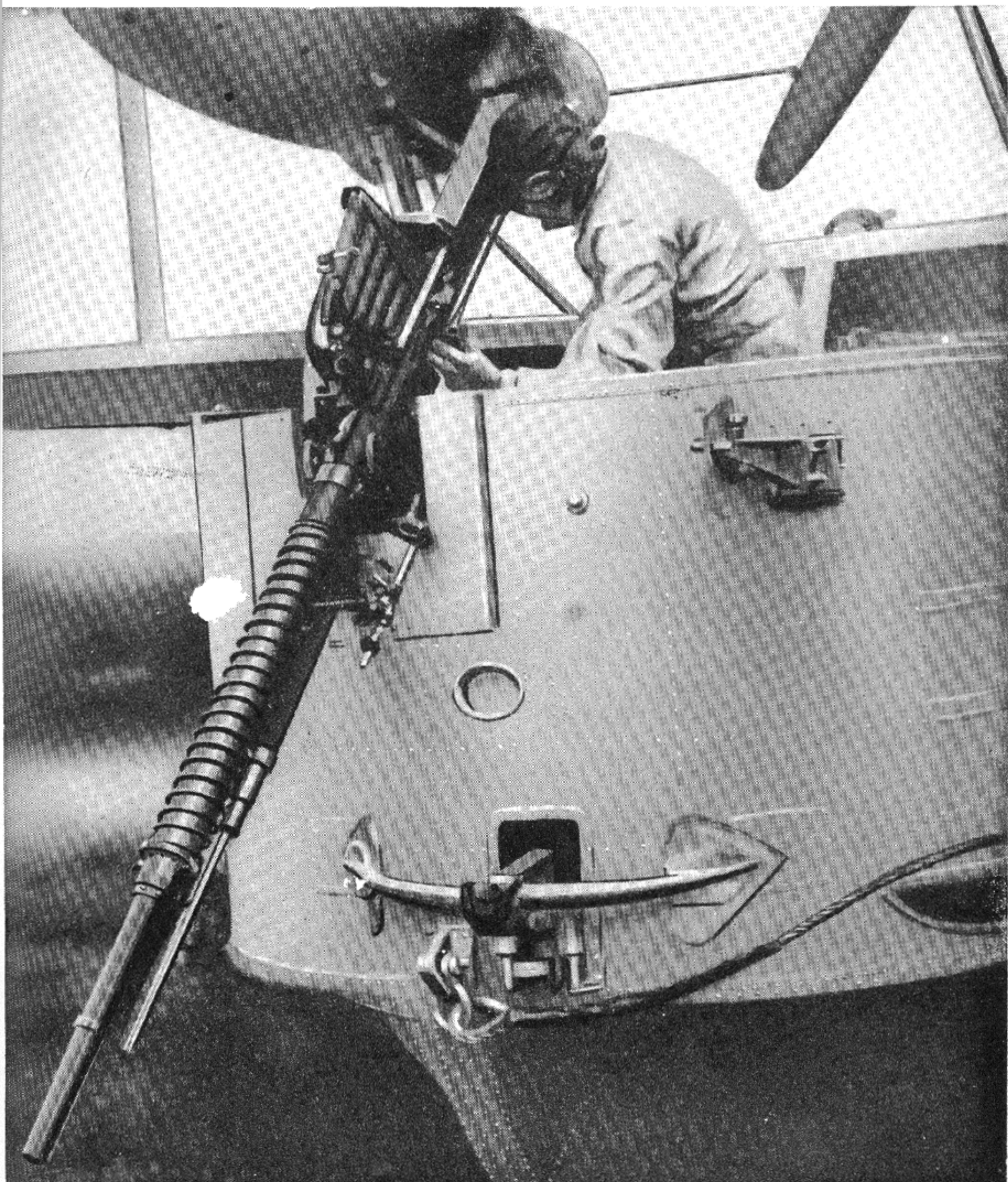
Vickers-Armstrong 37-mm Automatic Aircraft Cannon, Mounted in a Blackburn "Perth" Flying Boat.
