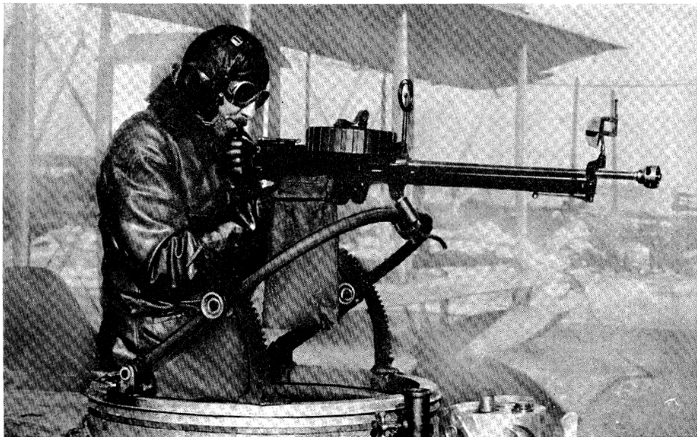
Flexible Lewis Machine Gun Mounted on a Scarff Ring.
