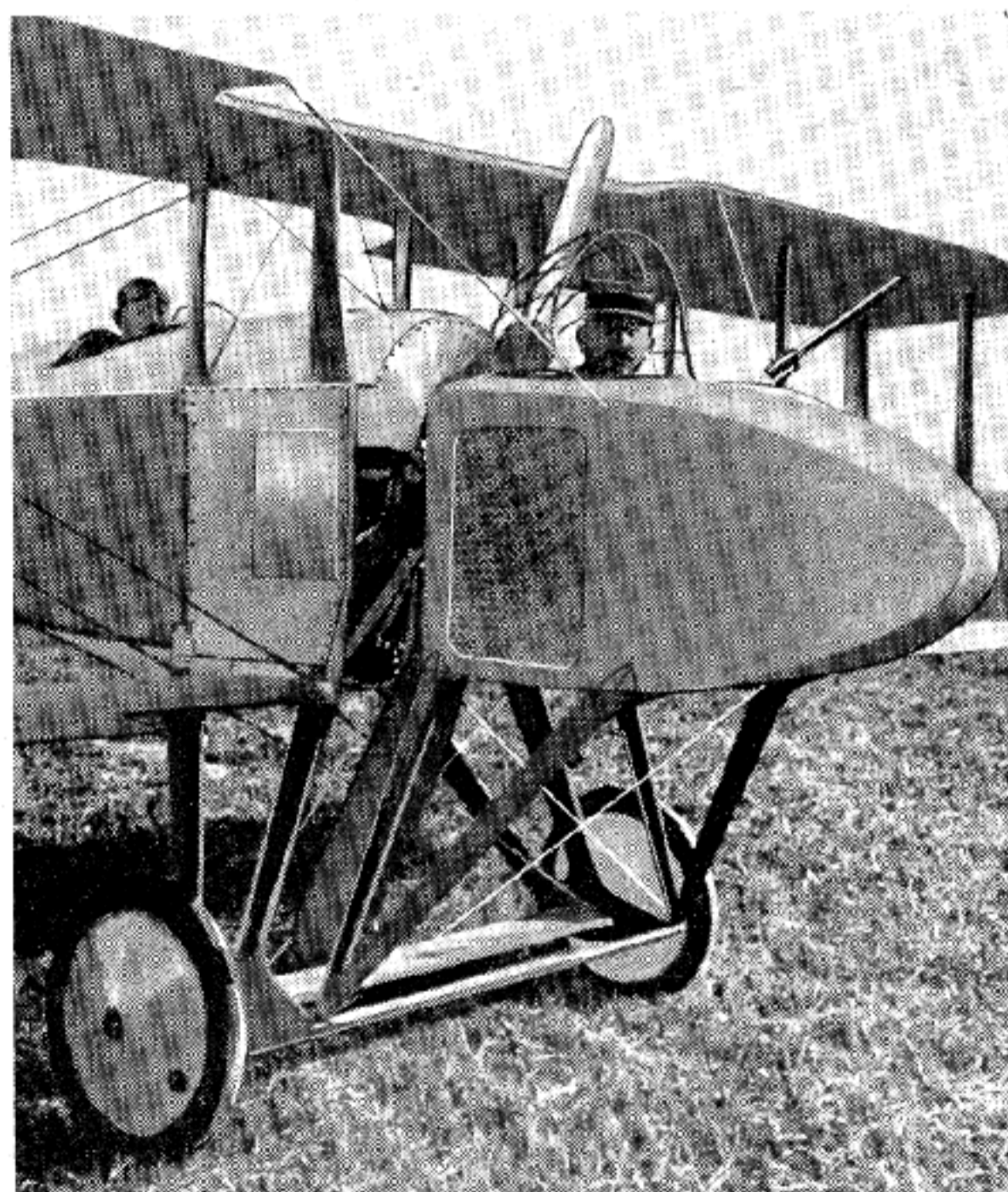
An Early Front-Gun Spad with False Nose to Accommodate Gunner.
