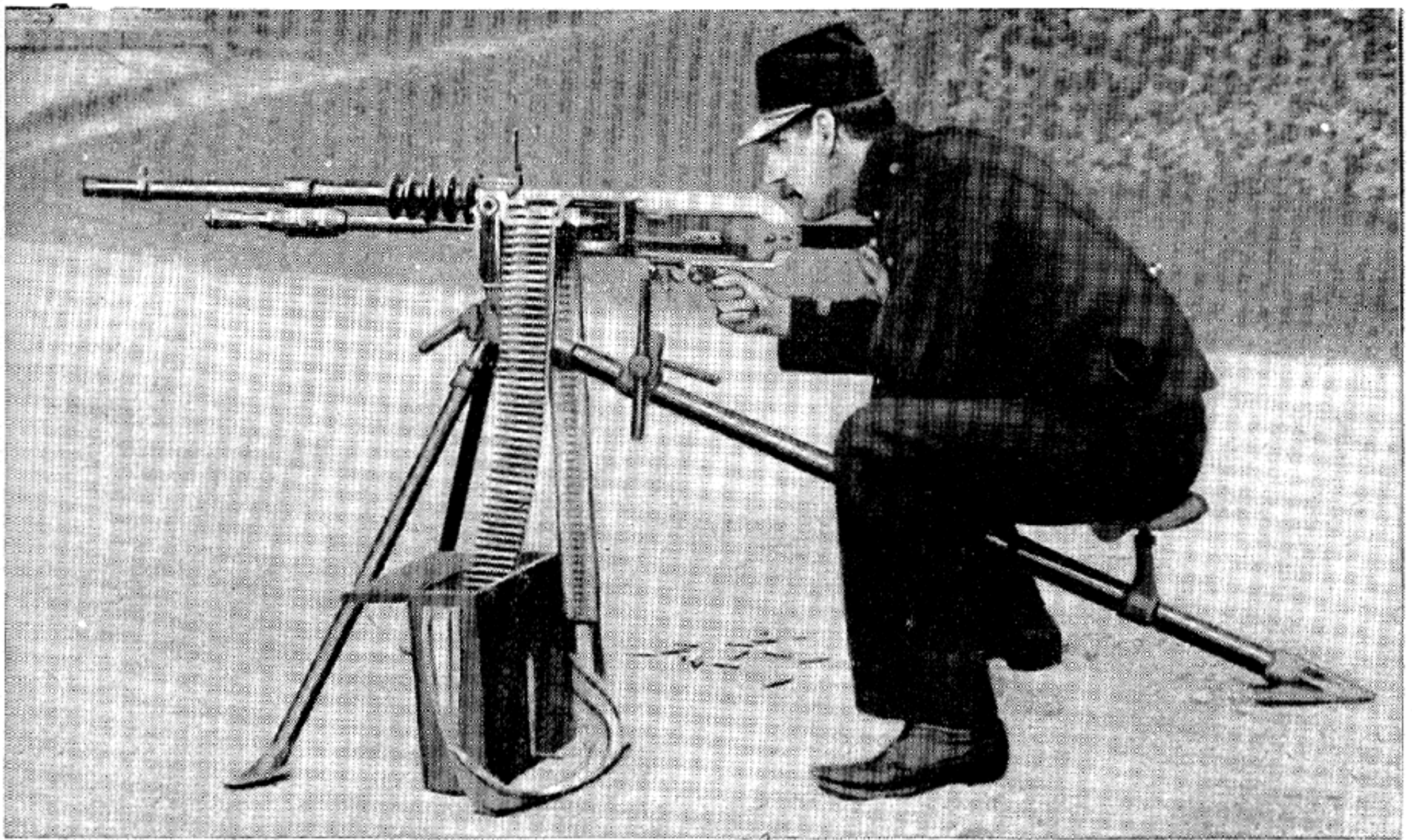
Hotchkiss Machine Gun, Model 1903. The First Hotchkiss Gun to Use a Belt Feed.
