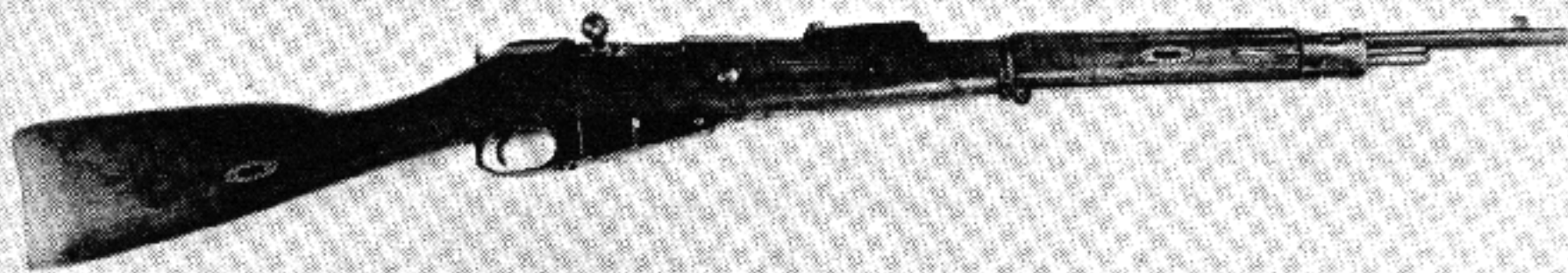
Polish 7.92mm M91/98/25 Rifle—an alteration of the Russian M91 rifle.
