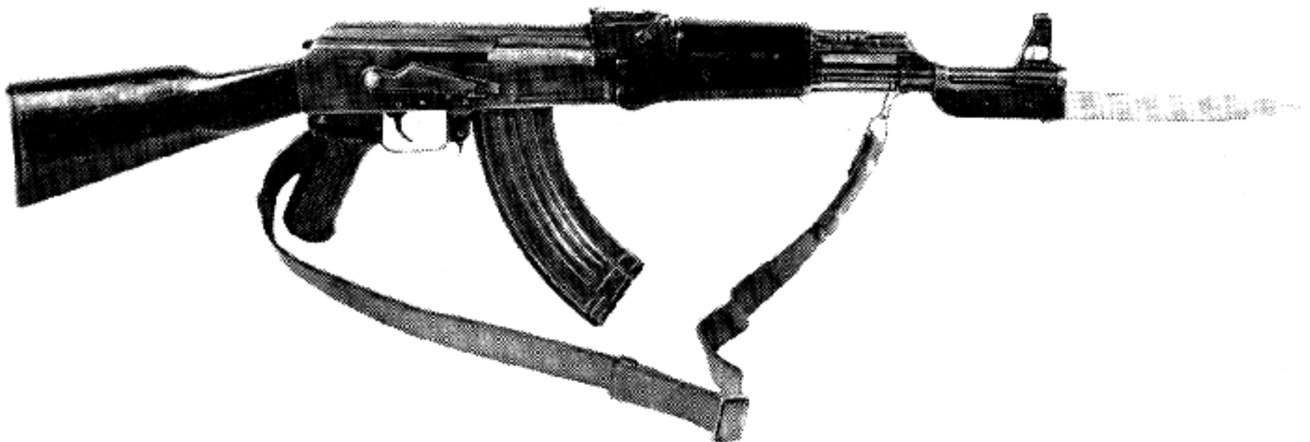
Soviet-Designed, Bulgarian-Made 7.62mm AK-47 Assault Rifle.
