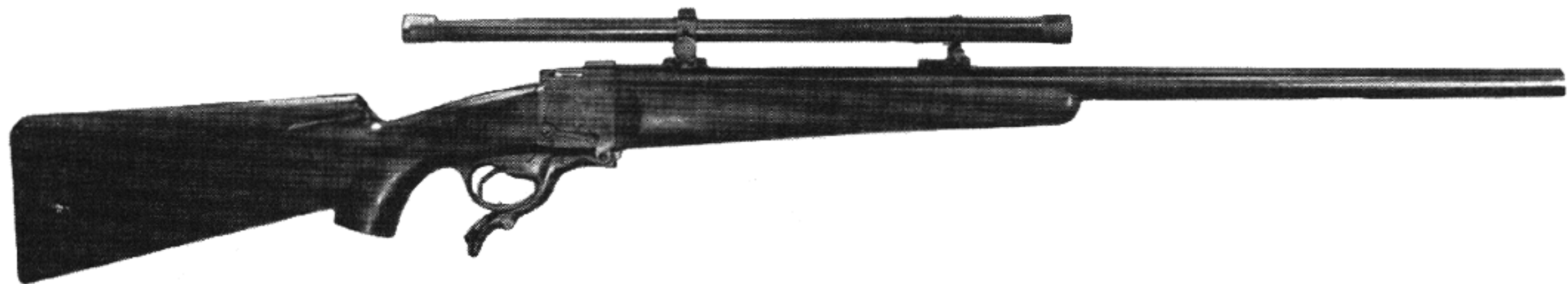
British Farquaharson Dropping Block Rifle. This is one of the strongest single shot actions ever developed. This lock design may be encountered in any caliber, since these actions were barreled up to custom order. The special lever under the triggerguard provides greater extracting power.
