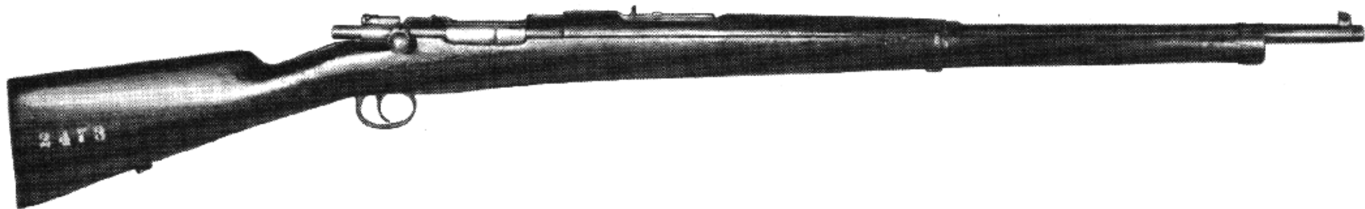
Spanish 7mm Mauser Model 1893. The rifle is shown cocked.
