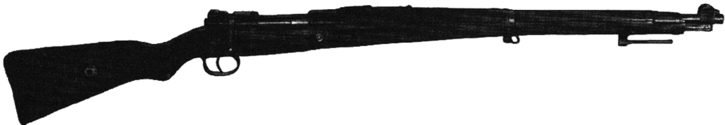
Polish Karabinek 1898, caliber 7.9mm. Except for minor details such as the shape of the stacking swivel and sling on underside this is the German Kar. 98.
