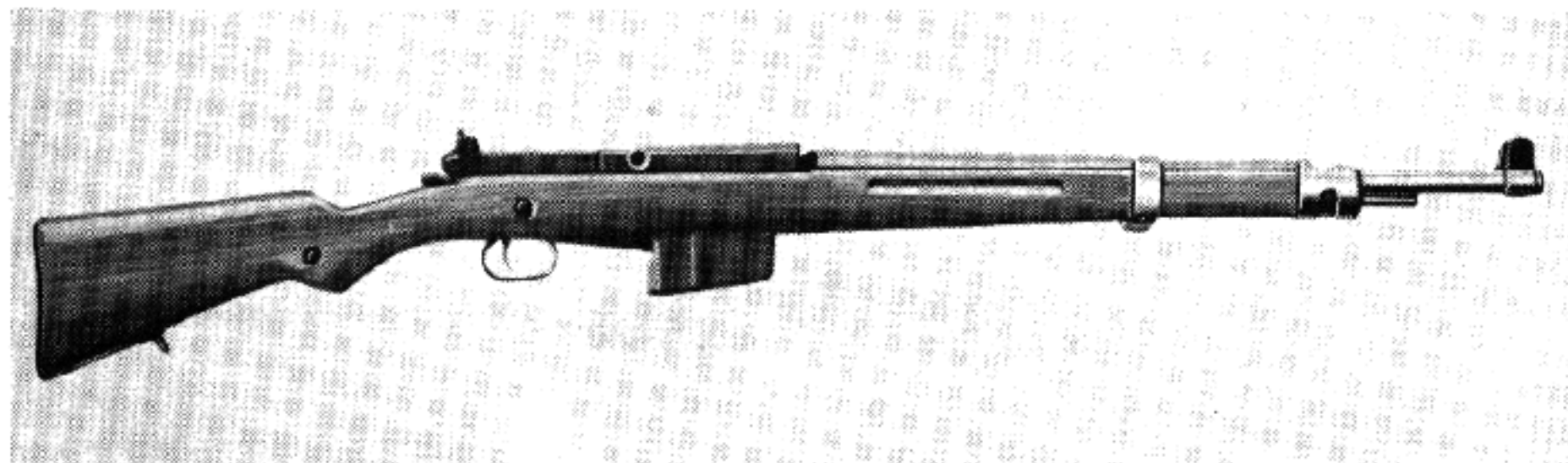
The Pelo Semiautomatic Rifle. This rifle was developed by a Finnish Captain. The prototypes were manufactured in Sweden in 6.5mm and 7.92mm and the weapon was tested by the Swedish and British governments after World War II. The Pelo has a ten-round magazine and is 43.3 inches overall. It weighs 9.25 pounds and is an interesting example of a post-war prototype rifle.
