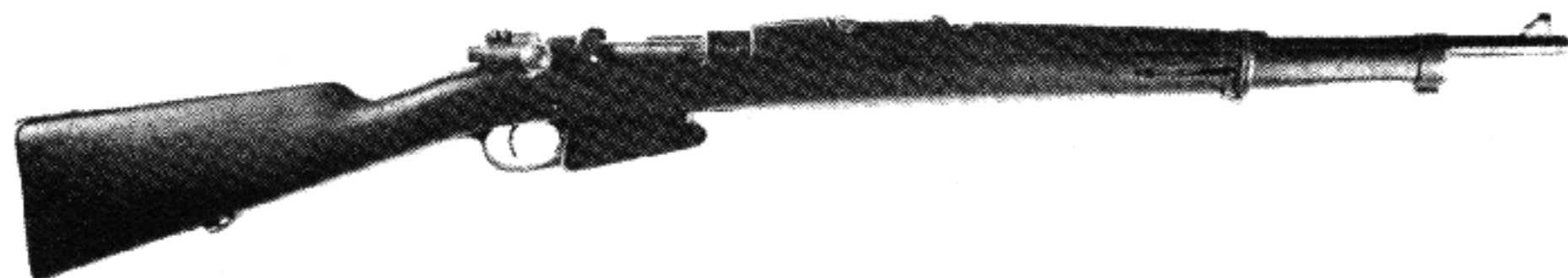
Yugoslav 7.92mm M90T; this is the Turkish 7.65mm cut down and rebarreled to 7.92mm.
