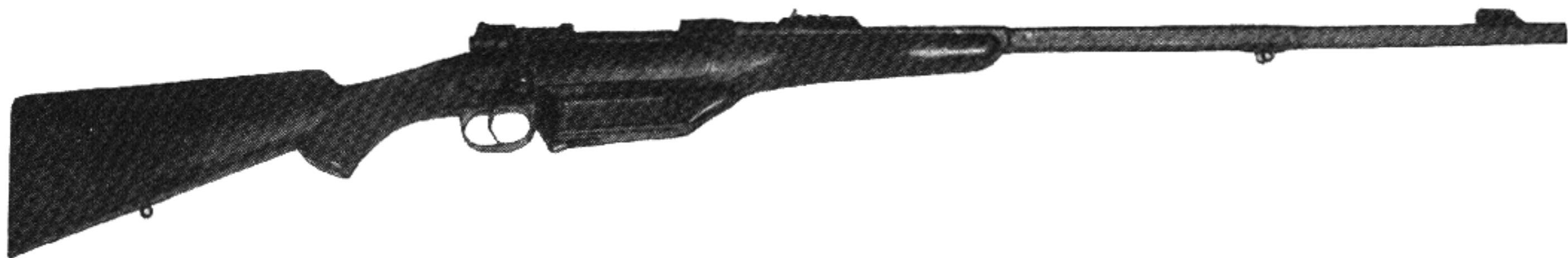
Pre-war British Westley Richards .425 Express Rifle. This is a typical custom built express rifle using a Mauser Magnum receiver. Stocks, sights, barrel lengths and similar details vary with individual specimens as ordered. The protruding box magazine is necessary because of the large size of the special cartridges used.
