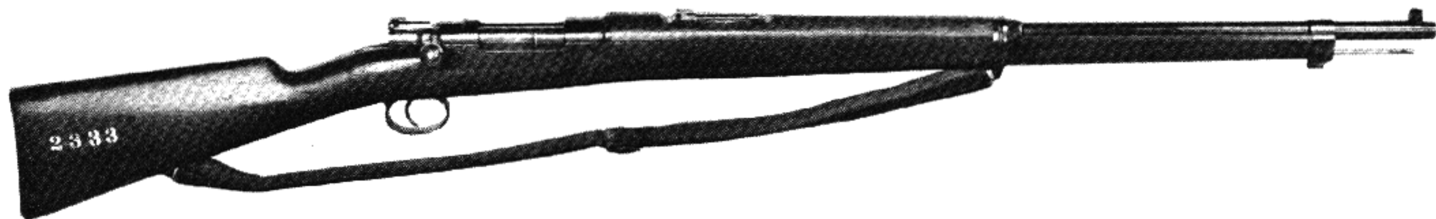
Chilean Mauser M1895 7mm Rifle, made in Germany. This rifle is essentially the 7mm Spanish M1893 Rimless.
