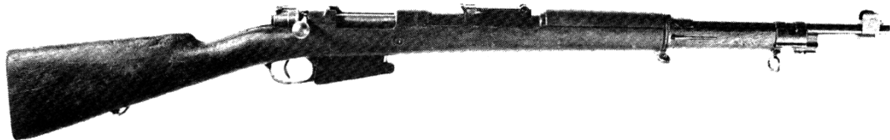
Belgian 7.65mm M1936 Service Rifle. This weapon is a conversion of M1889 Rifles and Carbines. It has a 98 Mauser type bolt sleeve and firing pin mechanism.
