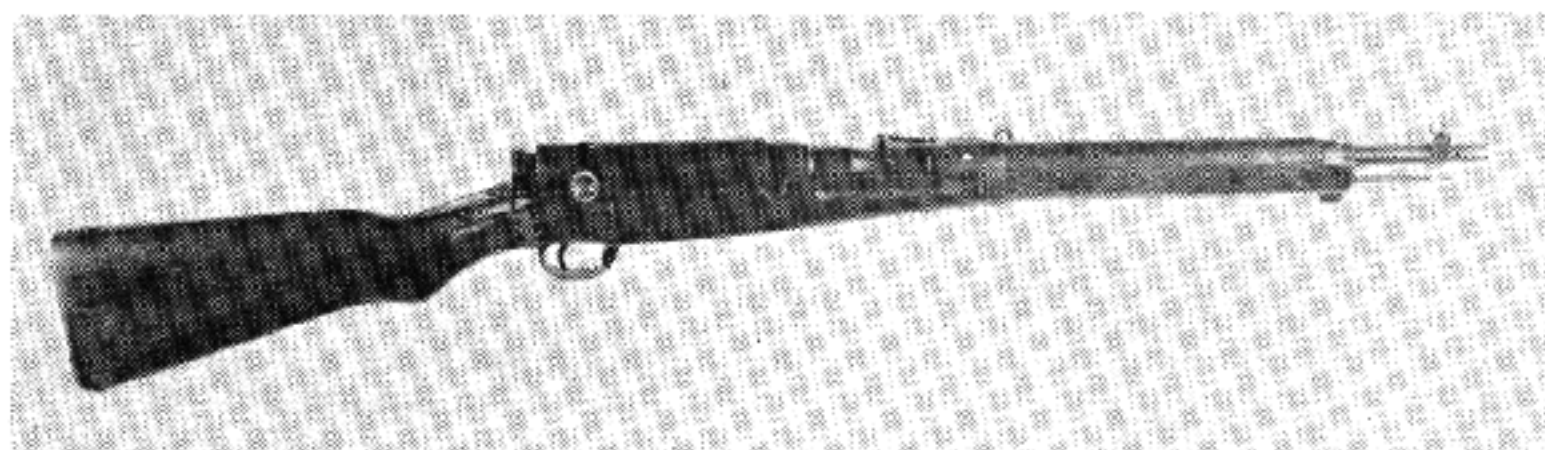
Japanese 6.5mm Type 38 Carbine; Converted to a Paratrooper Model by Hinging the Stock.
