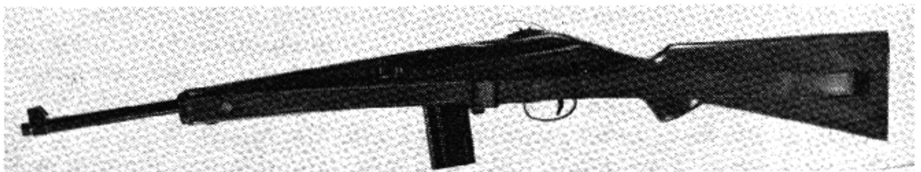
French Caliber 30 MAC 1949 Carbine.
