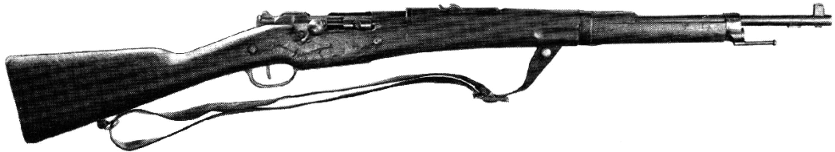
French 7.5mm Model 07/15M34 rimless. Modified 5-shot magazine to permit strip loading from standard Mauser-pattern clips.
