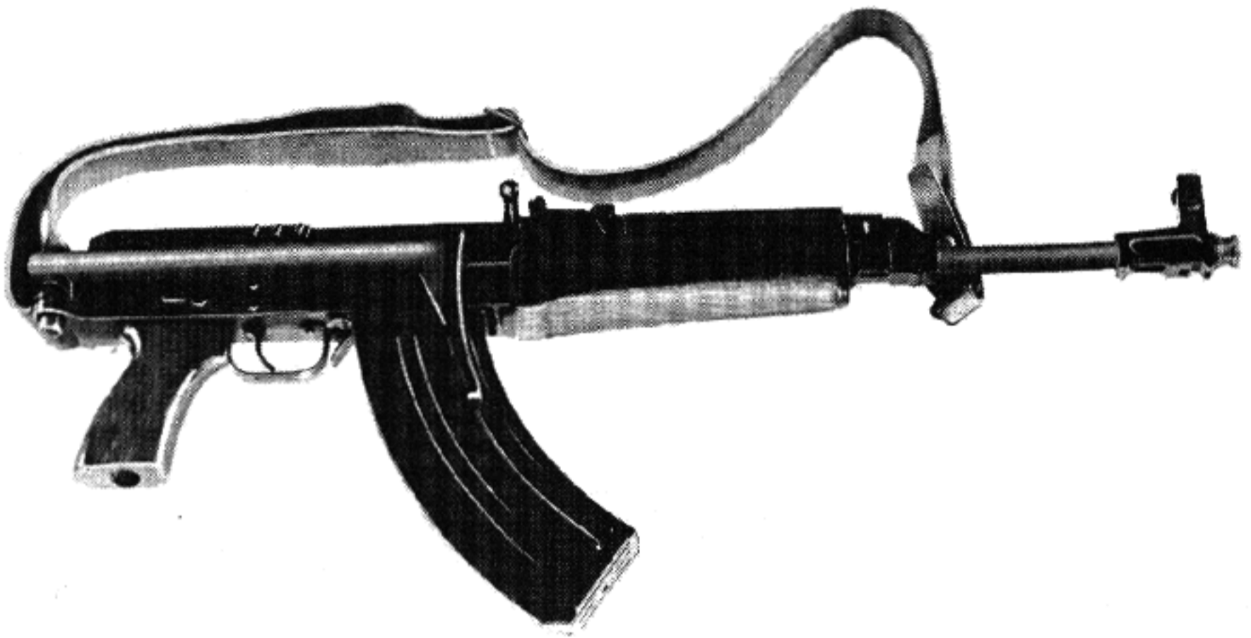
Czech 7.62mm Model 58 Assault Rifle with Folding Stock, Stock Folded.
