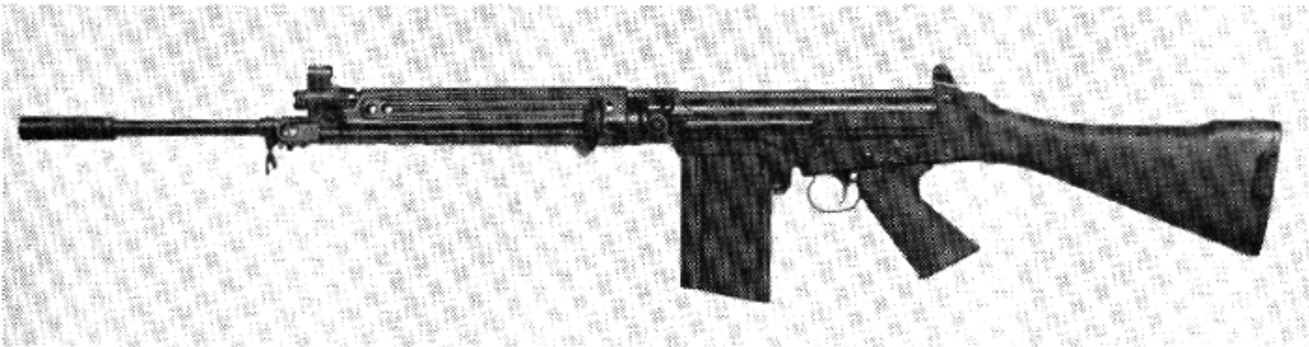
FN 7.62mm NATO Light Automatic Rifle. This version was made for the Netherlands. Attention is called to the bipod and the metal handguards.
