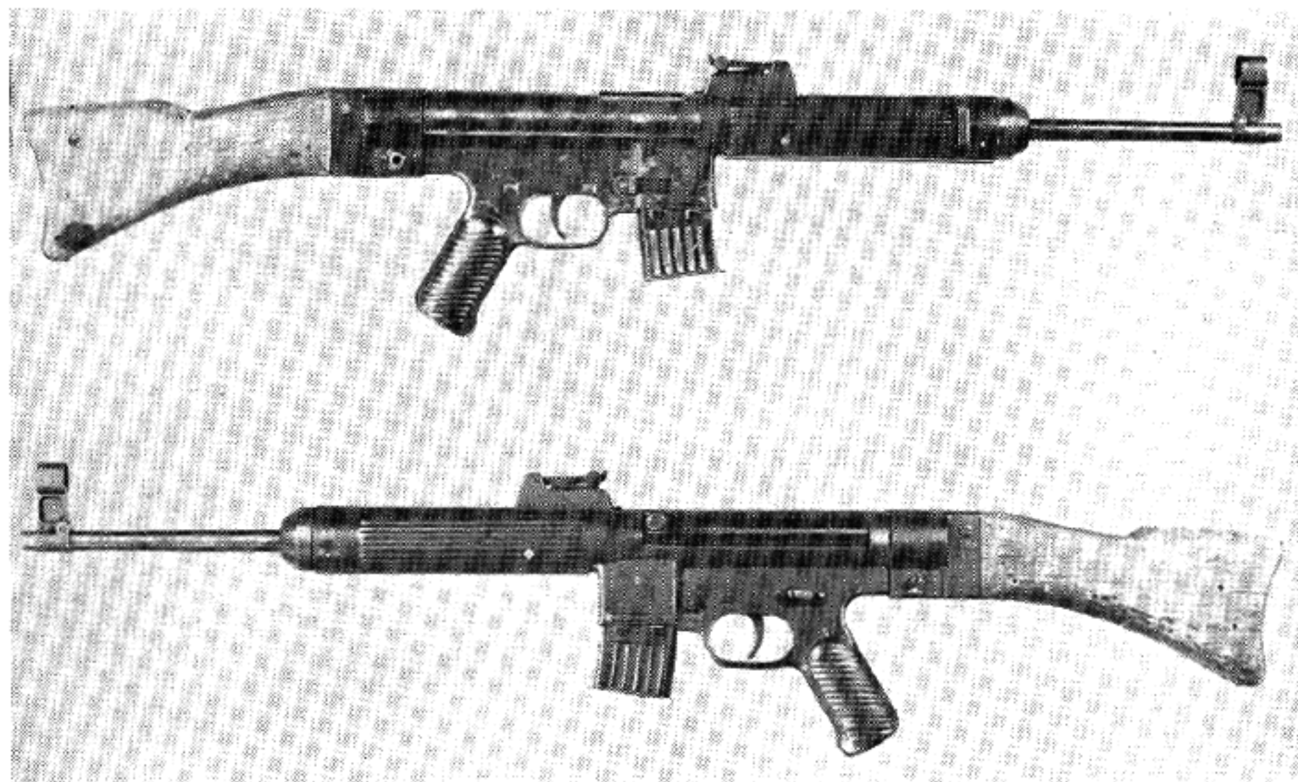
Mauser Prototype Assault Rifle, the 7.92mm StG-45 (M). This weapon, sometimes called Gerät 06 (H), has the delayed blowback locking mechanism currently used in the German G3, and the Spanish CETME.
