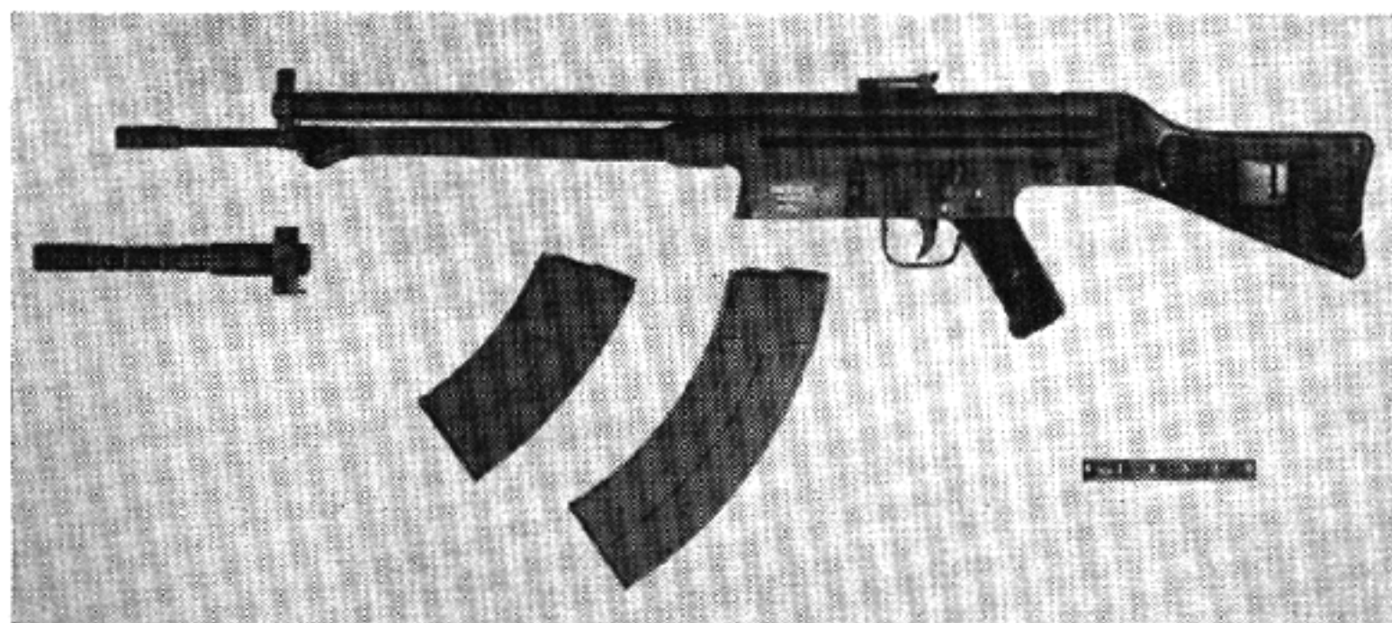
Prototype 7.92mm CETME Assault Rifle shown with grenade launcher, 32-round magazine, and 20-round magazine.
