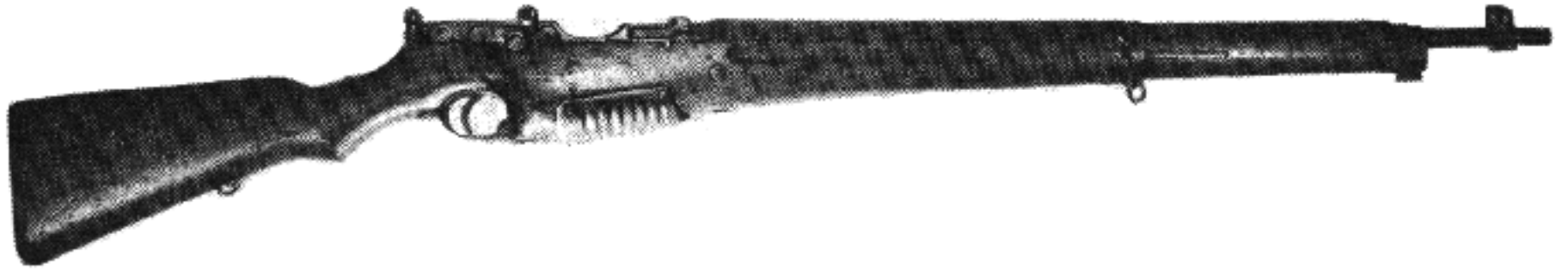
Japanese Copy of Pedersen Semiautomatic Rifle. This weapon has a rotary type magazine.
