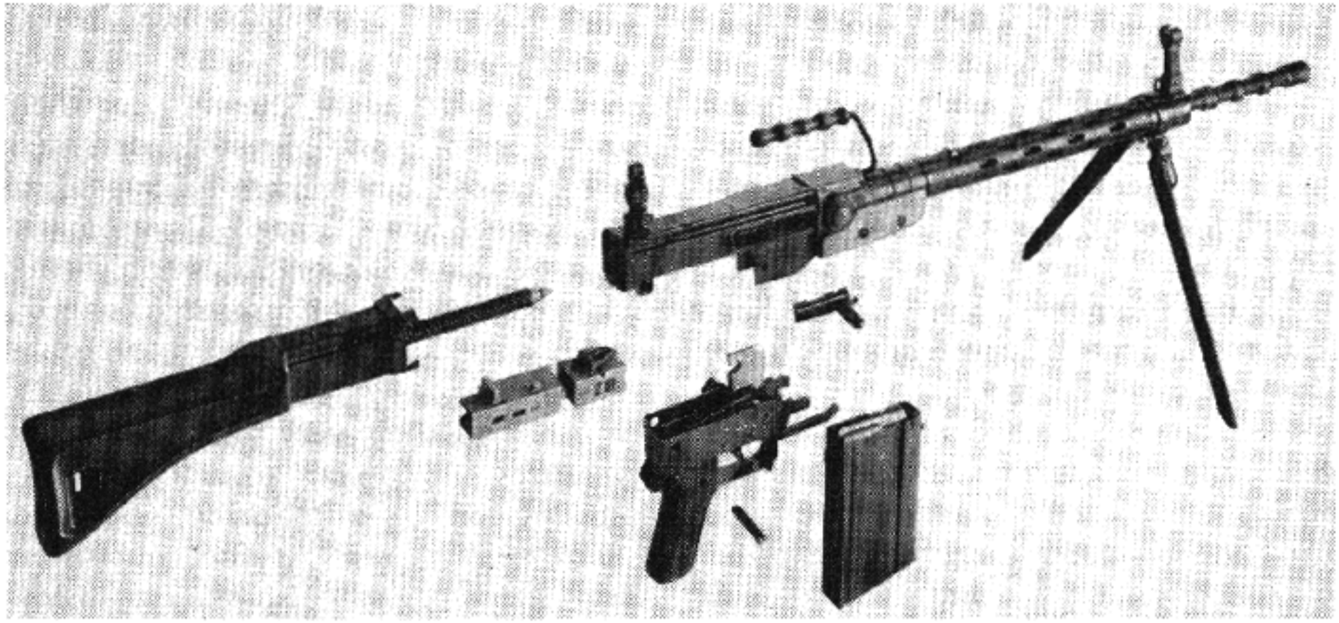
Swiss SIGw Model 57 Assault Rifle, Stripped.
