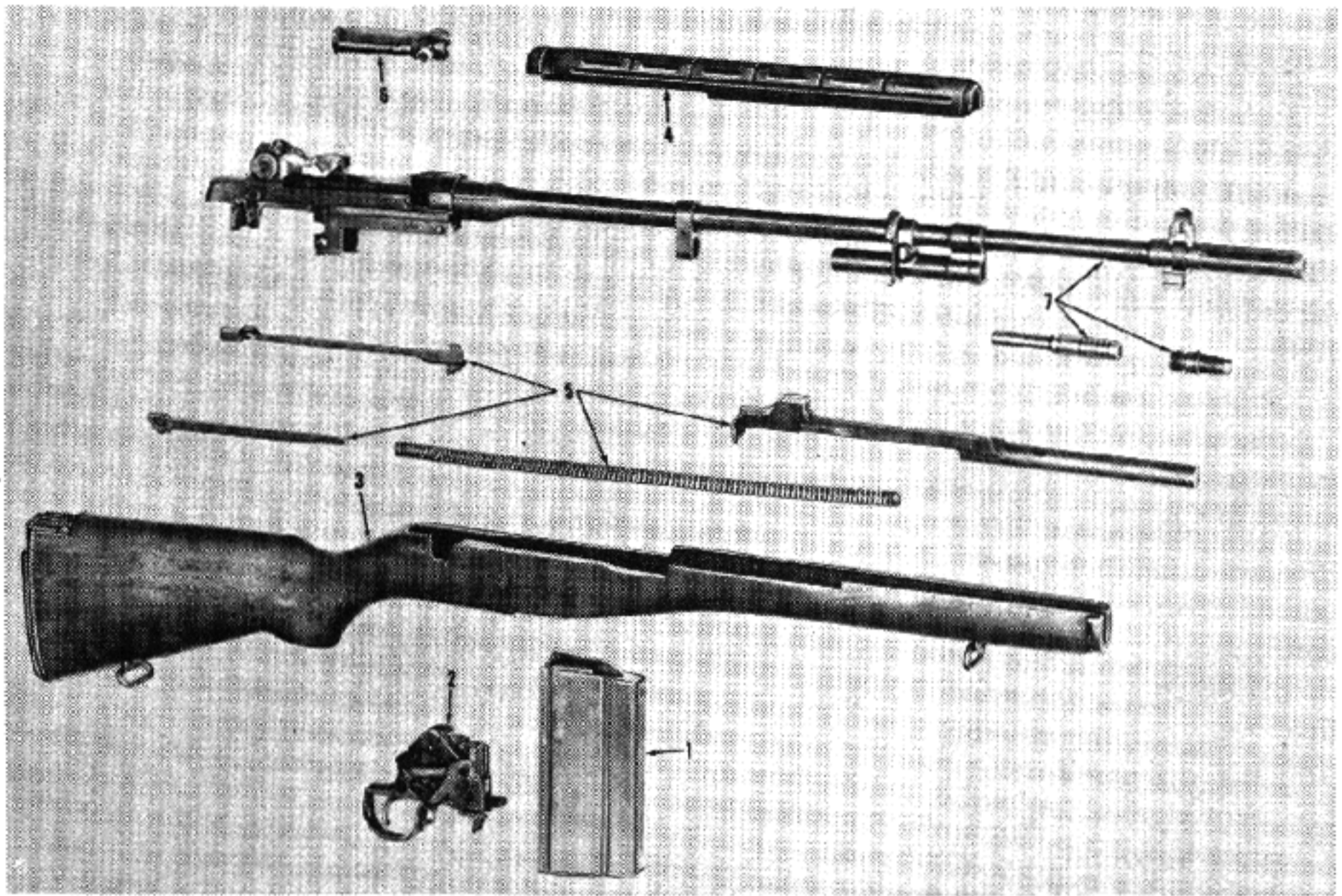
U. S. 7.62mm Rifle M14, Field Stripped. 1, Magazine. 2, Trigger mechanism. 3, Stock. 4, Handguard. 5, Operating Rod Assembly. 6, Bolt. 7, Gas Piston, Gas Cylinder Valve, and Barrel.
