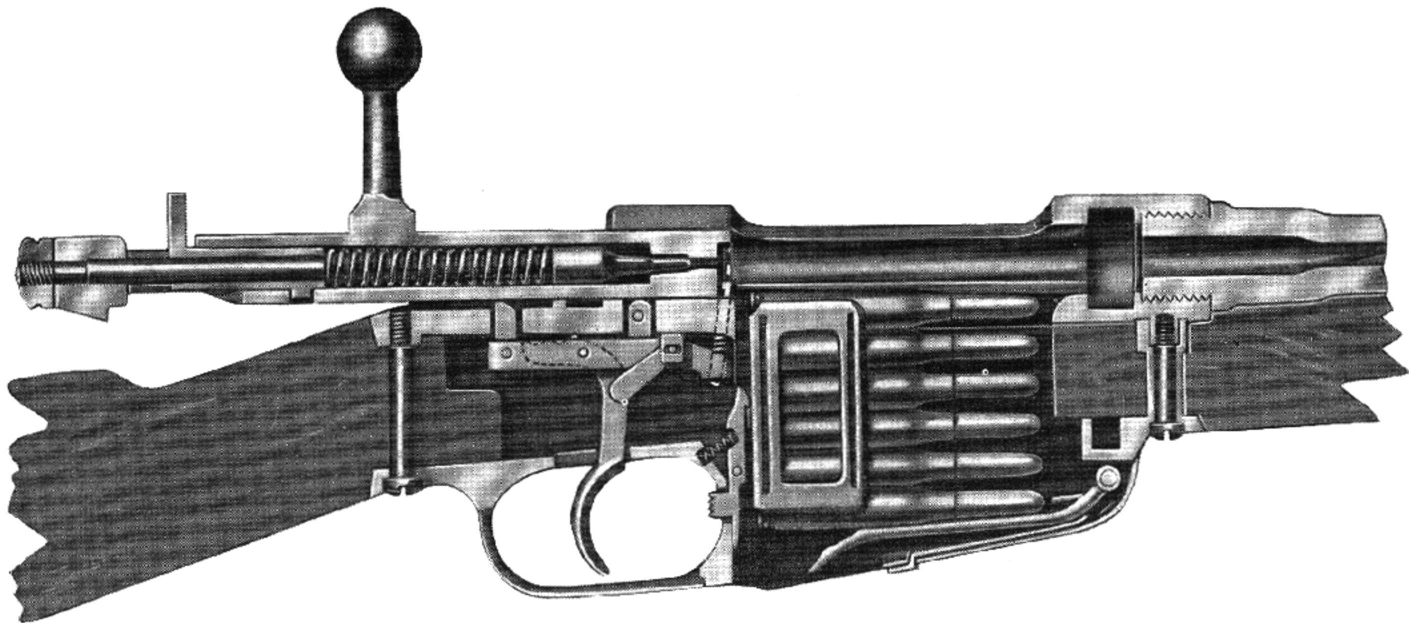
Italian M 91, Sectional Drawing Showing Action Open and Magazine loaded ready for forward bolt stroke.
