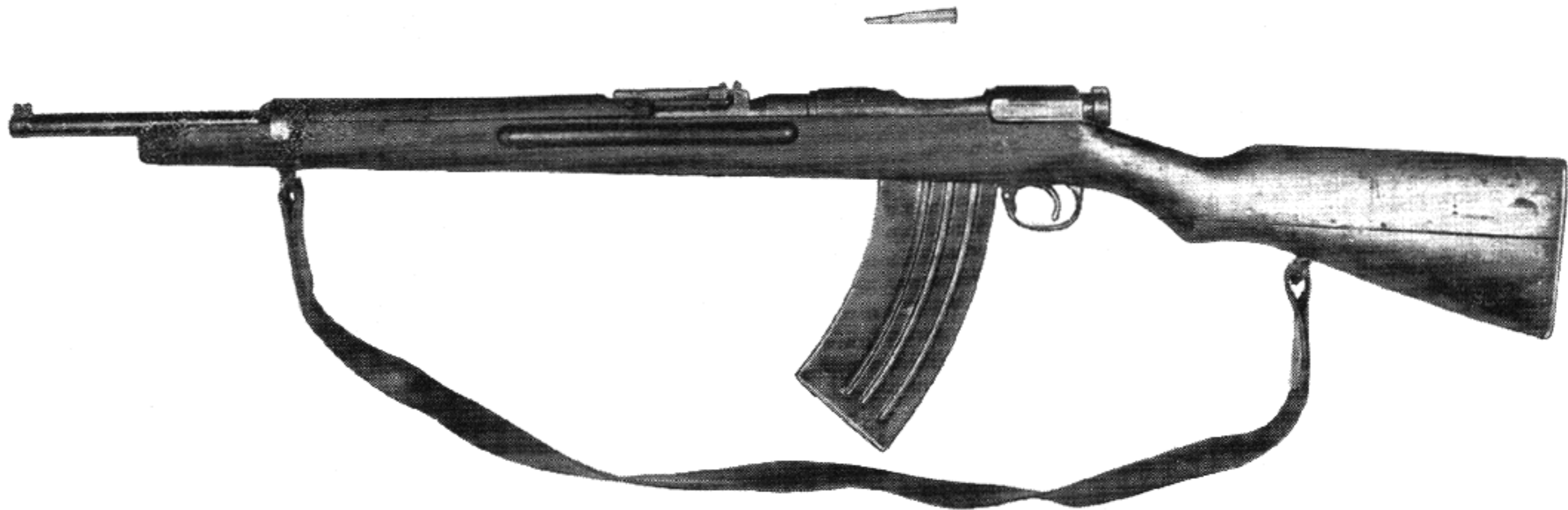
Japanese Type 38 (1905) stock cut down and with a LMG magazine.
