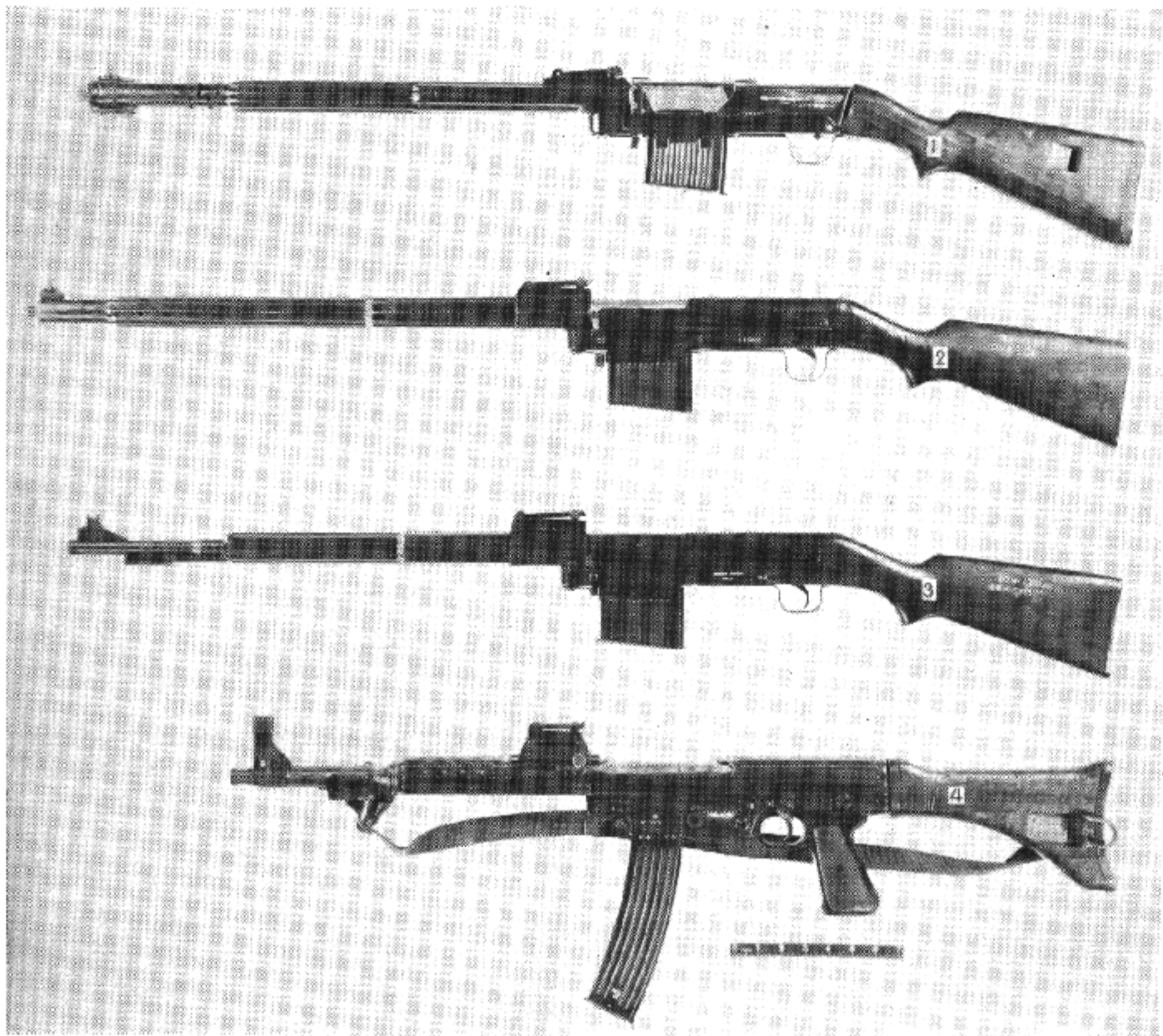
Top to Bottom: Walther G A115 No. 1, G A115 No. 2, G A115 No. 3, Semiautomatic Rifles; and Walther MKb-42 (W) Assault Rifle. The rifles appeared in prototype form and their gas system was used on the MKb-42 (W) Assault Rifle and in modified form is currently being used on the Czech Model 52 Rifle.
