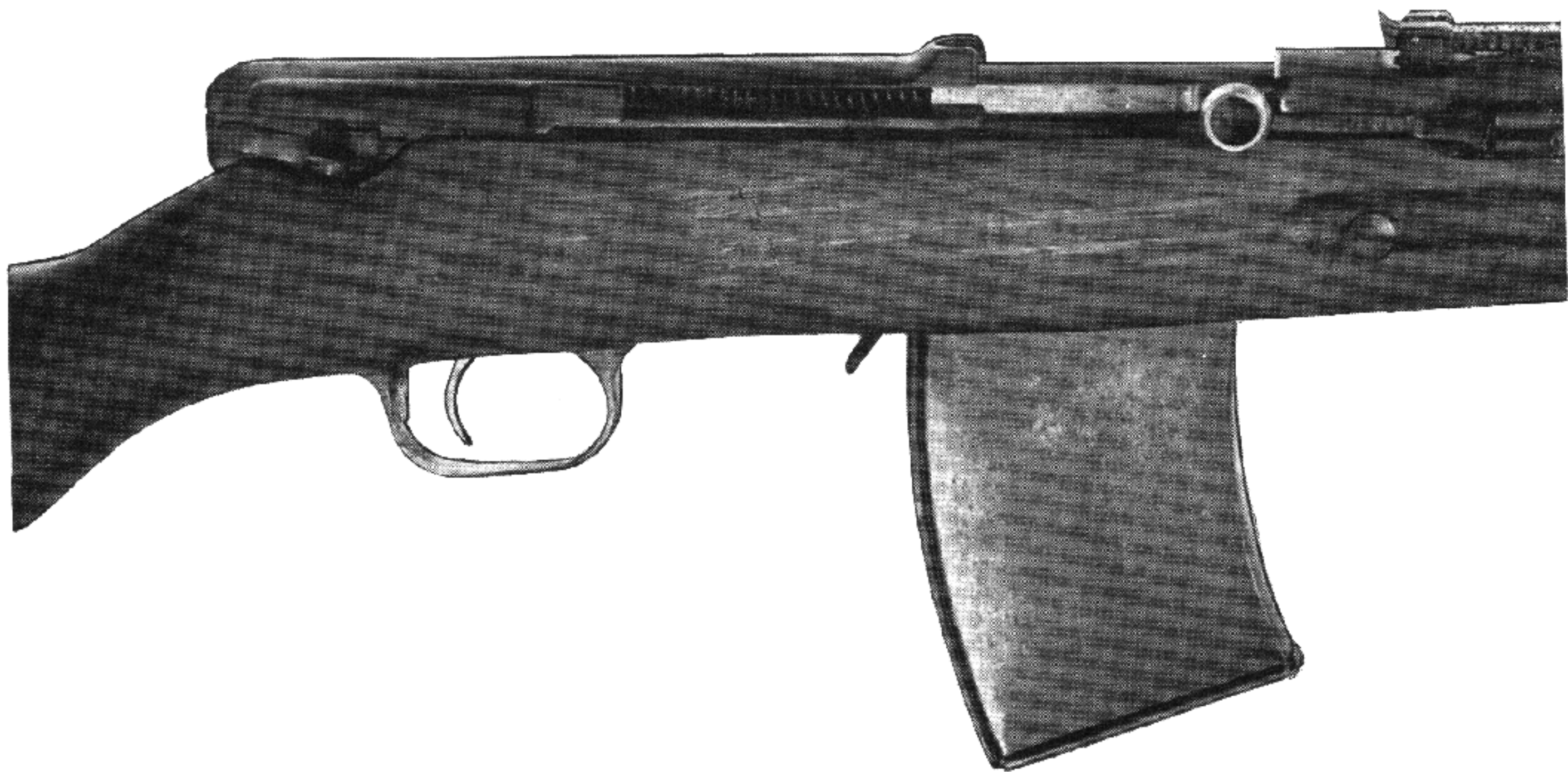
Russian Model 1936, showing details of breech construction and cocking handle. The exposed travel port permits dirt to enter the action very readily which results in unreliable performance. This design was not put into extensive production.
