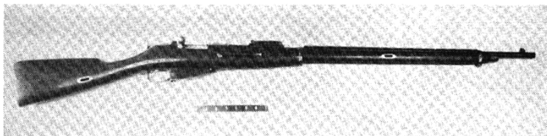
7.62mm M1891 Mosin Nagant Rifle of later manufacture. Note sling slots through stock and rounded sight leaf.
