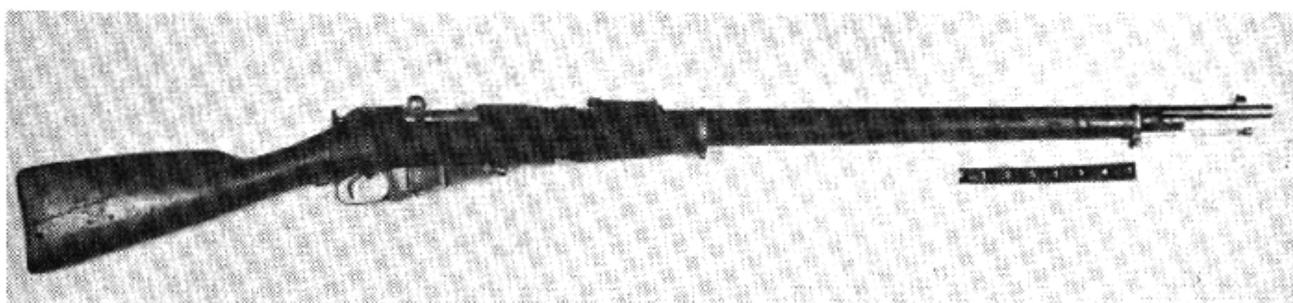
7.62mm M1891 Mosin Nagant Rifle of early manufacture. Note sling swivels and flat leaf rear sight.
