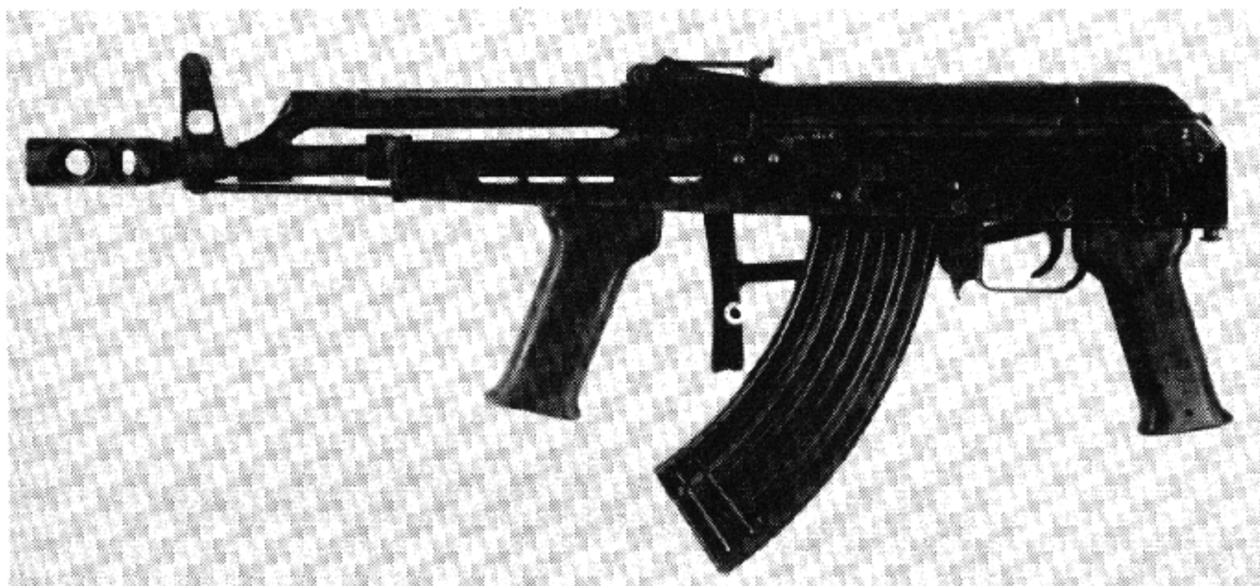
The AMD, Hungarian version of 7.62mm AKM with short barrel and muzzle brake.
