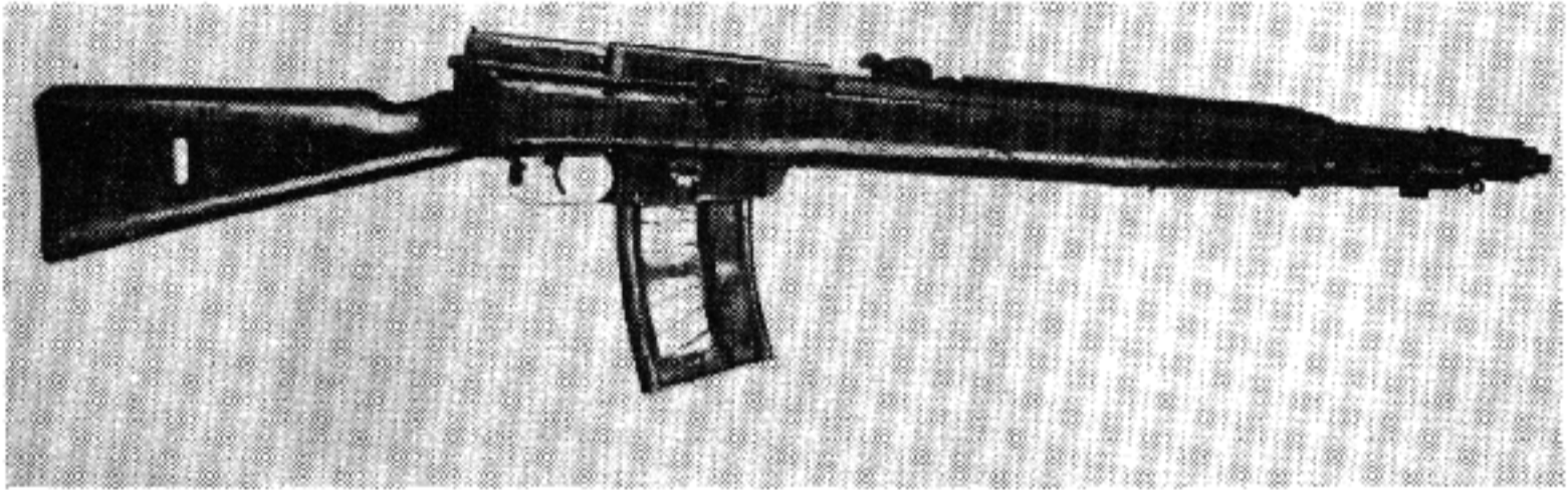
Breda 6.5mm Model G.P. 1935 Semiautomatic Rifle.
