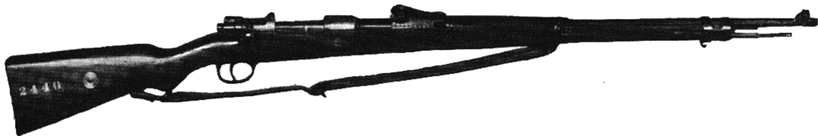
Peruvian Model 1907 (Mauser) caliber 7.65mm. Except for caliber this is practically identical with the German Gewehr 98. It was made in Germany. Later patterns based on the improved Kar. 98k are also used in Peru, most being Belgian F. N. manufacture.
