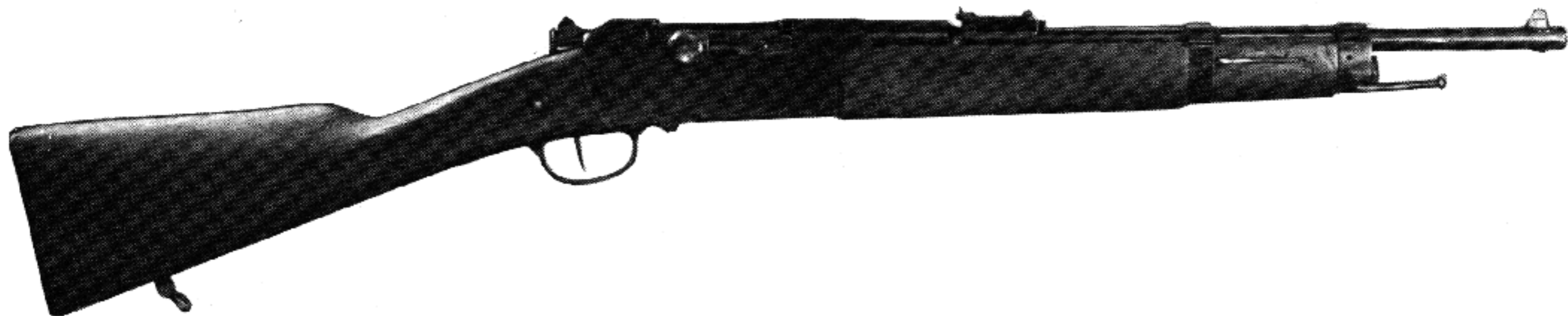
French Model 1886-RM-35 (1886 M93 R35). This is the old M. 1886 M93 altered in 1935 to a carbine form. The 8mm caliber was retained, as was the tubular magazine form. Magazine holds 3 cartridges.
