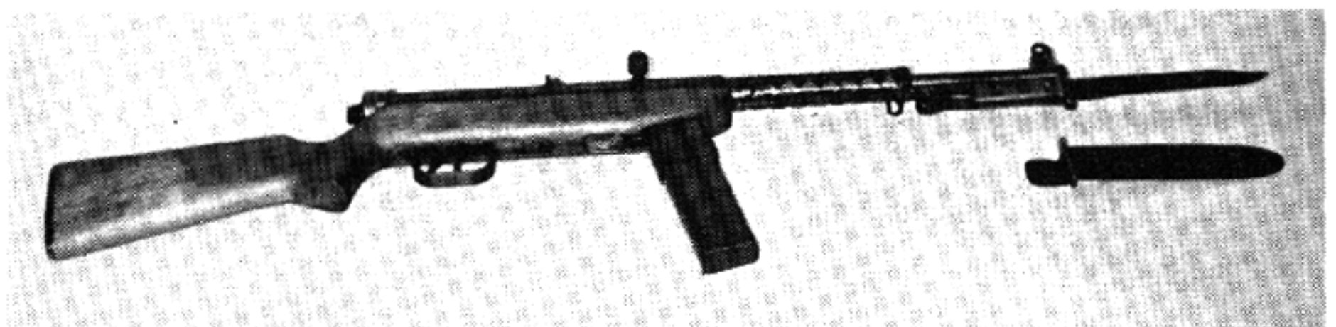
Dominican Cal. 30 M1962 Carbine. This weapon uses the 30 carbine cartridge and is made with a folding steel stock or with a wooden stock.
