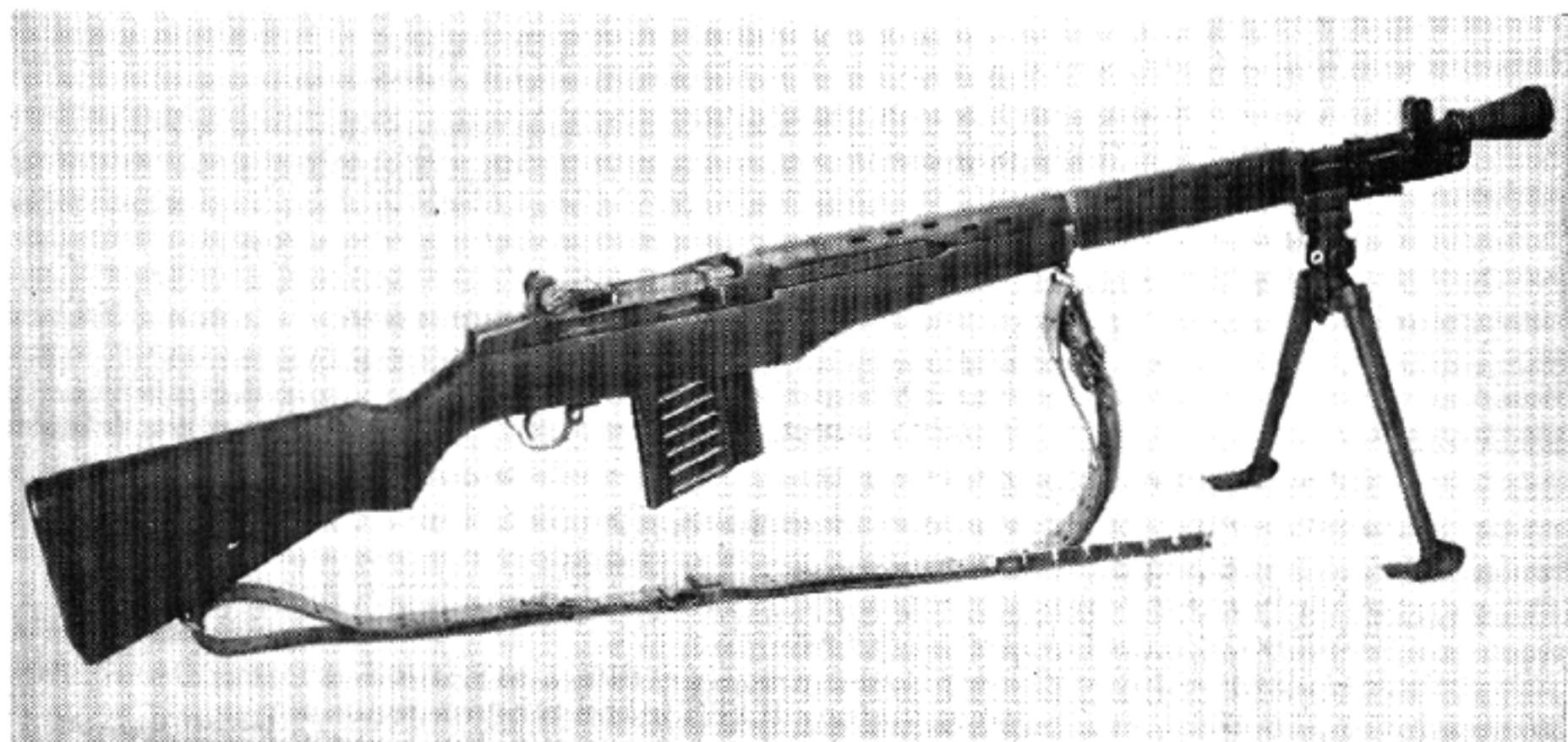
U. S. Rifle Caliber .30, T22. A selective fire prototype developed by Remington from the M1.
