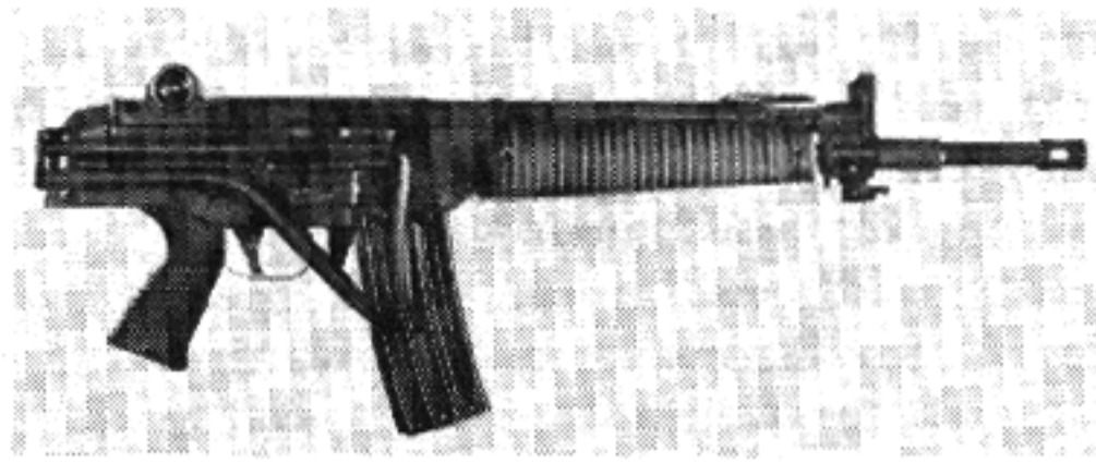
SIG .223 Model 530-1 Rifle with folding butt stock.
