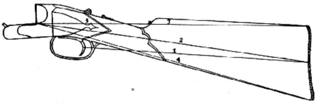
Measurements of stock for single trigger
