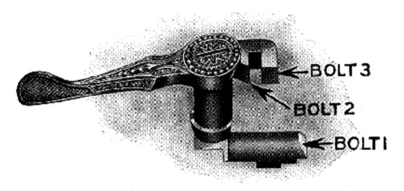
Ithaca bolting mechanism
