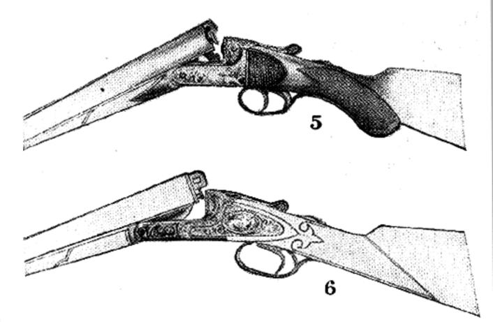
(5) Quintuple fastening, double bolts in lugs, extension rib with shoulder bearing, and through cross bolt, Purdey sideclips;
