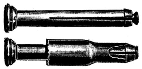
Extractor with section of broken shell
