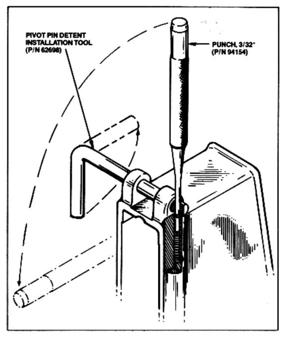
A. DETENT AND DETENT SPRING INSTALLATION.
