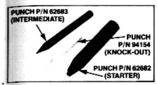
FIGURE A5. PUNCH SET FOR FRONT SIGHT TAPER PIN REMOVAL AND INSTALLATION (SEE FIG. 3-2E, PAGE 21)
