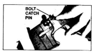
H. BOLT CATCH PIN REMOVED
