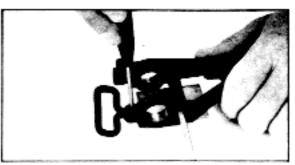
K. FRONT SWIVEL RIVET REMOVAL (1/4" PUNCH, P/N 94155)
