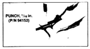
AE. FORWARD ASSIST PAWL ROLL PIN REMOVAL
