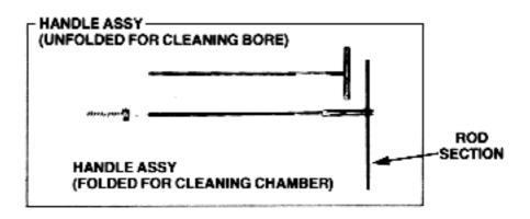
FIGURE A-1. BORE AND CHAMBER CLEANING TOOLS
