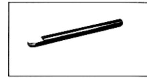
FIGURE A8. PUNCH SETTER (P/N 62692) (WINDAGE DRUM ROLLPIN)
