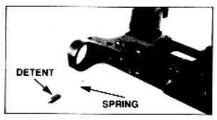
E. REMOVE/INSTALL DETENT AND SPRING.
