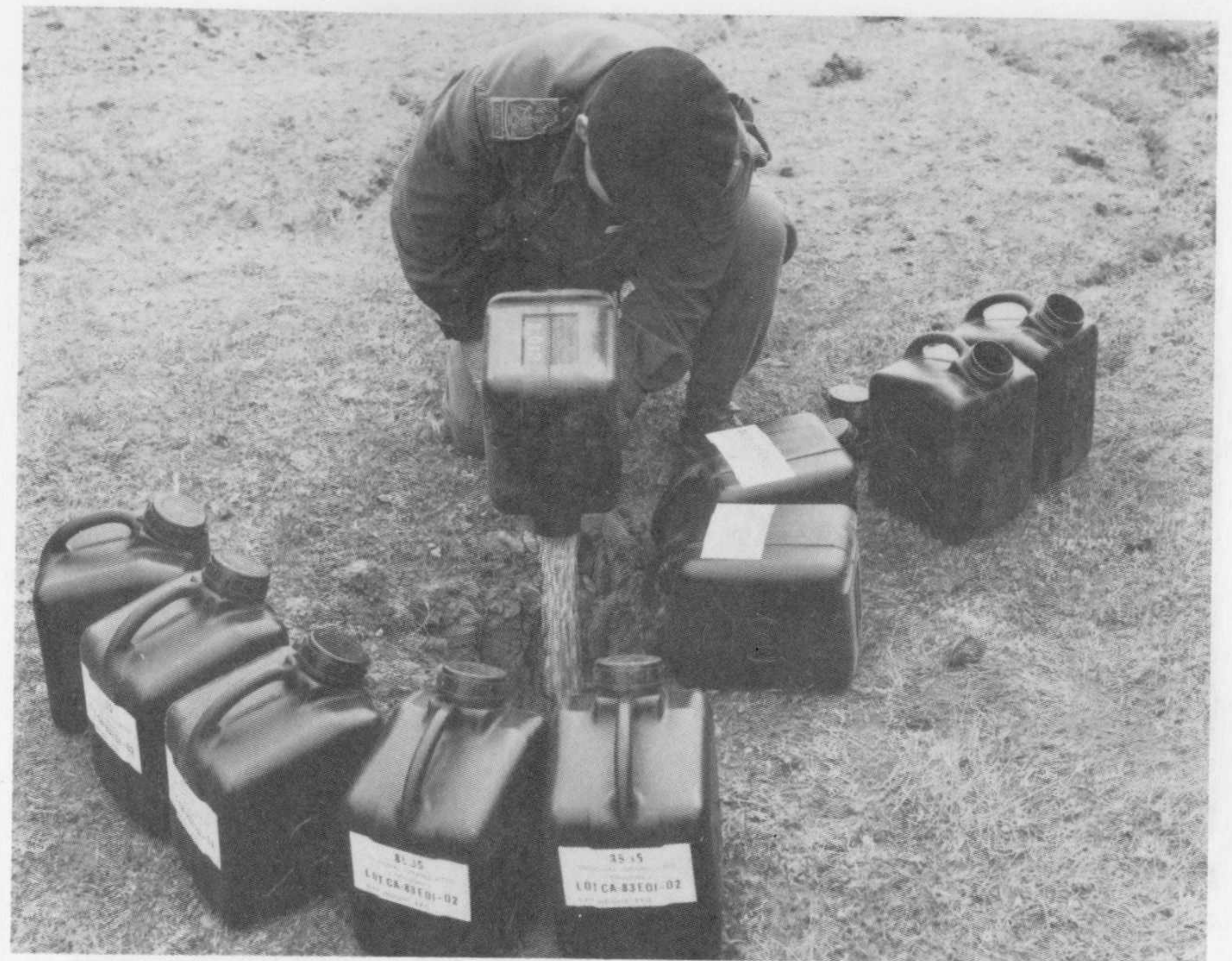
Figure 56. TRIGAN is poured from its original plastic containers into a shaped charge borehole (courtesy Defense Research Establishment Suffield)).
