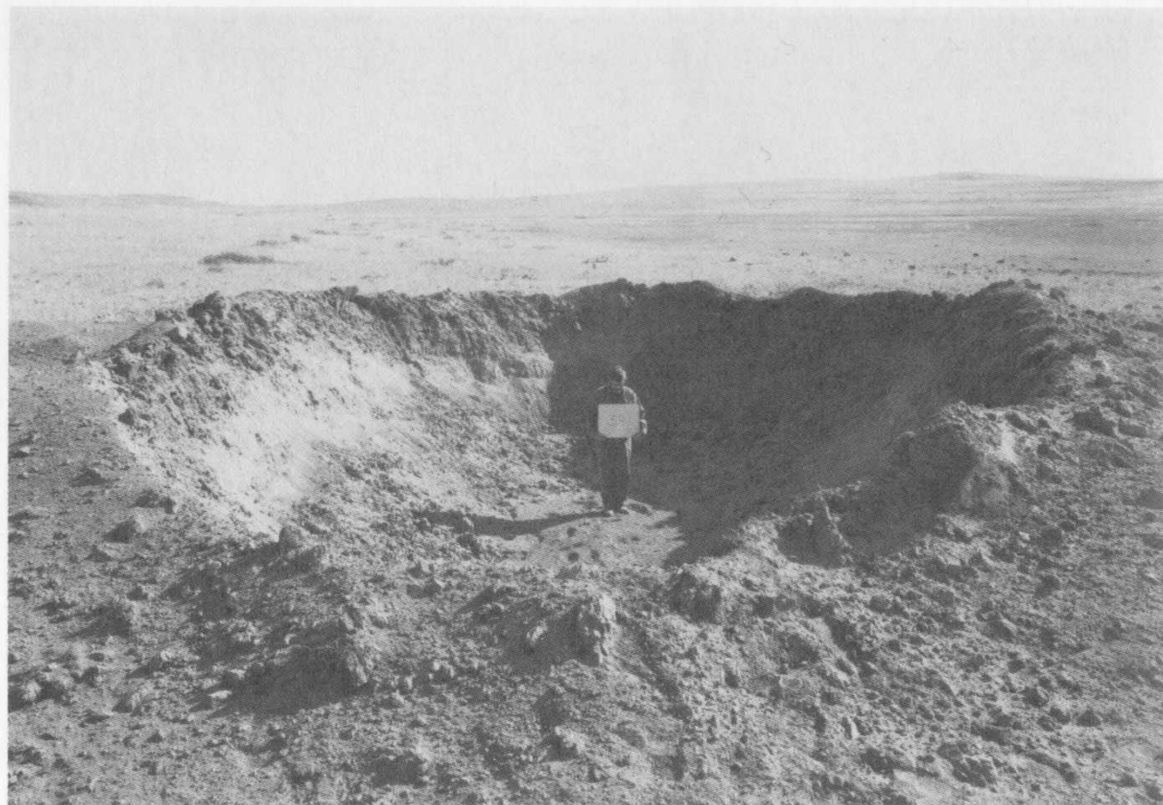
Figure 58. A typical countermobility obstacle produced by the detonation of TRIGAN charges (courtesy Defense Research Establishment Suffield).
