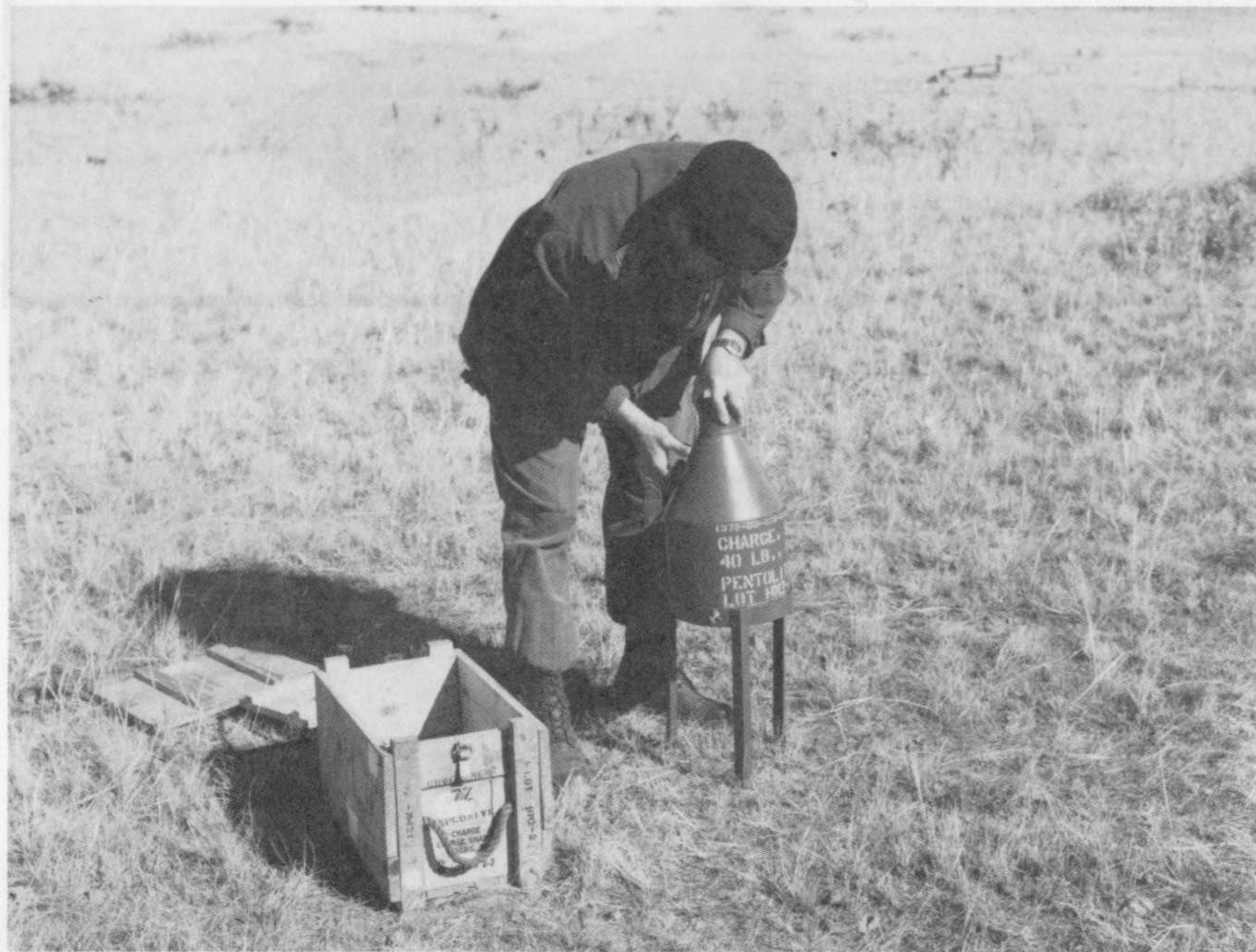
Figure 54. The setup of a shaped charge used for cratering (courtesy Defense Research Establishment Suffield).
