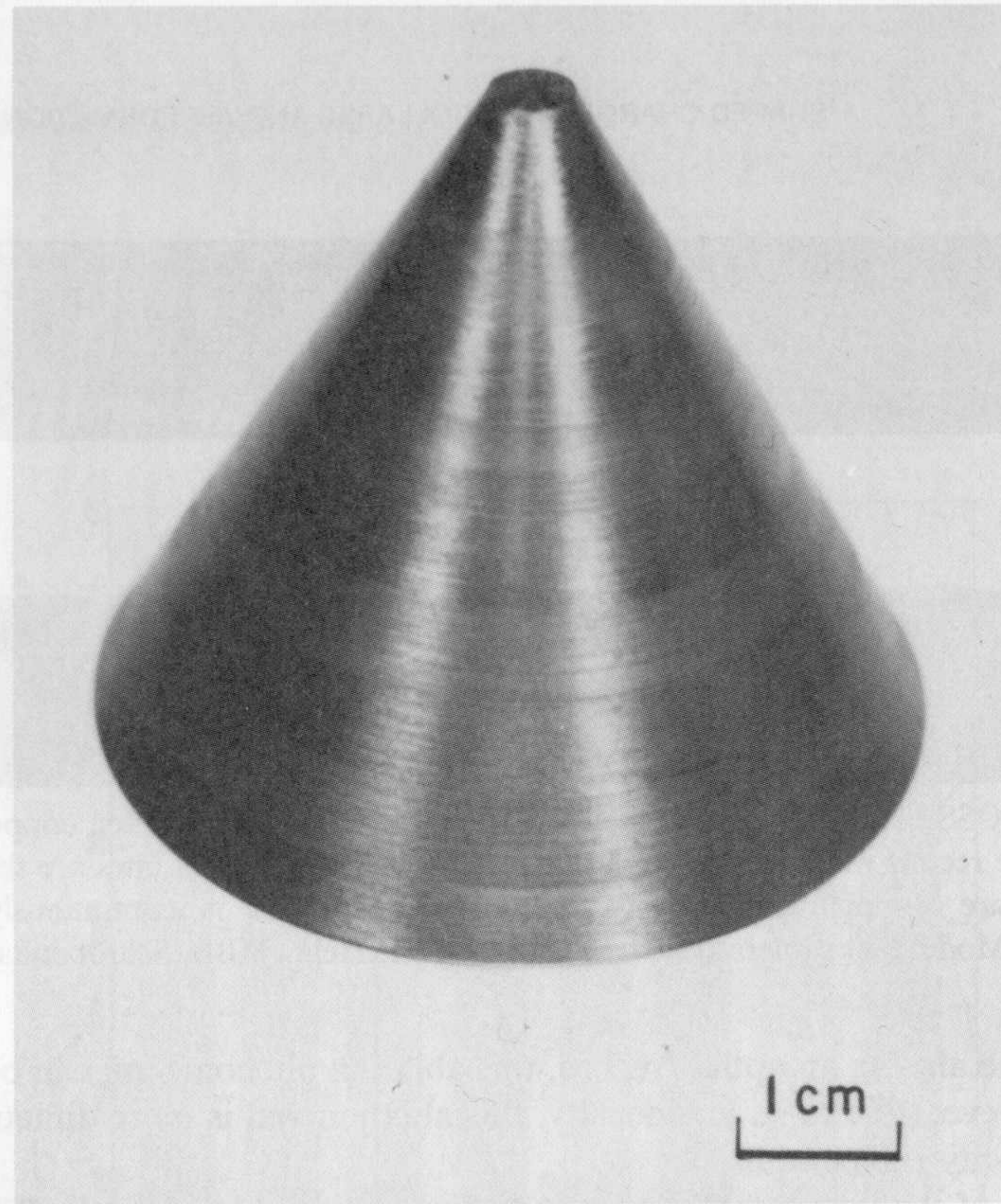
Figure 21. Finish machined, stratified, copper-nickel, conical shaped charge liner (Walters and Golaski 1987).
