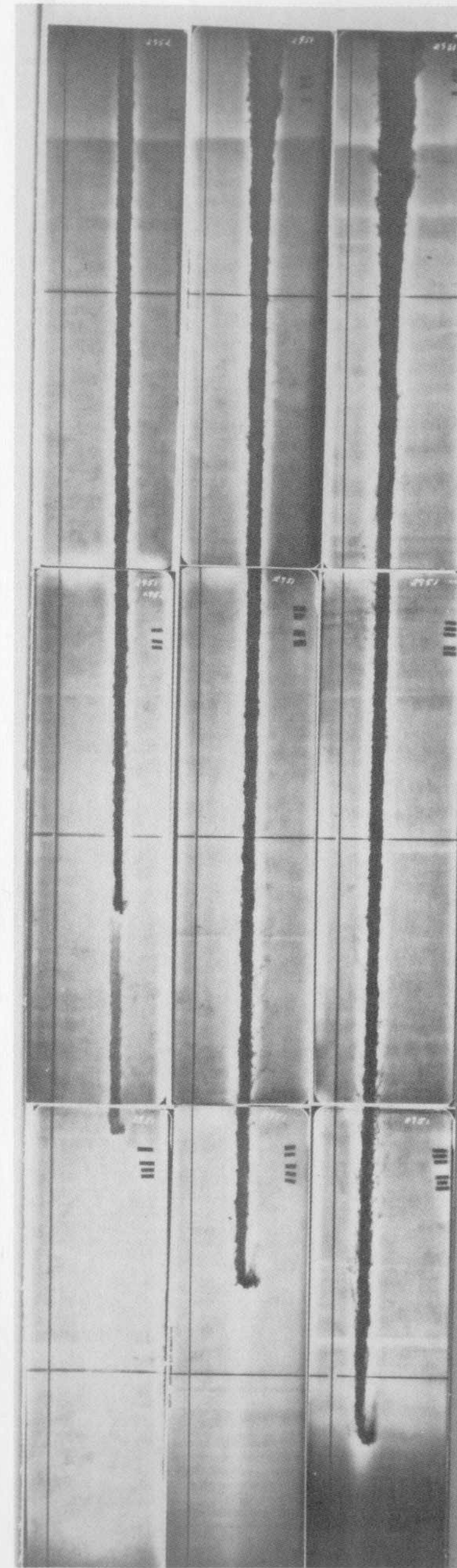
Figure 77. Free-flight flash radiograph of round 2951 of Table 1 (Walters et al. 1985).
