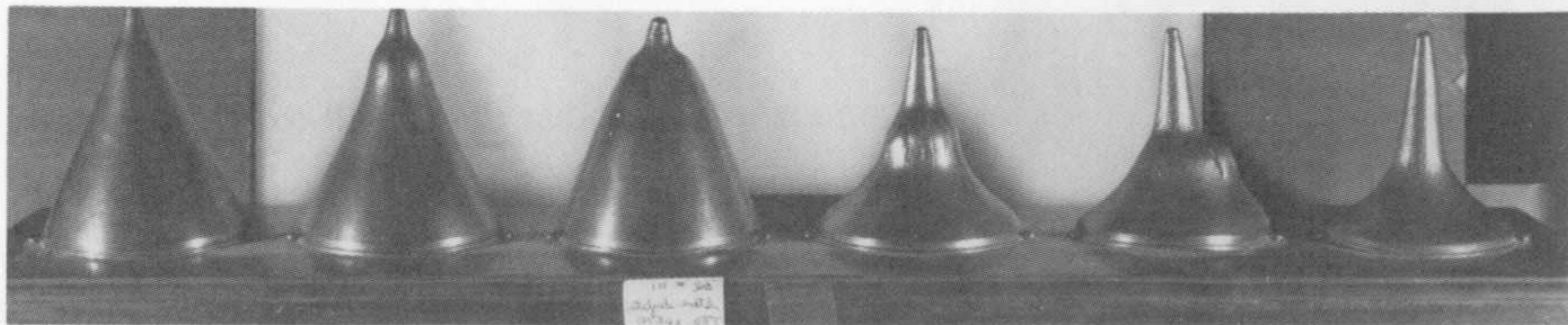
Figure 81. The partial collapse of a conical shaped charge liner, rear view (courtesy BRL).
