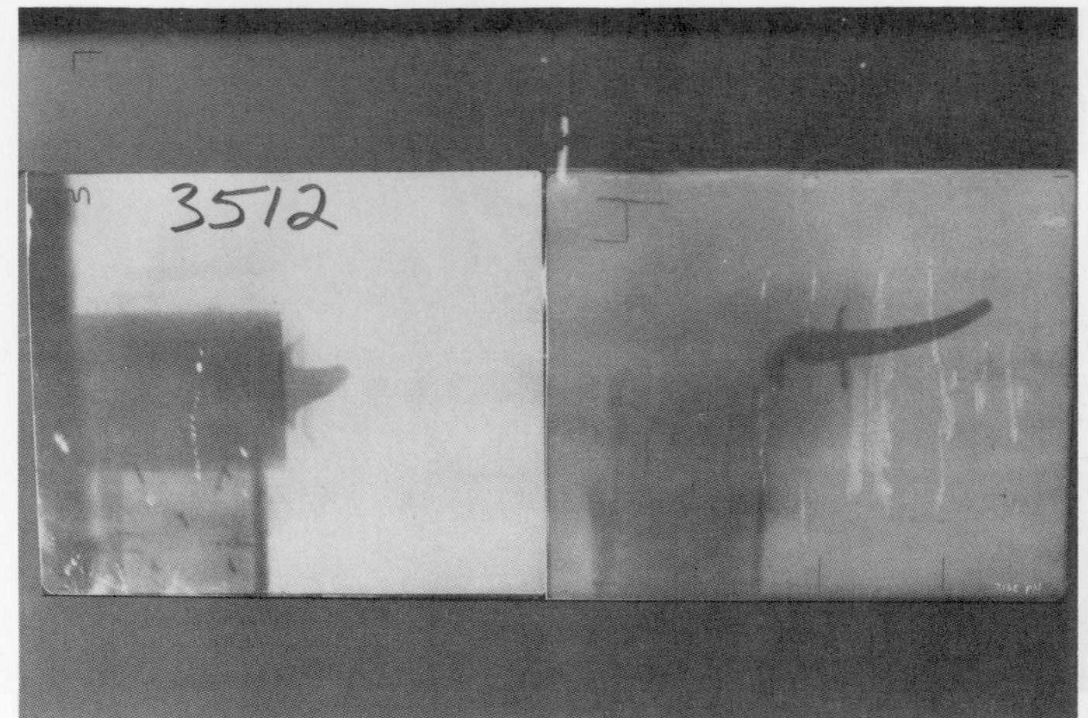
Figure 72. The jet formed from the collapse of a shaped charge with a hemispherical liner. The flash times were 39.4 and 54.4 \mu s. The offset angle was 17.35° (Walters 1986).
