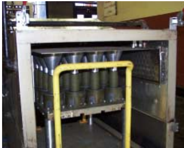
Figure 5 – Controlled Cooling Oven (front door removed)
