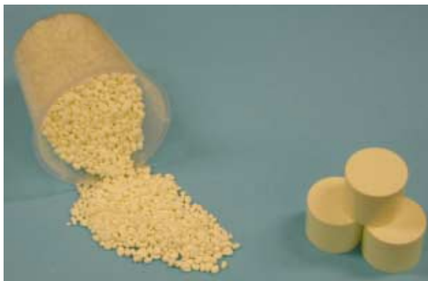
Figure 2. The DLE-P031 granules and pressed pellets.
