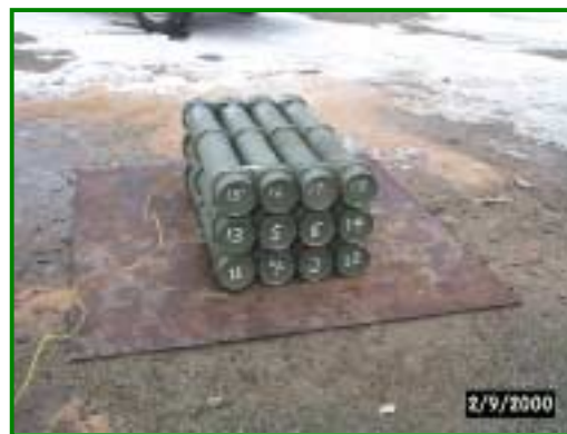
Figure 23 - Sympathetic Det. Test Setup
