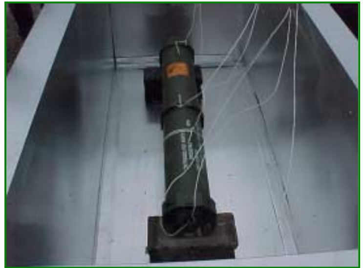
Figure 29 – M915 Projectile & Container in Oven
