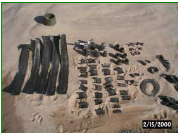
Donor round banana peeled projectile body and resulted in intact grenades and fragments
