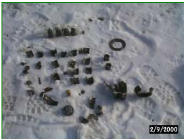
Recovered Components - only 4 intact grenades from one acceptor round
