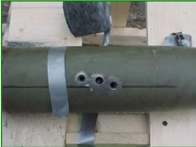
Figure 9 – PAX-2A (7.62mm Impact)
