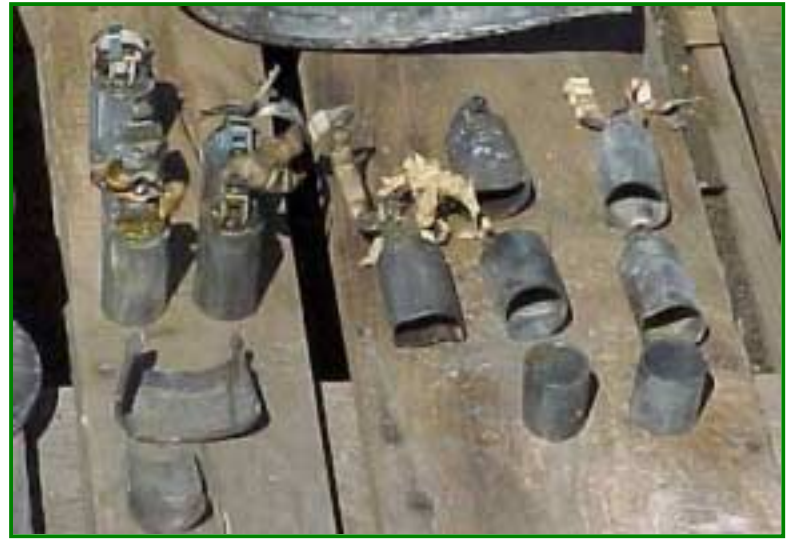
Figure 34 – PAX-2A Post Test Grenades
