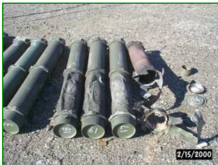
Acceptor rounds failed to detonate sympathetically
