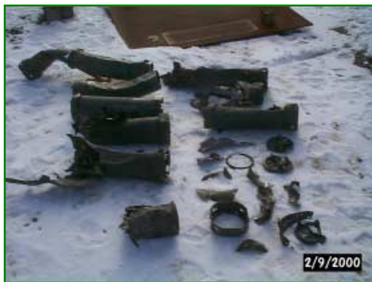
Recovered Containers – all acceptor rounds functioned high order!
