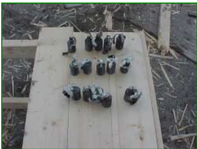
Figure 13- PAX-2A 0.50-Cal Impact
