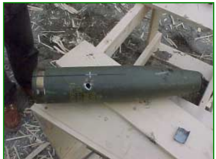
Figure 12- PAX-2A 0.50-Cal Impact
