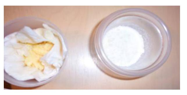
The products tested were "cold formed" white crystalline acetone peroxide and what was assumed to be yellow diphorone penta peroxide. A plastic sleeve was fitted around the top to hold in the *thermalite* "slow lent" fuse and then duct taped to insure adequate compression.
