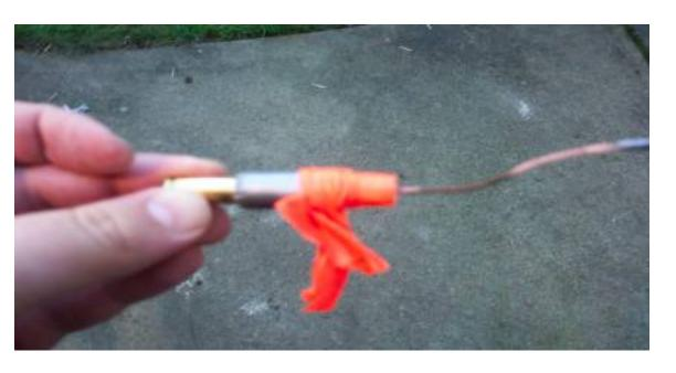
I placed the acetone peroxide-blasting cap into concrete block that was padded with low density Styrofoam. The blasting cap sat vertically with primer base on top of 2.5mm primed steel shelf plating.
