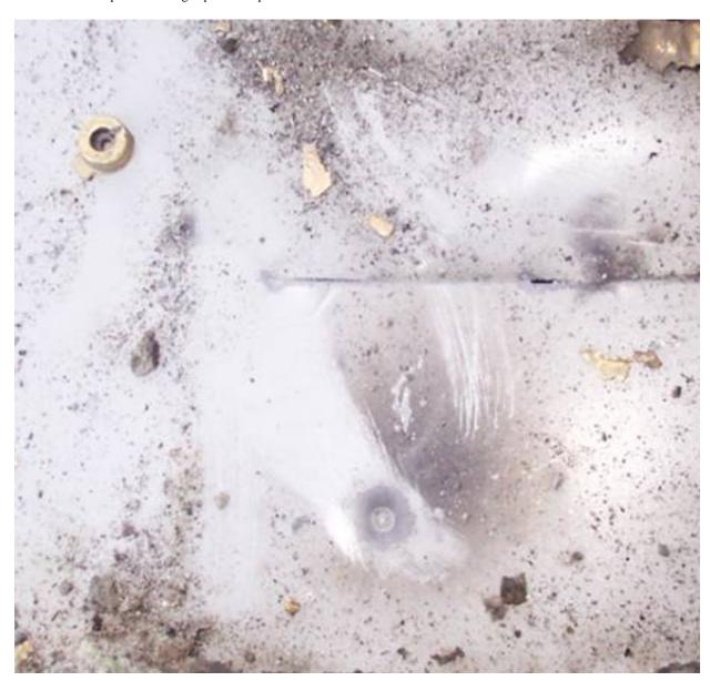
Next came the test of the diphorone penta peroxide-blasting cap. Again the blasting cap was ignited pyrotechnically. The explosion was intense and destroyed the brick housing. There was no smoke upon detonation. From the image below you can see the larger indentation clearly visible from the picture below.
