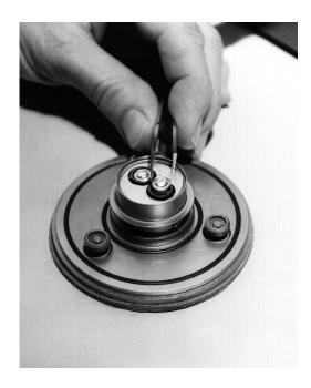
them to keep their temperatures exactly the same: *there is no heat flow between them.* The energy required to keep the temperatures the same is the quantity measured. If the sample melts, energy is supplied to the sample to keep its temperature the same as the reference. If the sample decomposes exothermically, energy is supplied to the reference to keep its temperature the same as the sample. The energy measured *is* the energy of the transition or reaction. The measurements are quantitative.
