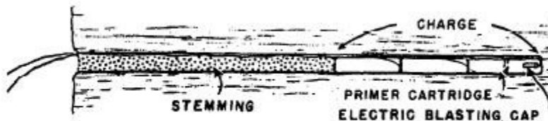
Fig 6 INDIRECT PRIMING OF PERMISSIBLE EXPLOSIVES
