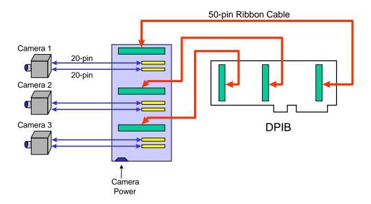
Figure 4.8 Break-out board example
