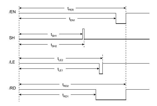
Figure 4.6 Pre-amplifier board timing diagram
