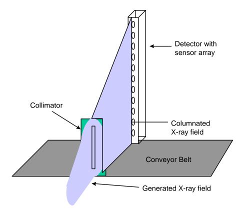
Figure 3.3 Collimated x-ray with sensor array
