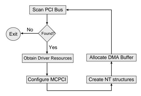
Figure 5.3 Flowchart of PCIDMA Initialization
