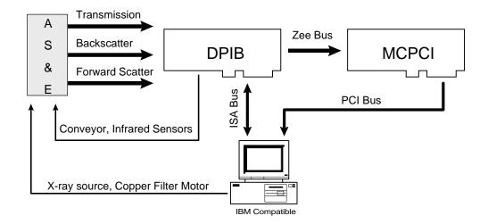
Figure 1.1 Prototype system overview
