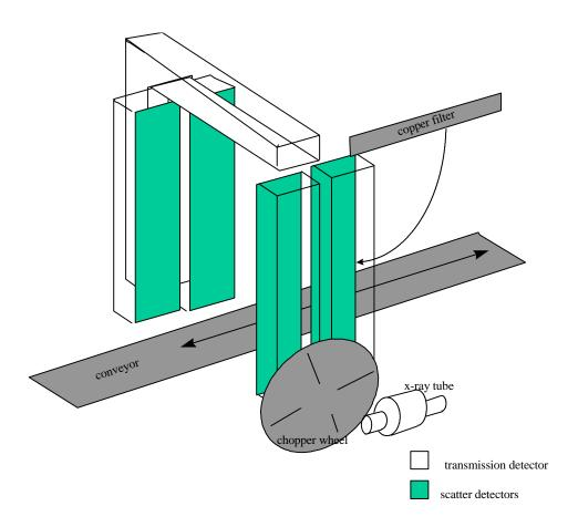
Figure 3.2 Modified source and detector placement
