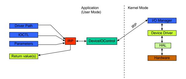
Figure 5.1 Hardware access through a device driver
