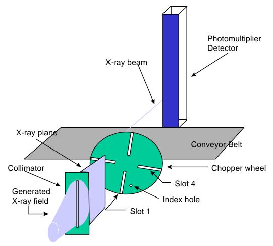
Figure 3.4 Flying-spot technology operation
