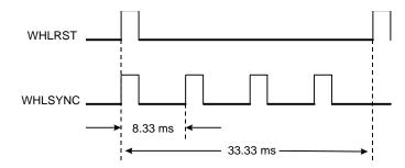
Figure 3.5 Chopper wheel synchronization pulses
