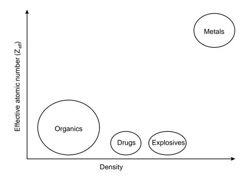
Figure 2.1 Z<sub>eff</sub> vs. Density of selected materials
