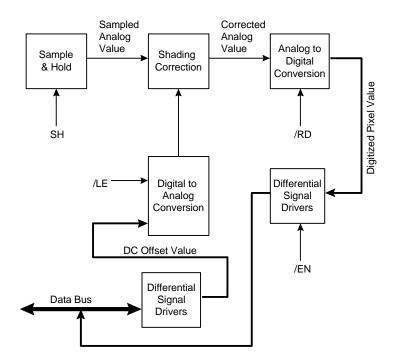
Figure 3.6 Digitizing pre-amplifier board block diagram
