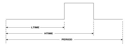
Figure 4.5 SIGGEN2 output waveform
