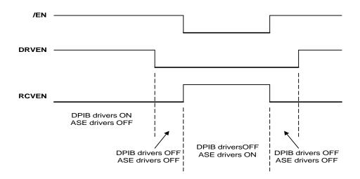
Figure 4.7 Differential bus arbitrator state machine
