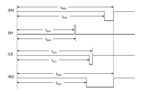
Figure 3.8 AS&E pre-amplifier board waveform
