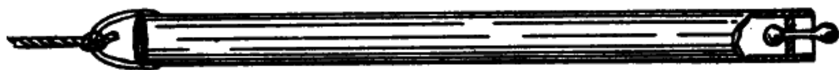
Fig. 79.—A pump for removing mud from deep well-drill holes. It is made of iron pipe with a valve in the bottom and a bail for attaching rope at top.
