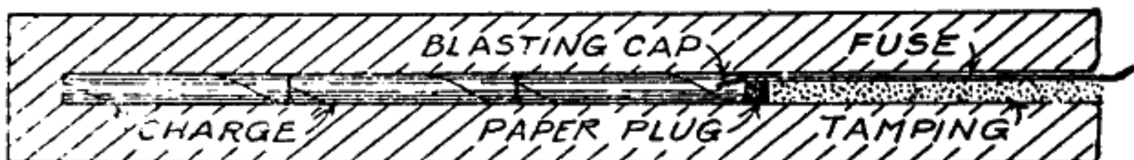
Fig. 86.—The use of a plug of paper, leaves or rags between the explosive charge and the tamping serves as a safety indicator of where to stop in removing tamping in case of misfires.
