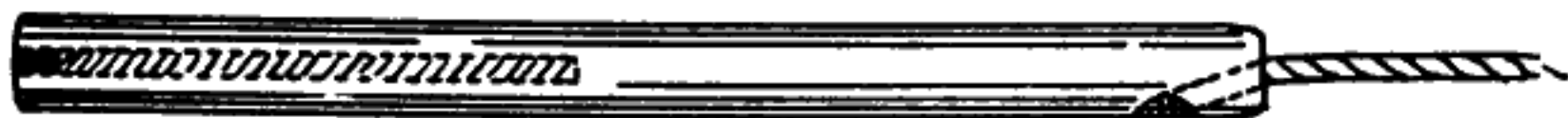
Fig. 78.—A tamping block for deep holes. The hole for the rope is bored diagonally from the center of the end and the rope knot countersunk into the side. For use under water, a hole is bored as shown by the dotted line and almost filled with babbitt or lead, then a wooden plug is driven in to close the hole. This makes the block sink in water.
