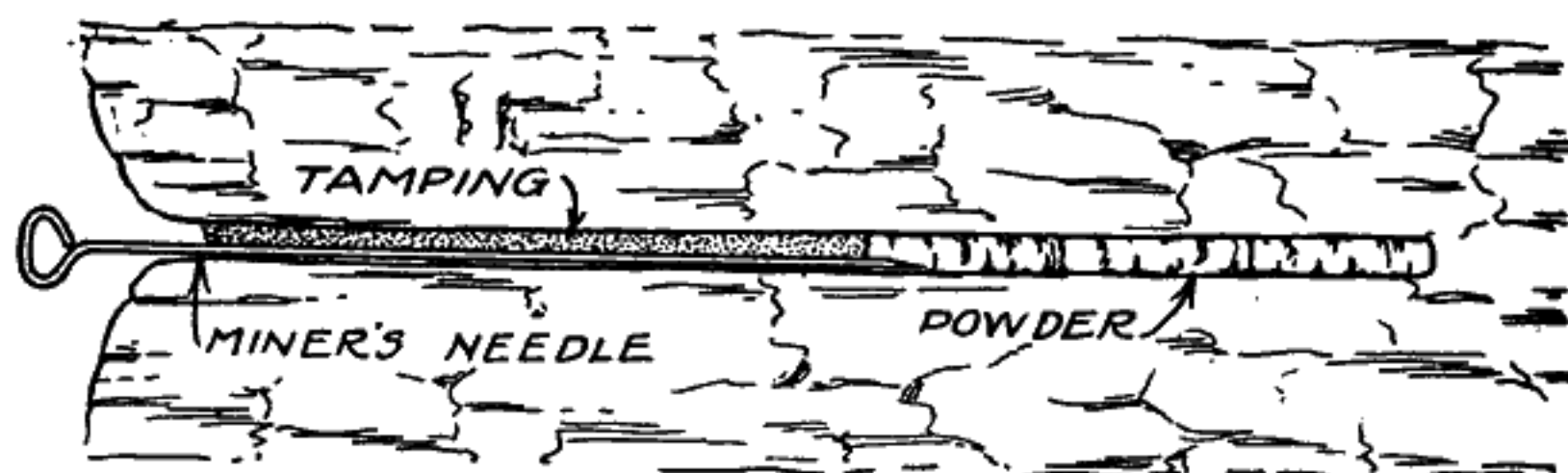
Fig. 7.—A bore hole loaded and tamped with miners' needle in place. The needle is withdrawn, and a miners' squib inserted in the opening thus made.
