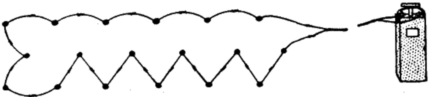
Fig. 147.—Plan of loading for a large electrically fired ditch blast using three lines of holes.
