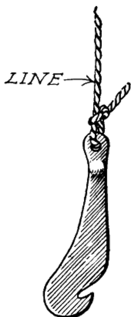
Fig. 139.—Special hook for bail of nitroglycerin container.
