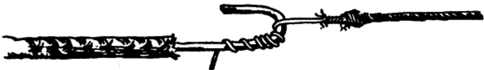
Fig. 45.—One method of attaching connecting wire or an Electric Blasting Cap wire to a leading wire.
