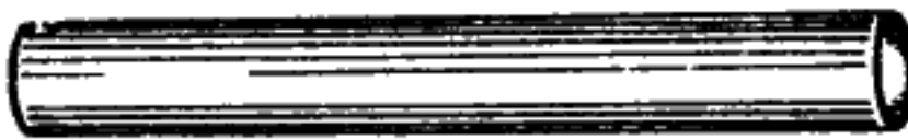
Fig. 12.—No. 6 Blasting Cap—exact size.
