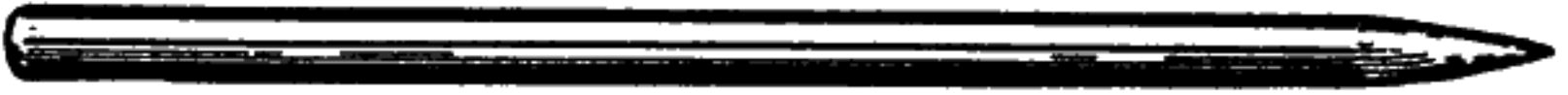
Fig. 68.—Soil punch or drill for making bore holes in clay, hardpan and rotten shale.
