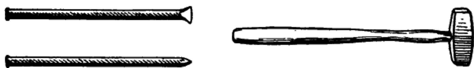
Fig. 71.—Hand drill and drilling hammer.
