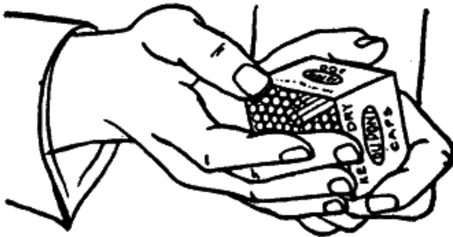
Fig. 31.—Take one cap from the box with the fingers.
