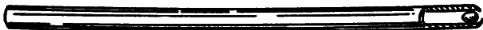
Fig. 81.—Another type of spoon, which is a modification of the pump for shallow bore holes.
