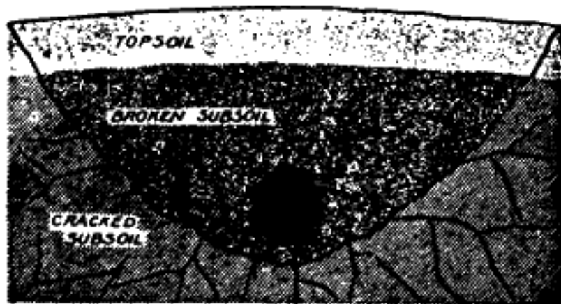
Fig. 128.—The blast thoroughly cracks the soil, but usually leaves a cavity or pothole at the bottom. This must be filled.
