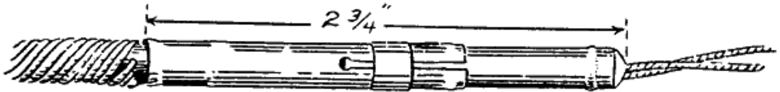
SPECIAL UNION FOR ATTACHING AN ELECTRIC BLASTING CAP TO CORDEAU
