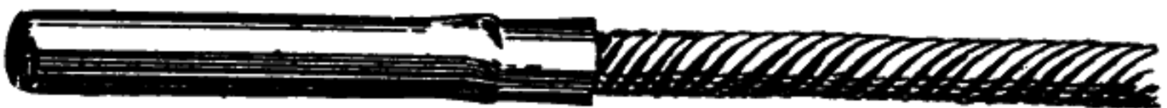
Fig. 16.—Cap crimped to fuse.
