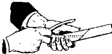
Side punching with handle of cutter-crimper.
