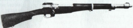
One of "Carbine" Williams' first homemade rifles, produced with milling machine or lathe from salvaged parts and an old piece of log. (Courtesy of J. David Truby.)
