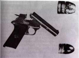
This single-shot "tip down" pistol was confiscated from a convict in transit between prisons. It showed real craftsmanship, having a floating firing pin, plus an unrifled barrel finished so well that it shot .38-caliber cartridges accurately. (Courtesy of Leslie L. Smith.)
