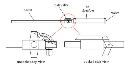
The above gun is charged from an air compressor through a tyre valve inserted in the end cap.
