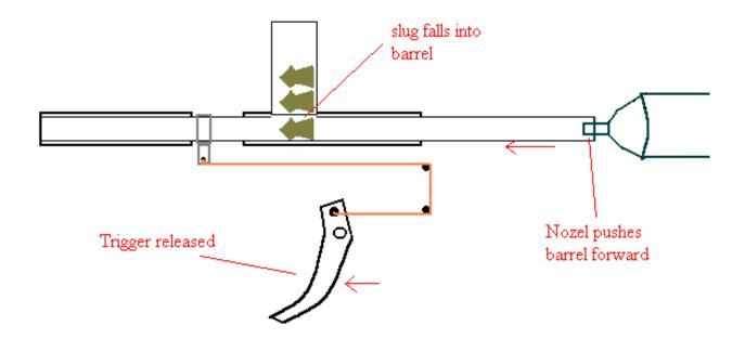
To avoid jamming pointed slugs should be used, another possibility that i hadnt thought of while constructing this weapon is the use of steel BB's, if these were used there would be no problem of jamming and it may be possible to hold the BB in the barrel by use of a magnet to stop it rolling out the end of the barrel.
