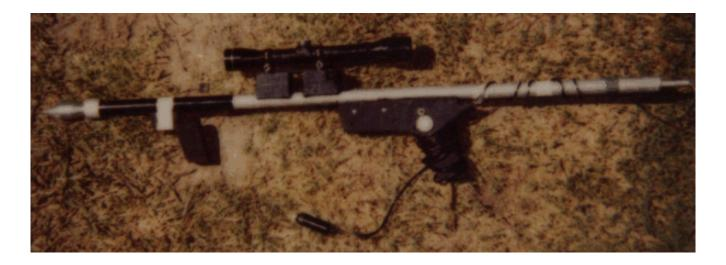
The launcher itself is simply an aluminium pipe, partially blocked at one end. A switch is built into the handle along with a 9 volt battery so that when the switch is pushed, the circuit is completed and the igniter ignites.
