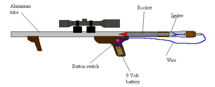
The rocket is powered by a bought estes D class engine, these can be found in most hobby shops however are rather expensive at around \$7-8 Australian per shot, trying to improvise a homemade rocket engine only increases the already high risk of an accident.
