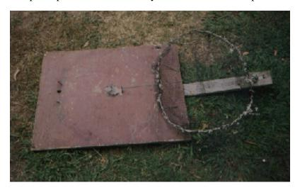
The trap above is nothing more than an oversized mouse trap, the wire is 8 gauge fencing wire that is bent into a circle (circle is vital). The back half of the circle is pinned down to a large flat board with the excess ends of wire bent in such a way as to put tension on the loop as its brought back. This is locked back by a strait piece of 8 gauge fencing wire, and the trigger is made in the shape of a standard mouse trap. Fine wire mesh is than tied around the loop to trap and hold the cat.
