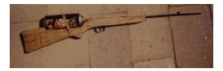
The idea is rather simple however rather hard to get to work. The gun is powered by an aerosole can that is fitted into a recession in the stock. There is an inner and an outer barrel in which the inner slides freely within the outer. I found these tubes at a hobby shop, the inner has to be a perfect fit for an air rifle slug and also inside the outer barrel.
