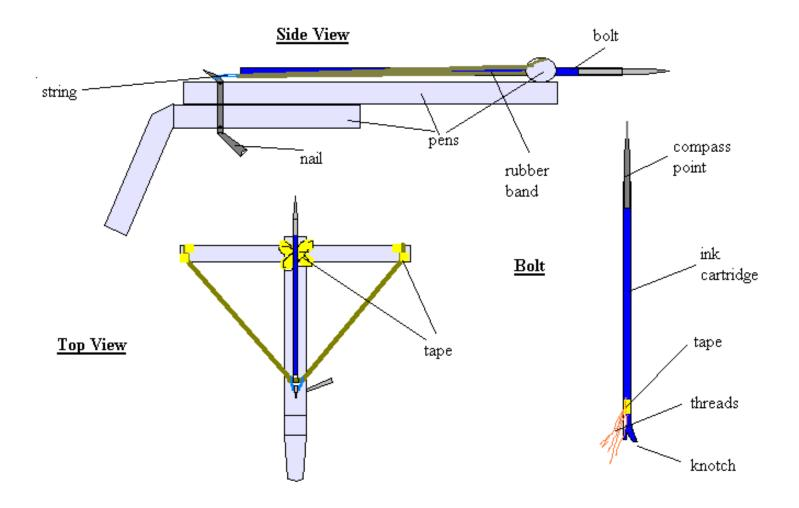
The pens are all taped together. The handle is heated over a heater until it can be bent down. To arm the weapon the rubber band is pulled back and the string loop is put around the nail, the knotch in the bolt is than pushed onto the rubber band inbetween the two knots from the string. To fire the nail is pulled back and the string slips off the top of the nail.
