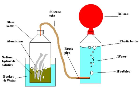
The bottle to the right contains the reaction between aluminium and sodium hydroxide (commonly sold as Caustic Soda in supermarkets \$3.50 for 500 grams), It is also possible to substatute sodium hydroxide for diluted hydrohloric acid. This reaction produces hydrogen, which runs through the tube, bubbles through the water and fills the balloon.
