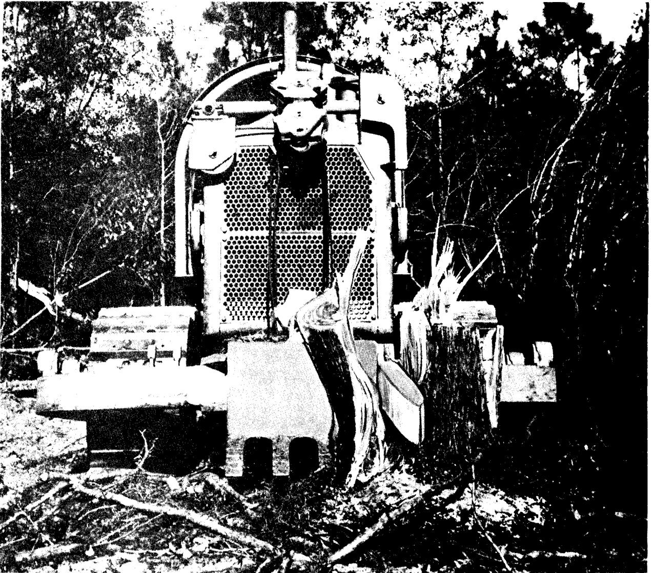
Figure 3-28. Detachable stumper with splitter.
