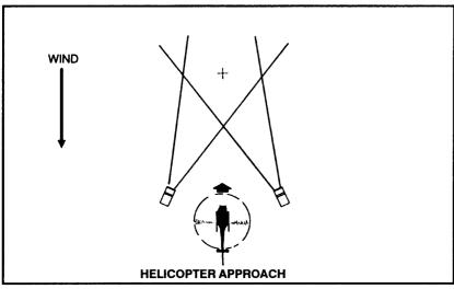
Figure 4-14. Emergency night lighting by vehicle headlights.
