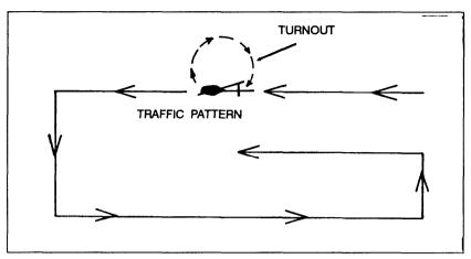
Figure 3-2. A 360-degree traffic pattern turnout.
