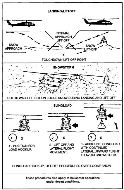
Figure 4-15. Lessening the effects of loose ground snow.
