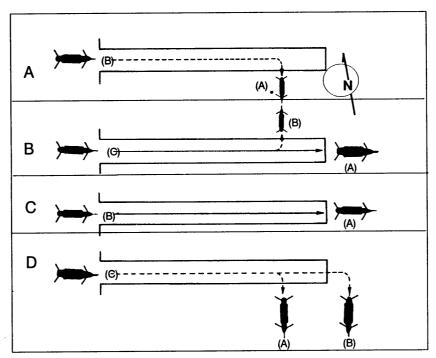
Figure 3-4. Minimum separation requirements.
