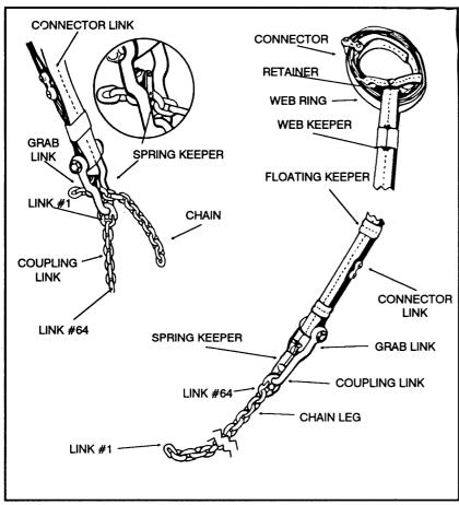
Figure 5-3. Parts of the multi-leg sling set.
