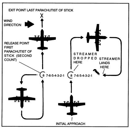
Figure 6-7. Wind streamer vector count.
