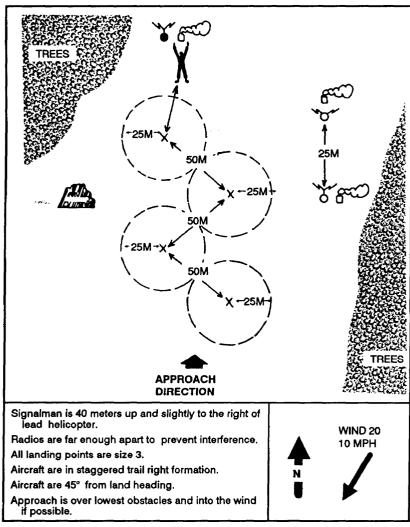
Figure 4-4. Helicopter day landing site, staggered trail-right formation.
