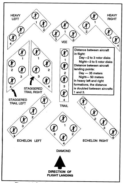
Figure 4-1. Standard flight and landing formations.
