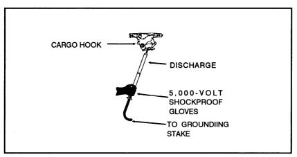
Figure 5-14. Grounding technique.
