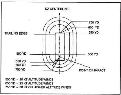
Figure 6-1. High tension lines criteria.
