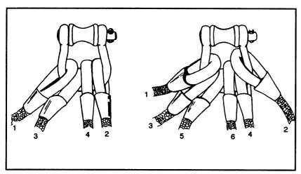
Figure 5-6. Sling leg numbering sequence.
