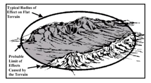
Figure 3-2. Effects of Mountains on Radiation and Blast
