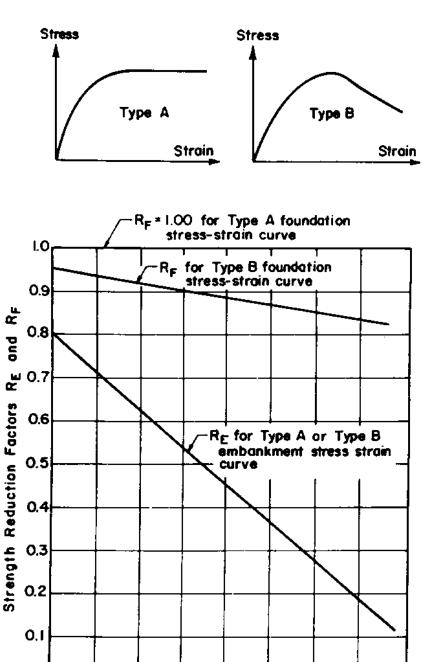
Figure 7-5. Peak strength correction factors for both embankment and foundation to prevent progressive failure in the foundation for embankments on soft clay foundations (Duncan and Buchignani 1975)
