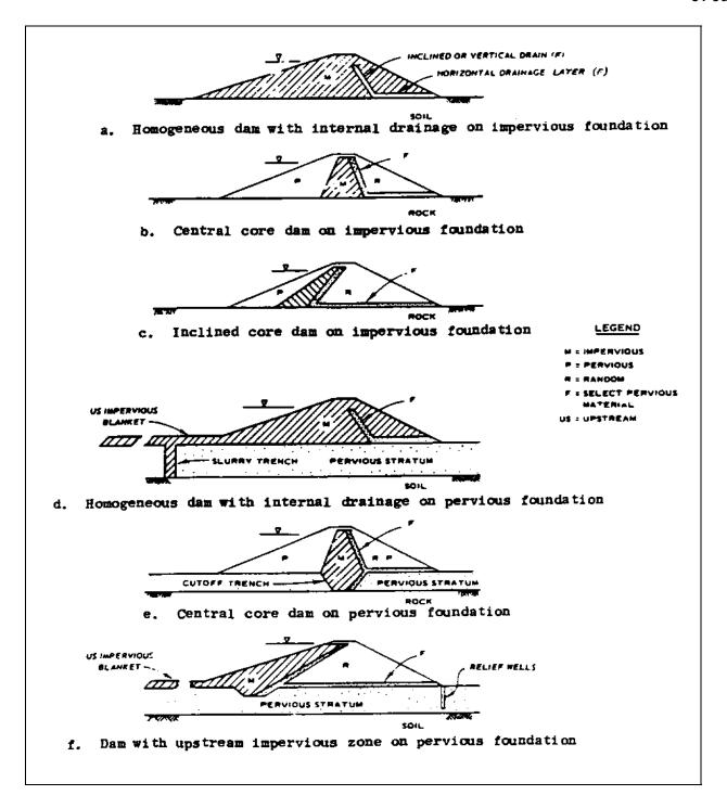
Figure 2-1. Types of earth dam sections
