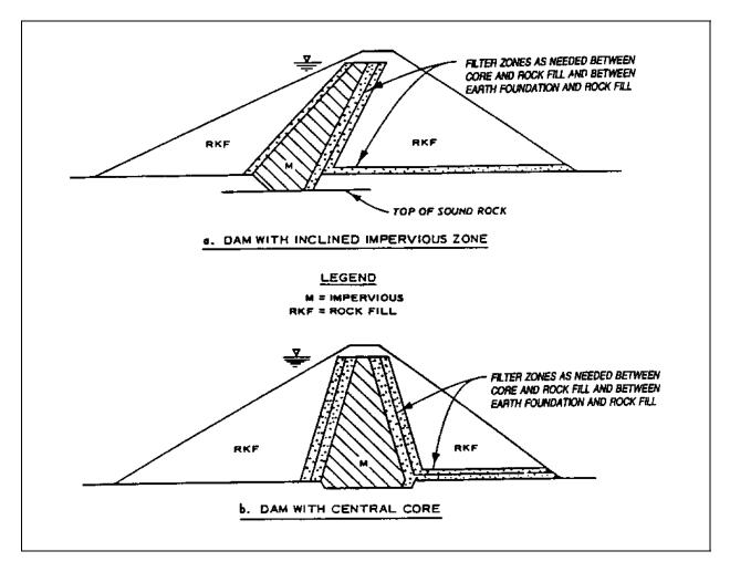
Figure 2-2. Two types of rock-fill dams
