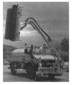
Fig. 2.14. Truck for tunnel washing<sup>46</sup>
