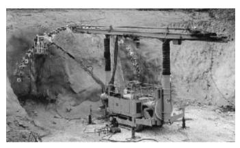
Fig. 5.25. Special forepoling rig, Rotex
