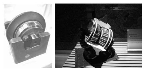
Fig. 4.55. Left: cutter, right: cutter bearing (Herrenknecht)
