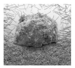
Fig. 5.7. Steel fibres and steel fibre reinforced shotcrete<sup>5</sup>
