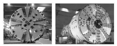
Fig. 4.27. Cutterheads with scrapers and discs
