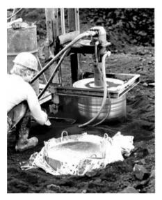
Fig. 3.3. Drilling of large core sample ( $\emptyset$  60 cm)
