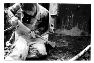
Fig. 3.4. Extraction of large sample by cutting
