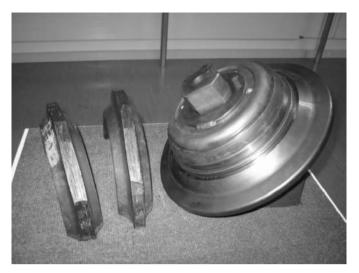
Fig. 4.65. Disc cutters from Lötschberg base tunnel. Left: Worn disc cutters
