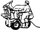
(c) A cavo loader: for development & stoping faces. Unloading into ore/waste passes
