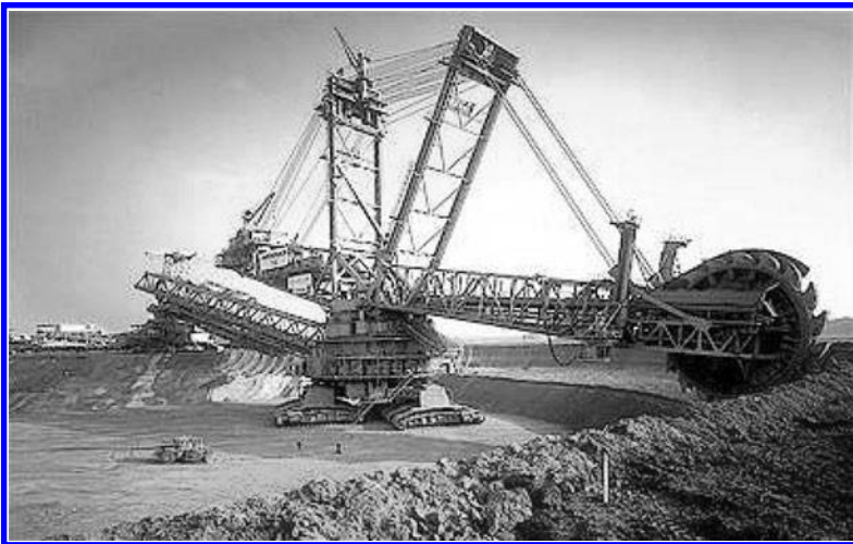
(b) Bucket wheel excavator – the largest mining equipment on earth. This technical giant is custom designed and built for the specific operating conditions and the production rates. Currently attained production rates are up to 240,000 m 3 (bank) per day, digging heights of as much as 100 m and service weights of 13,500 tons. (Courtesy: Krupp, 2000)
