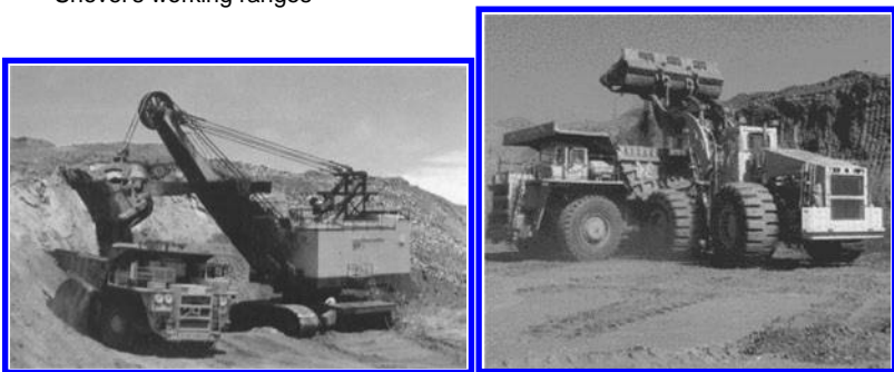
P&H 1900 electric shovels of 8.25 m 3 bucket loading Wabco off highway 120 tons truck.
