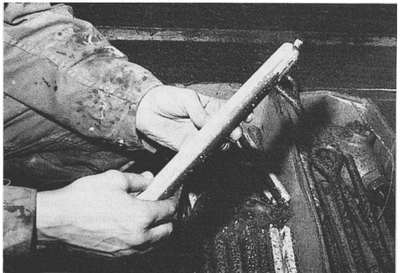
Figure 12.4: Typical resin cartridge for use in anchoring and grouting rockbolts.
