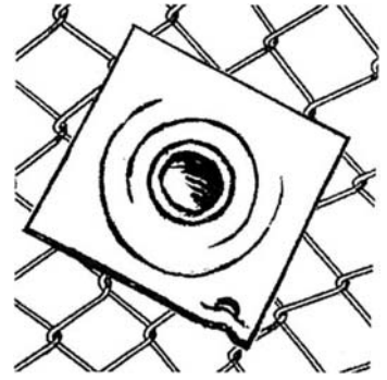
Wire mesh should be firmly attached to the rock by washers or face plates on the rockbolts or dowels.
