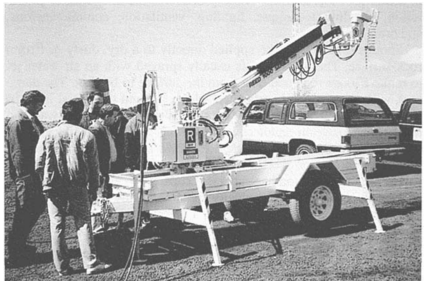
Figure 15.7: Compact trailer-mounted robot unit for remote controlled shotcrete application.
