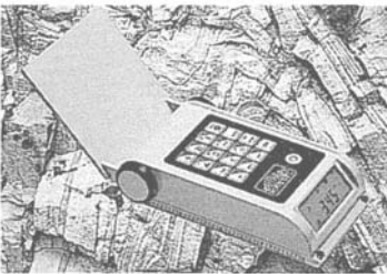
Tectronic 4000 compass for electronic measurement and storage of structural data. Manufactured by F.W. Breithaupt & Sohn, Kassel, Germany.
