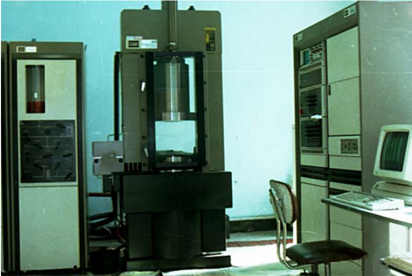
Fig. 4.9. Servo-controlled triaxial compressive test apparatus of MTS Systems in China University of Mining and Technology.
