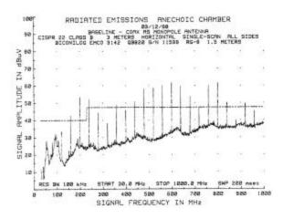
Figure 5. Baseline measurement of radiated emissions
