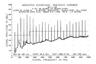
Figure 6. 5 mil trace with no RF return path
