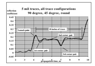
Figure 3. Impedance discontinuities Various corner configurations plotted together
