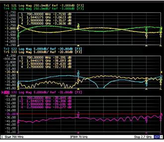
Figure 6. Hybrid coupler's typical characteristics for coupling (top), return loss (center) and isolation (bottom).
