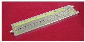
Figure 3. Ultrawideband 70 MHz to 2700 MHz Wilkinson divider/combiner using 17 sections with an air dielectric for minimum loss.
