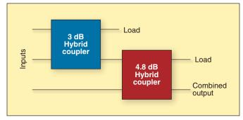
Figure 8. Schematic of a 3:1 hybrid combiner with 4.8 dB loss in each signal path.
