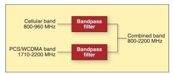
Figure 1. A typical two-input diplexer filter system.
