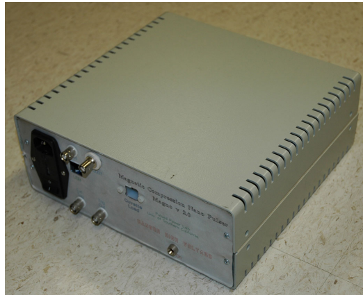
Figure 5.5 (a) Circuit diagram of Magna-II pulse generator. (b) Photo of Magna-II pulse generator.
